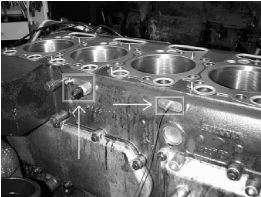
Figure 2.5 The picture shows a part of the warm side on a Scania DC12-01. The cylinder heads are removed and three sensor locations on the warm side can be seen. A Brüel & Kjær 4393 and a Lamerholm VP50/1 can be seen in the left marking and in the right a Brüel & Kjær 4393 with a connecting cable.
