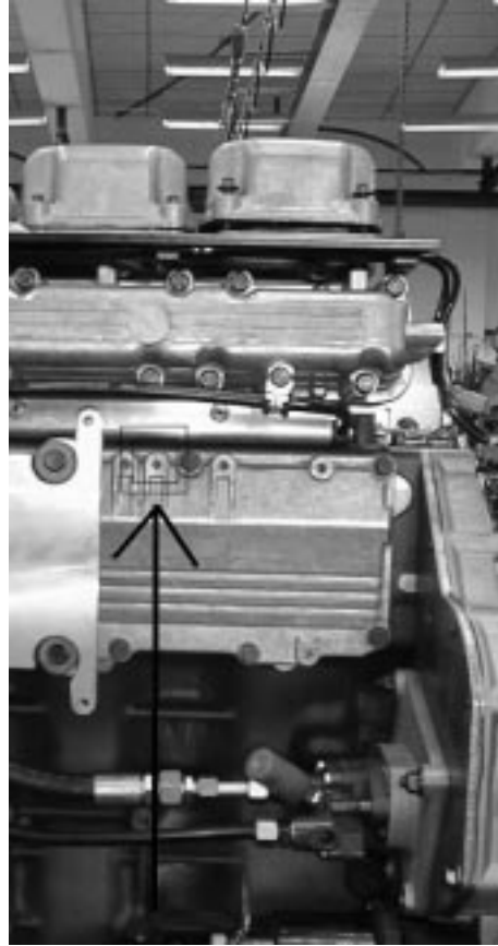
Figure 2.6 The picture shows a part of the cold side on a Scania DC12-01. The sensor location named B is marked.
