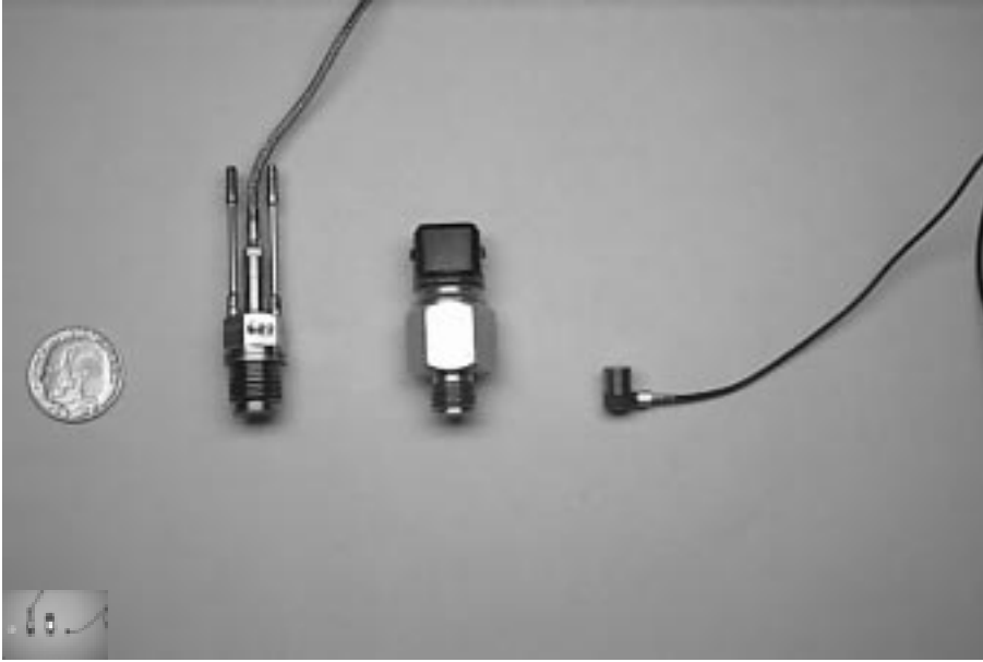
Figure 2.4 From the left: coin, Kistler 7061, Lamerholm VP50/1 and Brüel & Kjær 4393.
