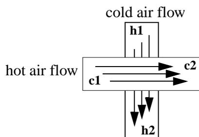
FIGURE 12. Cross sectional heat exchanger
