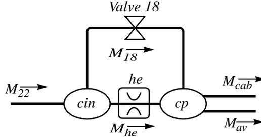
FIGURE 15. Model of cooling pack
