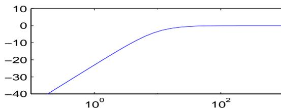
FIGURE 5. Model error transfer function,  $\Delta G(s)$ .
