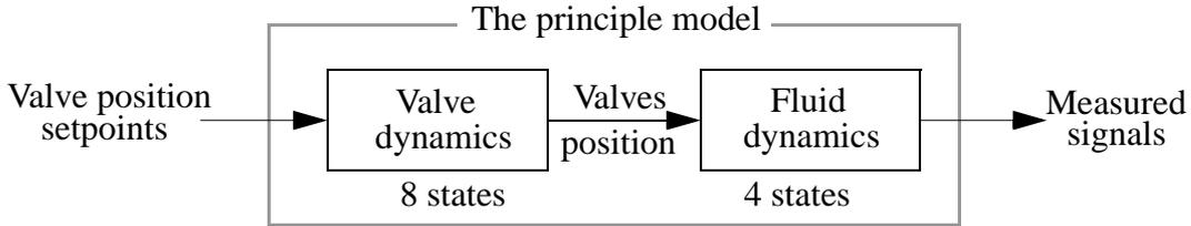
FIGURE 14. Principle model on state space form
