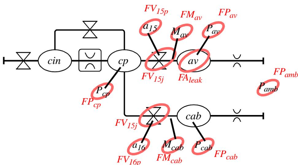
FIGURE 17. Localization of possible faults visualized in the principle model
