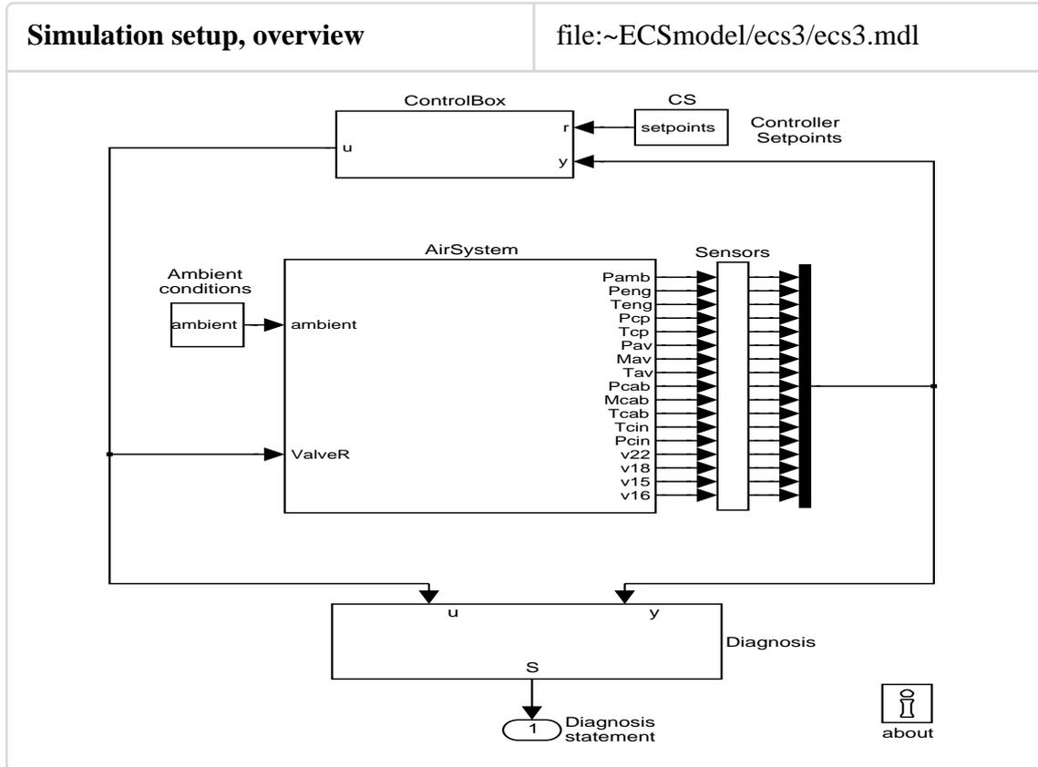
In order to shorten the evaluation time of the test quantities the model was divided in two parts. The first simulates the environmental process and the second runs the diagnosis system on the output from the first part.
