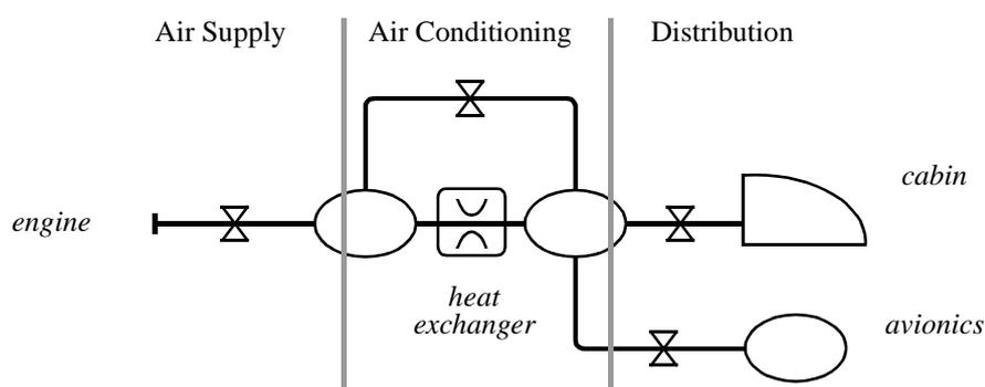
FIGURE 11. Principle model with main features
