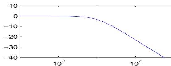
FIGURE 4. Valve, low order model transfer function,  $G(s)$ .
