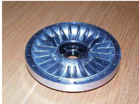
Figure 2.2: Photo of a hydraulic coupling half.
