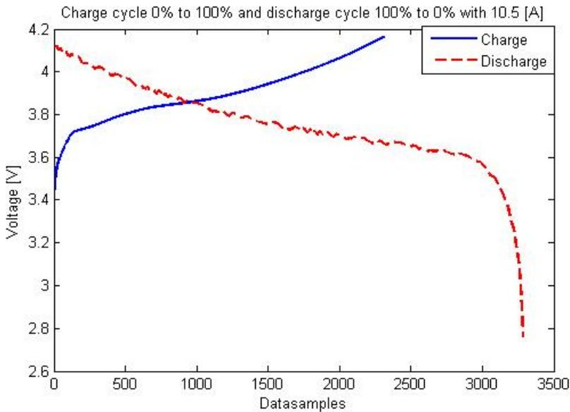
**Figure 2.3:** Charge and discharge cycle of one cell battery with current 10.5 [A].
