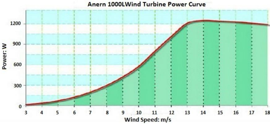
**Figure 2.2:** The power curve of Anern 1000L Wind Turbine.
