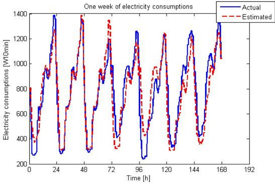
**Figure 3.6:** One week of electricity consumptions, estimated and actual data.
