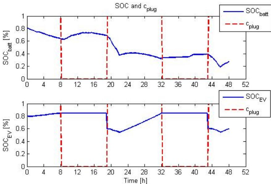
**Figure 5.6:** The state of charge of the EV during two days.
