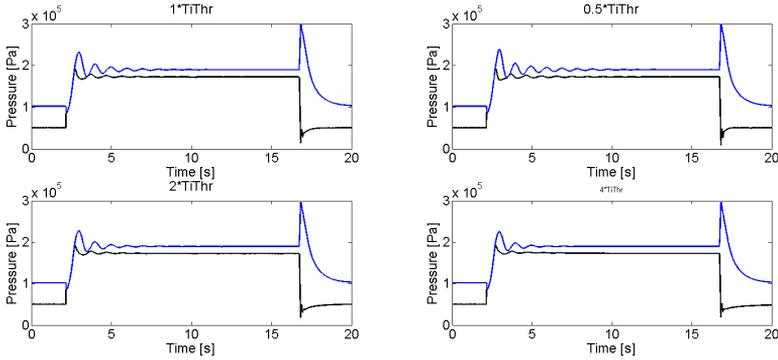
**Figure 3.16.** Pressure response with varying integration time at the throttle controller. The four responses are pretty much the same, but the oscillations damps out faster with a bigger integrational time  $TiThr$ .
