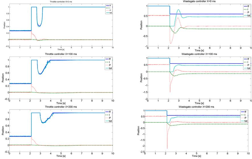
**Figure 4.2.** Throttle controller to the left and wastegate controller to the right. The blue is the feedforward part, red is the P-part and green is the I-part. The cyan is the total saturated control signal. The control signals, from the top row to the bottom row, X=0 ms, X=100 ms and X=200 ms.
