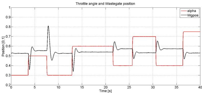
**Figure 3.12.** Wastegate and throttle position - Throttle controller off, wastegate controller on. The red line shows the numerous of step in throttle angle. The black line shows the controlled wastegate position. The wastegate controller reacts hard and overcompensate for the control error, causing the overshoot and the oscillation in  $p_{ic}$  shown in Figure 3.11.
