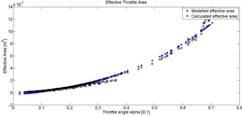
**Figure 2.5.** Validation of the throttle effective area model. Blue marks the model and black the calculated effective area. The model shows a good approximation for  $0 < \alpha < 0.65$  and but loses in accuracy for  $\alpha > 0.65$ . The measured data only supplied measurements for throttle angle up to 0.7
