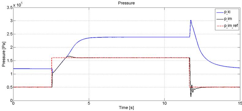
**Figure 3.9.** Pressure - Throttle controller on, wastegate controller off. There is a small overshoot in  $p_{im}$  but no oscillations. The fixed wastegate position give the  $p_{ic}$  response to be slow and that makes the  $p_{im}$  response slow.
