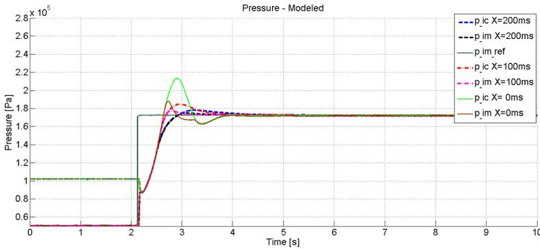
**Figure 4.1.** Pressure response with compensating controller. Without the compensation ( $p_{ic}$  green,  $p_{im}$  brown) the figure shows that both pressures overshoots and undershoots before it settles at the target value. For X=100ms the compensation reduces both the  $p_{ic}$  (red) and  $p_{im}$  (magenta) overshoots and removes the undershoots altogether. For X=200ms the  $p_{ic}$  (blue) and  $p_{im}$  (black) overshoots is even more reduced but the bigger X makes the response slower.
