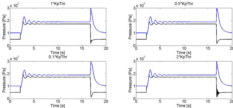
**Figure 3.15.** Pressure response with varying proportional gain at the throttle controller. The pressure response is pretty much the same for all four different  $KpThr$ , showing both overshoots and oscillations.
