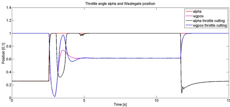
**Figure 3.24.** Throttle angle alpha (red and black) and wastegate position (magenta and blue). Red and magenta shows the position when the throttle is set to not cut the flow. Black and blue shows position when the throttle cuts the flow. When the throttle cuts the flow, the throttle angle goes from 1 to about 0.35 and back to 1 and the wastegate controller reacts harder as a result of the bigger overshoot in  $p_{ic}$ .
