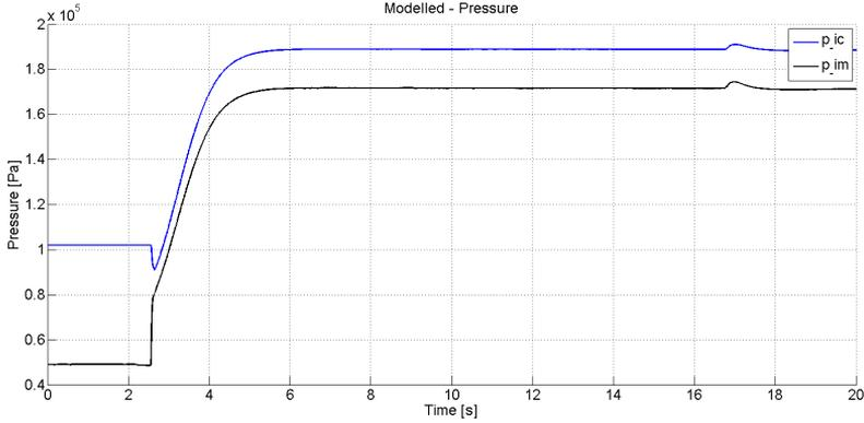
**Figure 3.7.** Pressure - Throttle controller off, wastegate controller off. There are no overshoots or oscillations in either  $p_{ic}$  or  $p_{im}$ . The bulb on the pressure lines at  $t=17$ s is caused by the dip in engine speed seen in Figure 3.1
