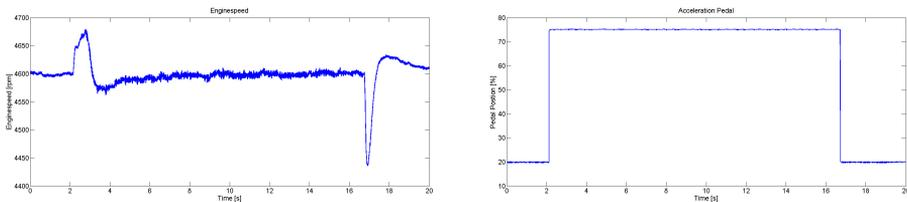
**Figure 3.1.** Engine speed to the left and step in acceleration pedal position to the right. Both these inputs is taken from the measurements. The engine speed is aimed to be constant 4600 rpm and a step in acceleration pedal position from 20-75%.
