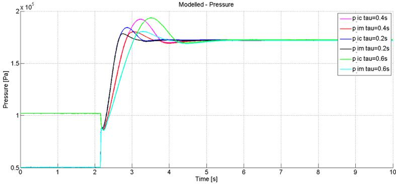
**Figure 3.29.** Pressure response with first-order system as delay and dynamics in the turbocharger. A bigger time constant,  $\tau$ , causes the pressure response to get slower and slower, but it also causes the pressures to overshoot more, which is most apparent in  $p_{ic}$ , but  $p_{im}$  also gets a slightly bigger overshoot for a bigger  $\tau$ . The settling time before the pressures have settled at the target value increases with increased  $\tau$ .
