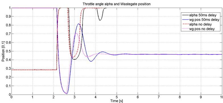
**Figure 3.26.** Control signals with delay in pressure sensors compared to no delayed sensors. The figures shows that the control signals reacted slower and more heavily.
