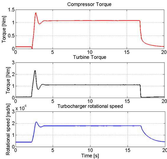
**Figure 3.4.** Top: Compressor braking torque. Middle: Turbine driving torque. Bottom: The resulting turbocharger rotational speed. All three subplots are linked together, the turbine driving torque, which accelerates the turbocharger rotational speed and the compressor braking torque which decelerates the turbocharger rotational speed. The three subplots shows that the oscillations in present in the turbocharger system as well as the pressure system.
