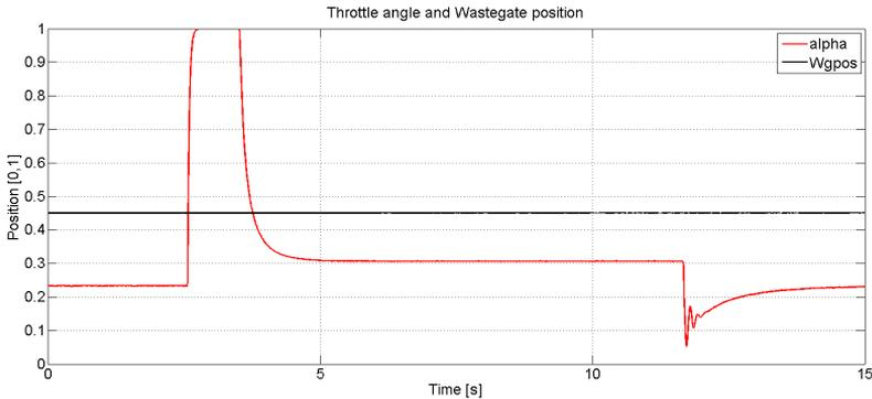
**Figure 3.10.** Wastegate (black) and throttle angle (red) - Throttle controller on, wastegate controller off. The wastegate position is held fixed at 0.45 at all times. The throttle starts at a constant value and when the step comes, the throttle gets fully open. When it has reached its target value, the throttle cuts the flow by closing and slowly decreasing and reaching a constant value.
