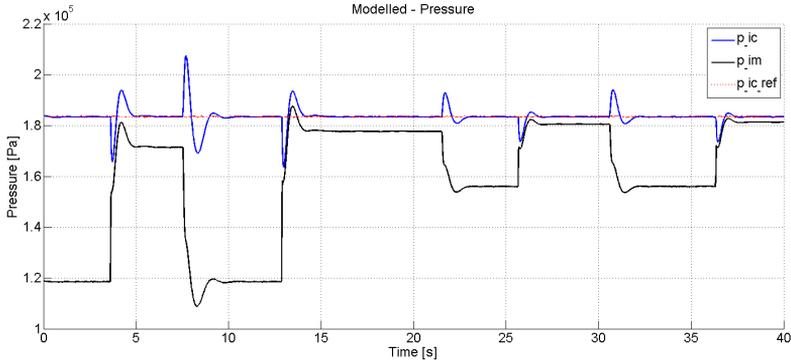
**Figure 3.11.** Pressure - Throttle controller off, wastegate controller on.  $p_{im}$  overshoots in every step, which is caused by the wastegate controller overshoots in its attempt to keep  $p_{ic}$  constant.  $p_{ic}$  shows an oscillatory behavior before it reaches its target value, caused by the pressure drop when the throttle opens and the resulting overcompensation that causes the overshoot.
