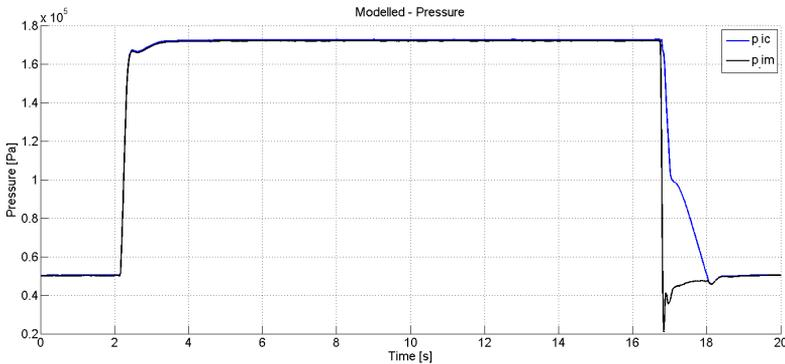
**Figure 3.27.** Pressure response with no delays in the turbocharger. Intercooler pressure,  $p_{ic}$  (blue) and intake manifold pressure  $p_{im}$  (black). The pressures follow each other and the step responses are fast without overshoots or oscillations. There is a small bulb on the pressure response caused by the controller, see Figure 3.28.
