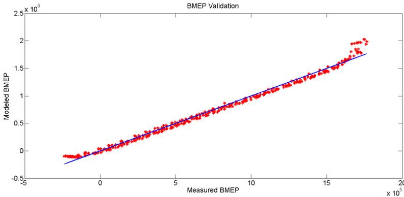
**Figure 2.7.** Validation of the BMEP model. The blue line is the ideal model, while the red stars represent measured BMEP plotted against the modeled BMEP. The figure shows a good agreement, the red dots is place around the ideal blue line.
