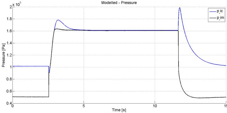
**Figure 3.17.** Step response in pressure without actuator dynamics. There is basically no overshoot in intake manifold pressure (blackline) but there is still a overshoot in intercooler pressure (blueline). At the end of the step, around  $t = 12s$ , the effects of a missing surge valve is seen, causing the  $p_{ic}$  to rapidly increase when the throttle is closed. With a surge valve, the pressure could have been dumped and the  $p_{ic}$  would have decreased faster.
