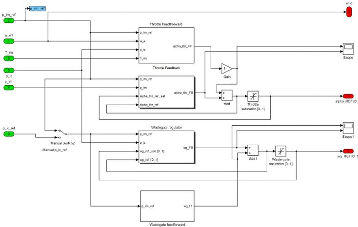
**Figure 2.9.** An overview of the ECU. From the top down, throttle feedforward, throttle PI-controller, wastegate PI-controller and wastegate feedforward.
