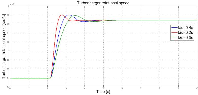
**Figure 3.31.** Turbocharger rotational speed with different time constants at the first-order system. A bigger delay gives a slower response but about the same in the overshoot height in all three simulations.
