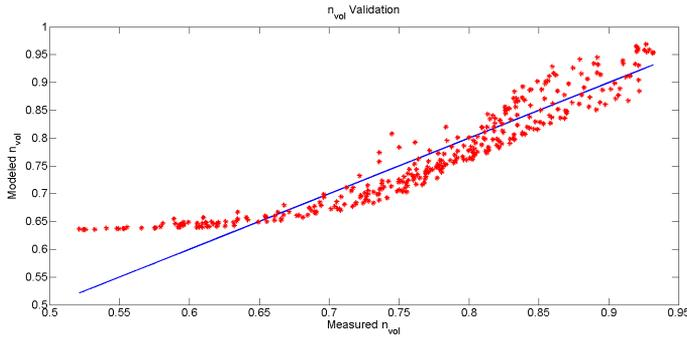
**Figure 2.8.** Validation of  $\eta_{vol}$ -model. The blue line represent a perfect model and the red stars is the result of plotting the measured  $\eta_{vol}$  against the modeled  $\eta_{vol}$ . The model gives a decent approximation for  $\eta_{vol}$  over 0.65 seen as the red dot is centered around the blue ideal line.
