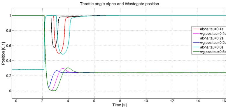
**Figure 3.30.** Control signals with first order system as delay and dynamics for turbocharger. The delays causes both control signals to act later and harder to compensate for the delayed response.
