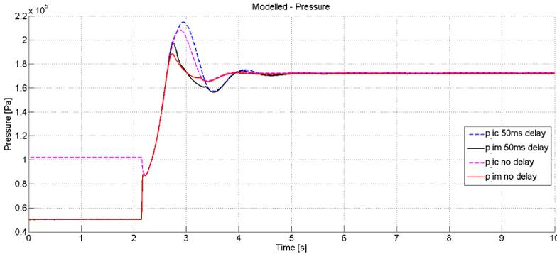
**Figure 3.25.** Pressure response with delay in pressure sensor compared to no delayed sensor. The figures shows both pressures giving a higher overshoot and more oscillations with delay.
