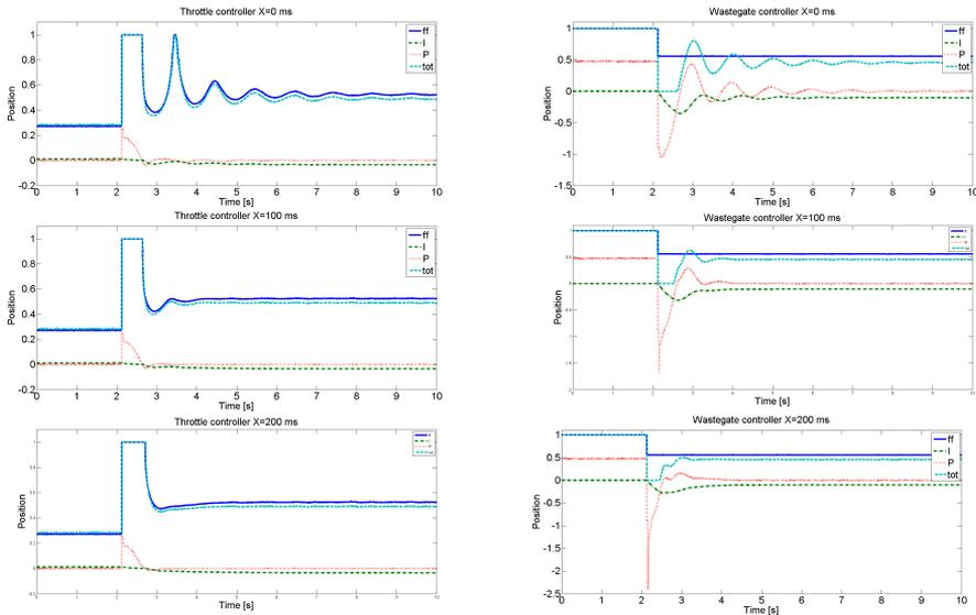
**Figure 4.4.** Throttle controller to the left and wastegate controller to the right. The blue is the feedforward part, red is the P-part and green is the I-part. The cyan is the total saturated control signal. The control signals, from the top row to the bottom row,  $X=0\text{ ms}$ ,  $X=100\text{ ms}$  and  $X=200\text{ ms}$ .
