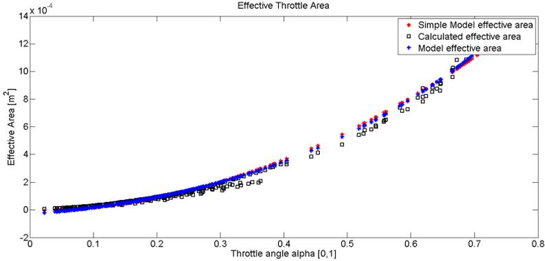
**Figure 2.6.** Validation of the simple effective area model. Red marks the simple model, blue the more complex model and black the calculated effective area. The simple model gives a less accurate approximation of the calculated effective area than the more complex effective area model. But it still gives a good approximation.
