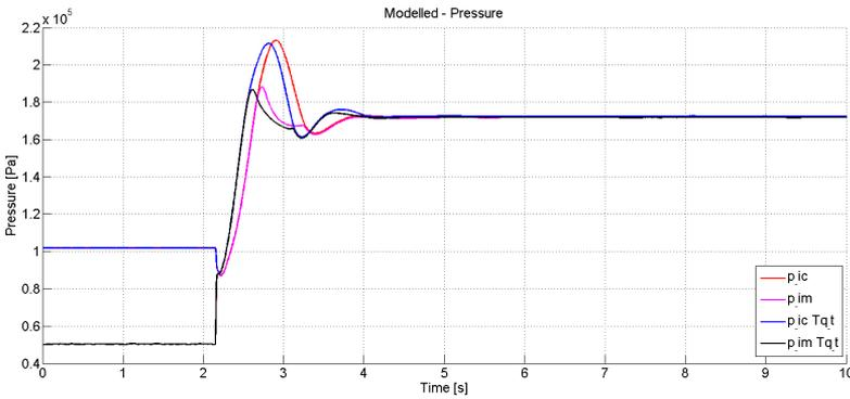
**Figure 3.32.** Pressure response. Red and magenta is with normal configuration. Blue and black is for the wastegate controlling turbine torque configuration. The wastegate controlling the turbine torque directly gives a faster response, but the characteristics of the pressure responses is the same as for the conventional configuration.
