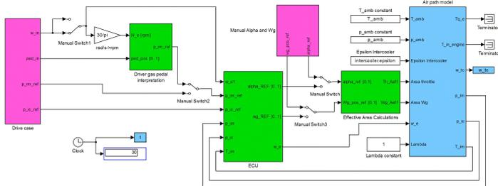
**Figure 2.1.** An overview of the entire model. The magenta colored blocks are for manual input, the green blocks are from the left; Driver gas pedal interpretation, ECU and effective area calculations. The blue block is the air path model.
