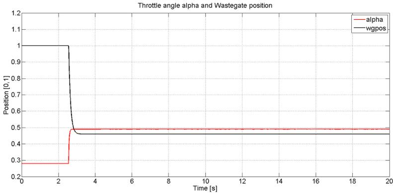
**Figure 3.8.** Wastegate and throttle position - Throttle controller off, wastegate controller off. Step from 1 to 0.46 in wastegate position and a step from 0.28 to 0.49 in throttle angle. The corresponding pressure response is shown in Figure 3.7.
