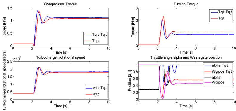
**Figure 3.33.** Top left: Compressor torque. Top right: Turbine torque. Bottom left: Turbocharger rotational speed. Bottom right: Throttle angle and wastegate position. The colors marked  $Tq-t$  is the simulations with wastegate controlling the turbine torque. The other is the normal configuration. When controlling the turbine torque directly, all responses are a little bit faster than the normal configuration, but the characteristics is the same for both cases.
