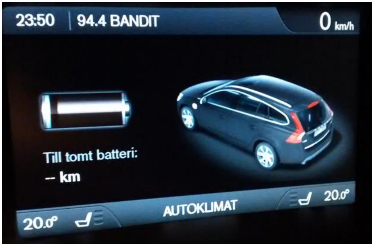
Figure 7: The infotainment display showing a totally depleted battery.
