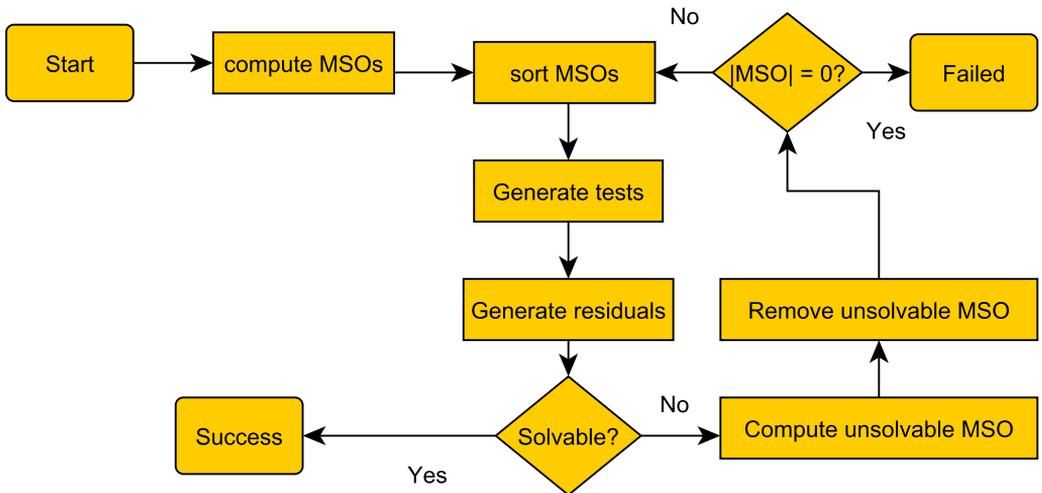
*Figure 4.1: General view of the diagnostic system generation*
