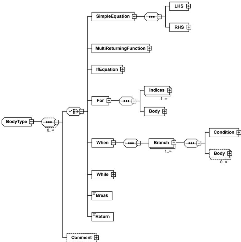
Figure A.4: All Body types that can be present in ModelicaXML.
