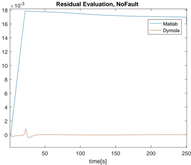
**Figure 5.2:** Evaluation of a Non-algebraic Residual in Matlab and Dymola
