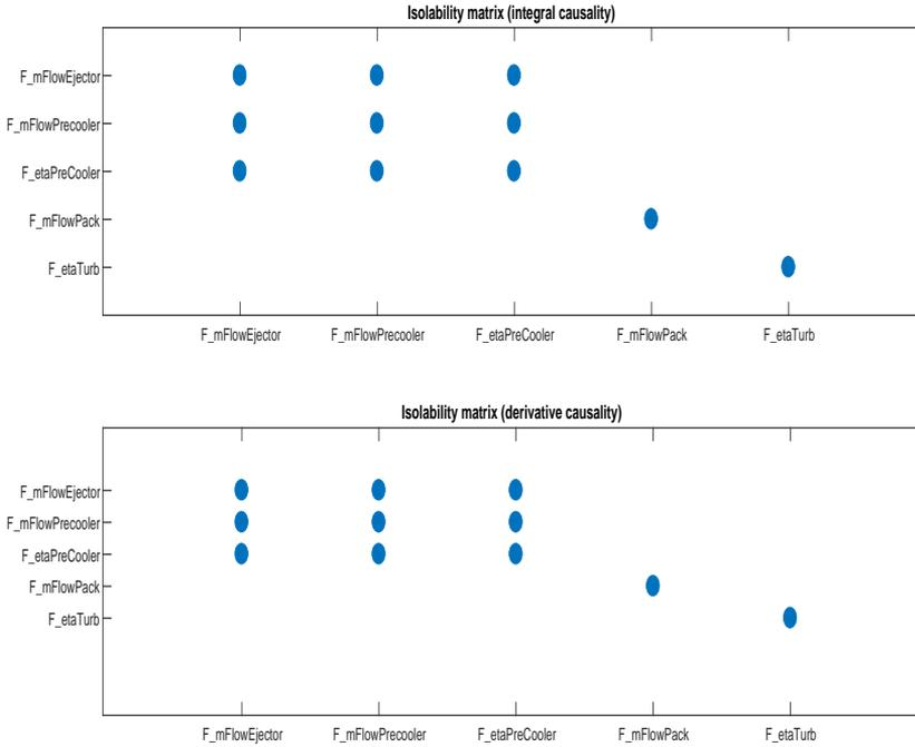
**Figure 5.6:** The Isolability potential of a Diagnostic system, given the sensors provided in SECS and causality restrictions
