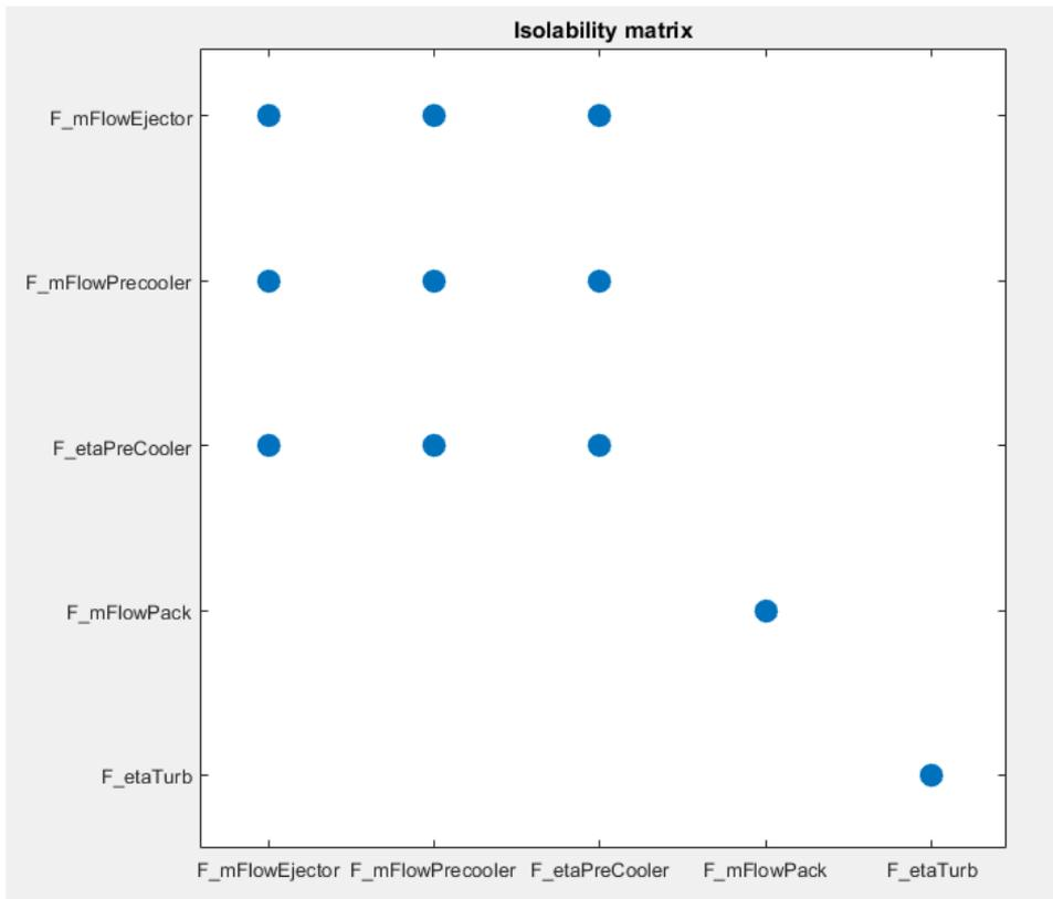
**Figure 5.5:** The Isolability potential of a Diagnostic system, given the sensors provided in SECS and no causality restrictions
