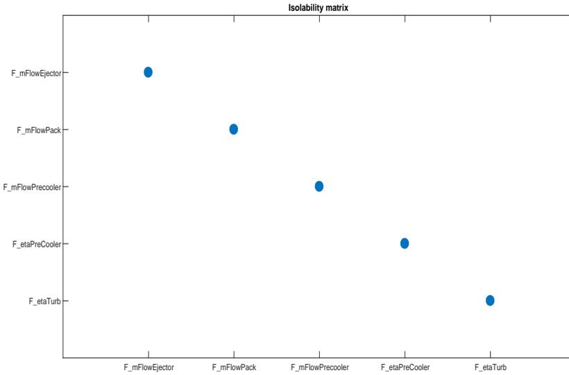
**Figure 5.7:** The Isolability potential of a Diagnostic system, after adding additional sensors to the sensors provided in SECS and no causality restrictions
