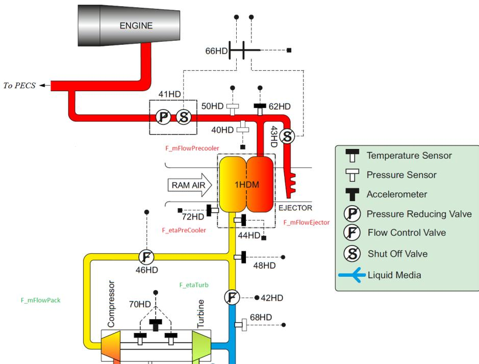
**Figure 3.8:** *The SECS model with faults of Table 3.3 implemented*
