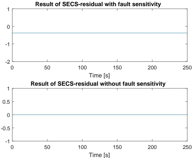
**Figure 5.9:** Residual result of two Algebraic residuals based on SECS with no faults present
