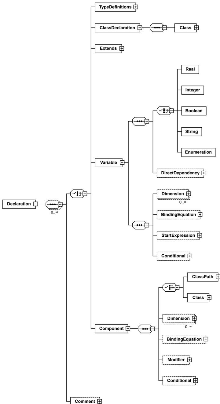
Figure A.3: The element *Declaration* and its children with the child elements *Variable* and *Component* expanded.
