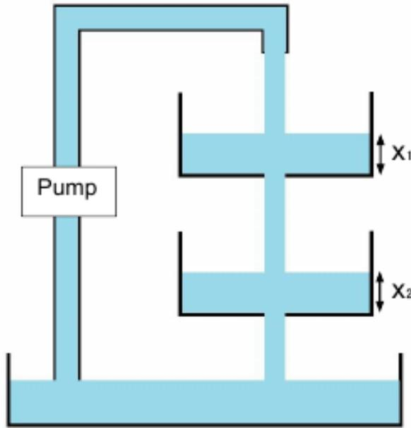
**Figure 3.6:** Schematics of the coupled two-tank system. Source [15]
