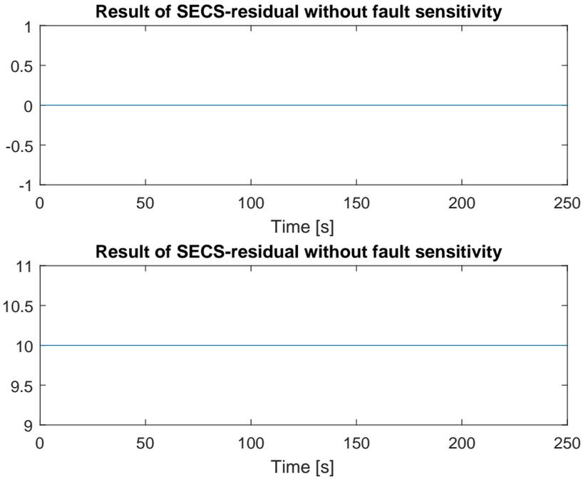
**Figure 5.10:** Non-sensitive Residual response to  $F\_mFlowPack$  and  $F\_nonmon$
