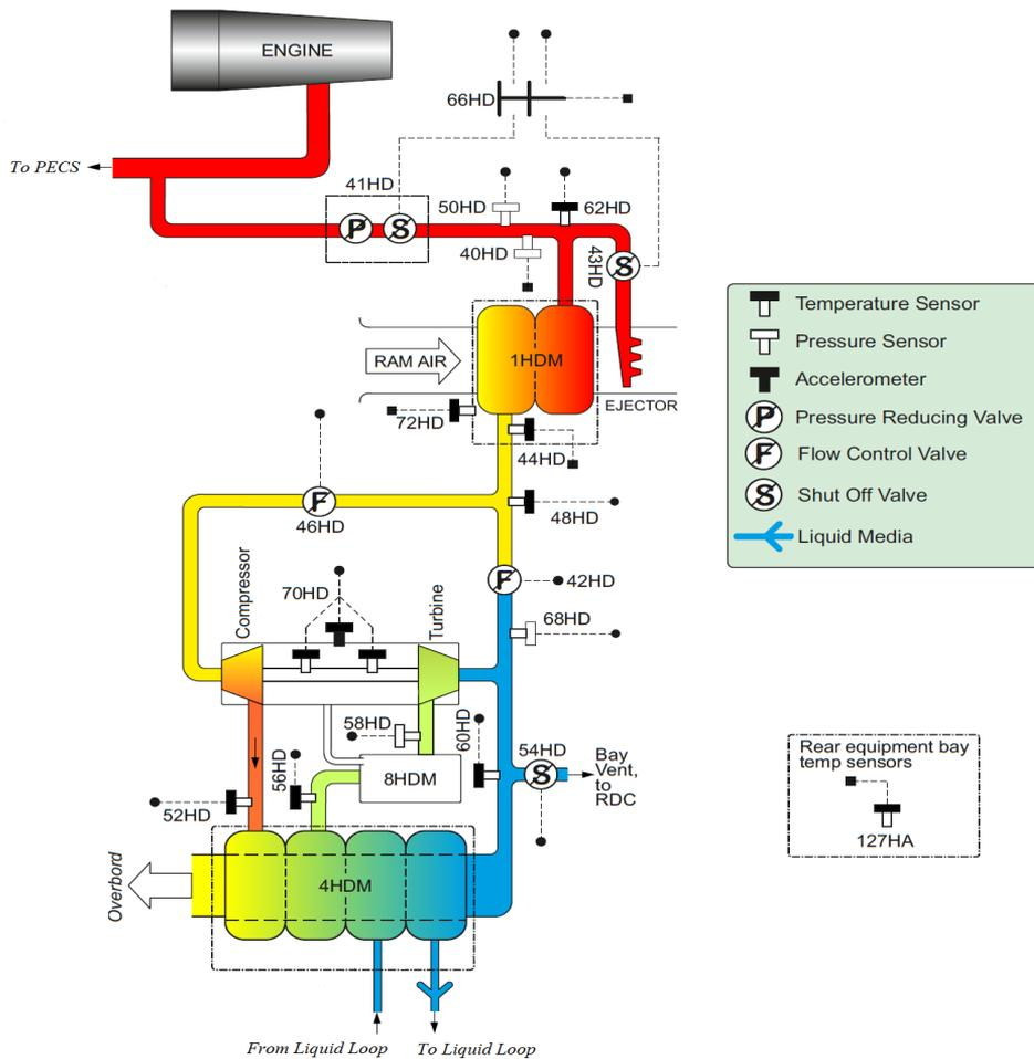
**Figure 3.7:** Schematic of the Secondary Environmental Control System.
