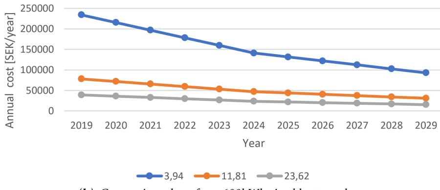
**Figure 4.22:** Yearly costs of three different cases where the expected number of cycles a battery lasts differs; 500, 1500 and 3000 cycles. Where the lifetime of these are 3.94, 11.81 and 23.62 years respectively. The years on the y-axis represent projections for price drops in li-ion batteries.
