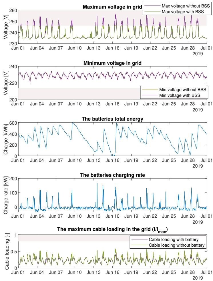
**Figure 4.17:** Illustration of maximum and minimum voltage, SoC variations and cable loading for a stationary battery in node 70. Note that the day that dimensions the size of the battery capacity is June 16 (the charge reaches both the top and bottom during this day) and that the battery reinforced grid behaves similarly to the cable reinforced grid, in terms of cable loading as well as maximum and minimum voltage.
