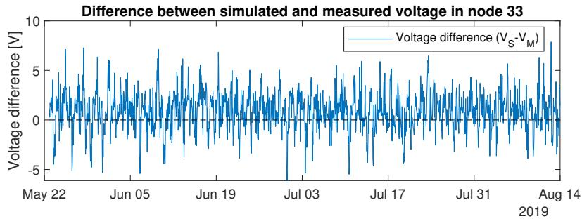
(a) The difference between the simulated voltages and the voltages measured by Tekniska verken. The interval is the chosen interval for validation.
