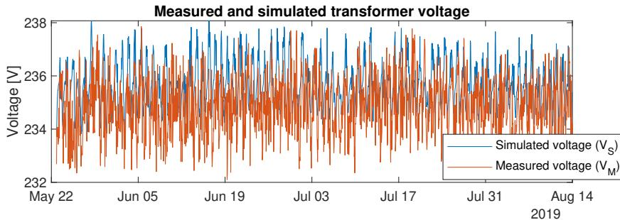
(a) The simulated voltages and the voltages measured by Tekniska verken. The interval is the chosen interval for validation.
