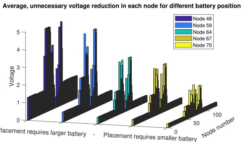
(b) Same as 4.14a but without showing the voltages that had to be reduced in order to stay under the voltage constraints. This means that the voltage reductions shown are reductions that were not necessary to make for the individual nodes. However, there might always have to be unnecessary reductions unless only one battery can lower the voltage in all nodes to just below +7% of 230 V.
