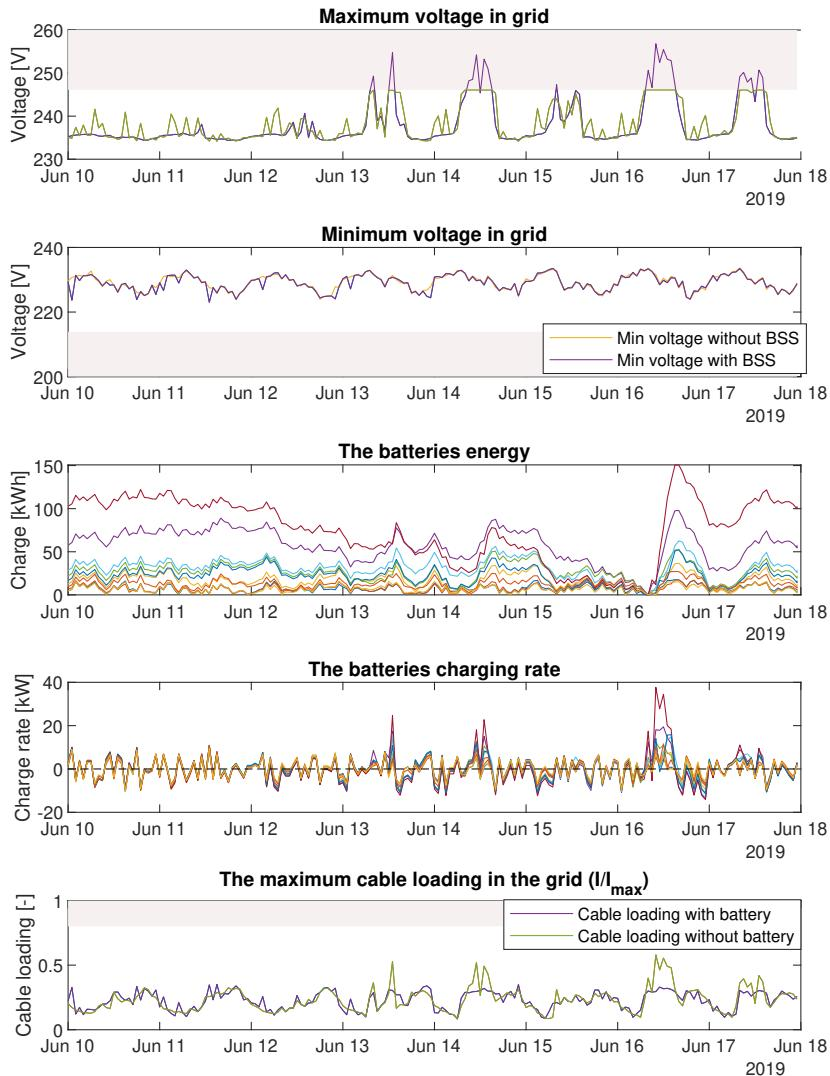
**Figure 4.16:** Placement of 10 batteries in the grid.
