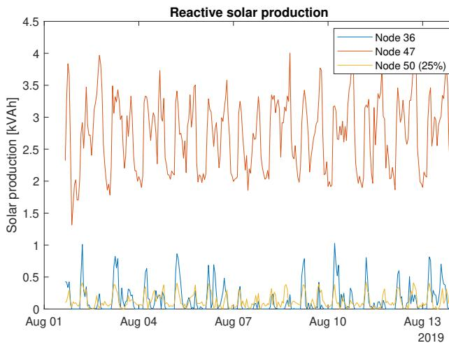
(b) Graph showing the reactive solar power production of the three PV-systems which has hour based data.
