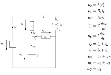
10 equation in 10 unknown  $(u_0, u_1, u_2, u_L, u_C, i_0, i_1, i_2, i_L, i_C)$  model Circuit
