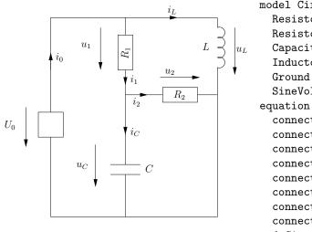
model Circuit Resistor R1; Resistor R2; Capacitor C; Inductor L; Ground G; SineVoltage src; connect(G.p, src.n); connect(src.p, R1.p); connect(src.p, L.p); connect(R1.n, R2.p); connect(R1.n,C.p); connect(L.n,R2.n); connect(L.n, C.n); connect(C.n,G.p); end Circuit;
