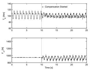
Figure 5: Brake torque variation compensation using the first-order compensator for a fixed wheel rotation speed of 60 rpm (1 Hz).
