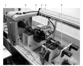
Figure 3: Brake dynamometer. The individual components are: 1. Dynamometer motor; 2. CAN cable; 3. Disc rotor; 4. EMB; 5. Thermometer connected to a thermocouple embedded in the brake pad; 6. Torque sensor.
