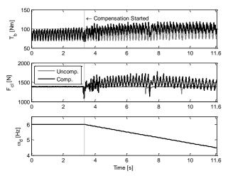
Figure 7: Brake torque responses with and without compensation under fixed brake torque reference (100 Nm) and varying wheel speed.
