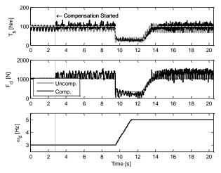
Figure 8: Brake torque responses with and without compensation under varying brake torque reference (dash grey line) and varying wheel speed.
