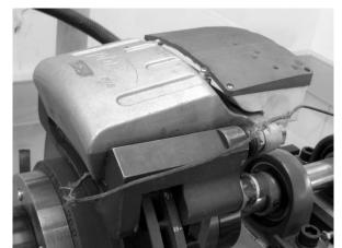
Figure 1: The production-ready electromechanical brake prototype used in this work.
