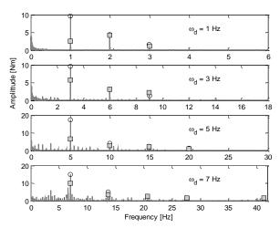
Figure 6: Amplitude spectrum of brake torque trajectories before (circles) and after (squares) compensation.
