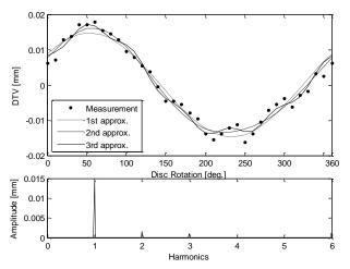
Figure 4: (Top) Disc thickness variation measurements and the first three orders of approximation. (Bottom) Amplitude spectrum of the disc thickness variation profile.
