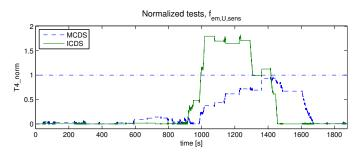
Fig. 4. The normalized test quantities when a fault is induced in the voltage sensor in the electric machine after 400 seconds. The test quantity in the MCDS is almost above the threshold, but the test does not alarm. The test in the ICDS reacts approximately 600 seconds after the fault is induced.
