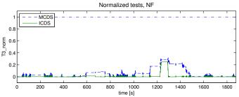
Fig. 3. The normalized test quantities in Tests 3 in the two diagnosis systems based on mixed and integral causality when the system is fault free. The tests react if the signal is above one. No false detection occurs in the diagnosis systems and the test quantities are well below the thresholds. Similar results are achieved in Tests 4.
