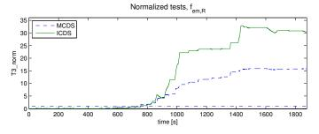
Fig. 5. The normalized test quantities when  $f_{em,R}$  is induced in the model after 400 seconds. Both diagnosis systems react about 350 seconds after the fault is induced in the simulation model. The magnitude of the test quantity in the ICDS is almost twice that of the MCDS at the end of the simulation.
