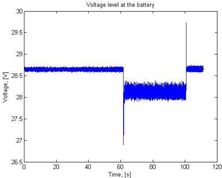
**Figure 1: The battery voltage charging level during 2 minutes, with a load of 10 A on the system. A voltage drop occurs after 1 minute when a load of 140 A is applied to the system that is turned off at 100 seconds.**
