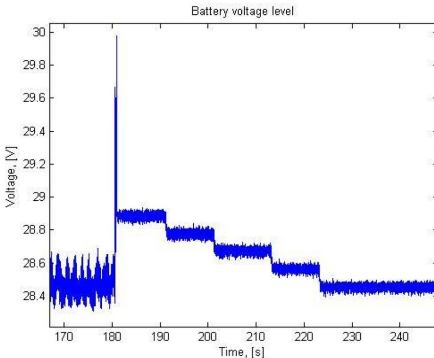
**Figure 37: A large power consumer is turned off after 180 s, the voltage is stepped down to the desired level.**
