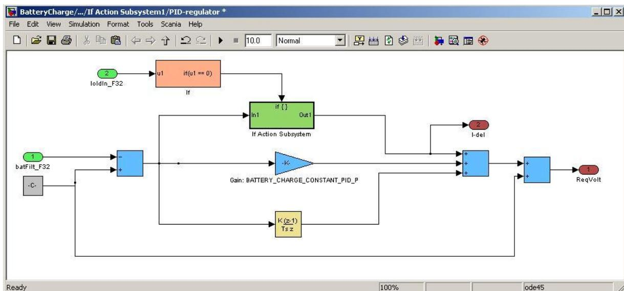
Figure 34: Simulink blocks of the PID controller, implemented on parallel form
