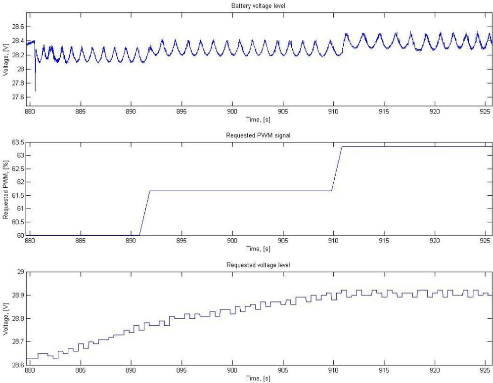
**Figure 26: Step response of the system, the third curve is the control signal expressed as voltage, the second curve is the control signal, expressed in per cents for the PWM-signal and the top curve is the voltage level at the battery. The peak that appears in the beginning of the battery voltage level curve is caused by that a load is put on the system, that lower the voltage level, and the control system rise the voltage to the correct level.**
