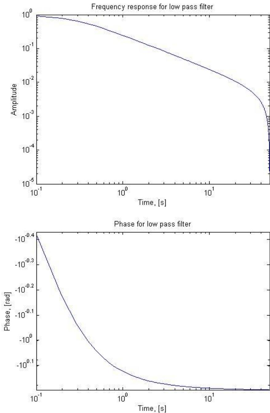
**Figure 9: Frequency response, amplitude in top graph and phase in bottom graph for the low pass filter applied to the signal before being decimated and used in the control system.**
