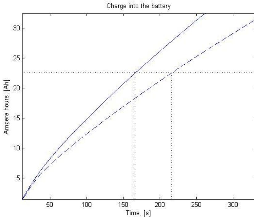
**Figure 40: The time for charging the batteries with 22.5 Ah with the control system, solid line and without the control system, dashed line.**
