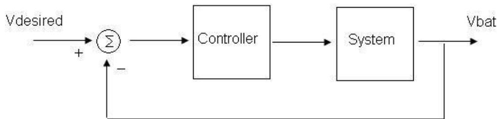
**Figure 22: The control strategy, a feedback loop, with the desired voltage level as input and the battery voltage level, calculated from the Coordinator voltage measurement as output and feedback signal.**
