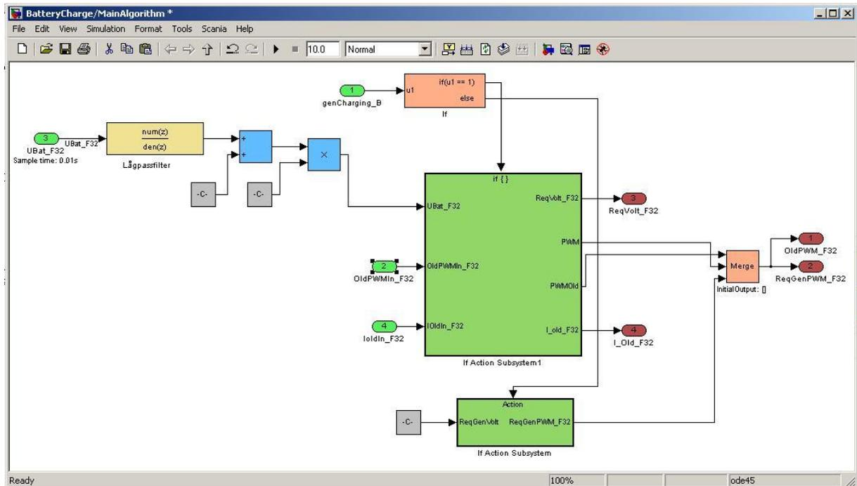
**Figure 32: Simulink blocks for the main algorithm of the control system.**
