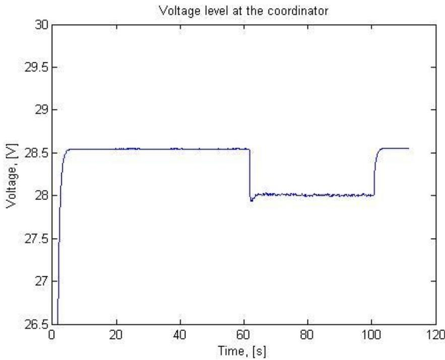
**Figure 12: The voltage level in the Coordinator from Figure 11, after applying Butterworth filter and decimating the signal.**
