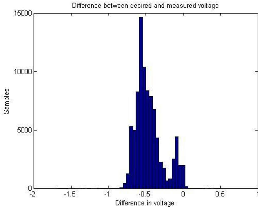
**Figure 35: Histogram of distribution of the difference between the desired voltage level and the battery voltage level when the control system is not used for the test drive in verification test 1.**
