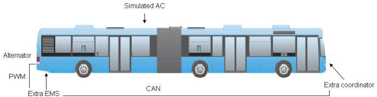
**Figure 30: The information flow for the implemented function in the bus, the extra Coordinator is placed in the front of the bus and the extra EMS is placed in the back of the bus, by the engine.**
