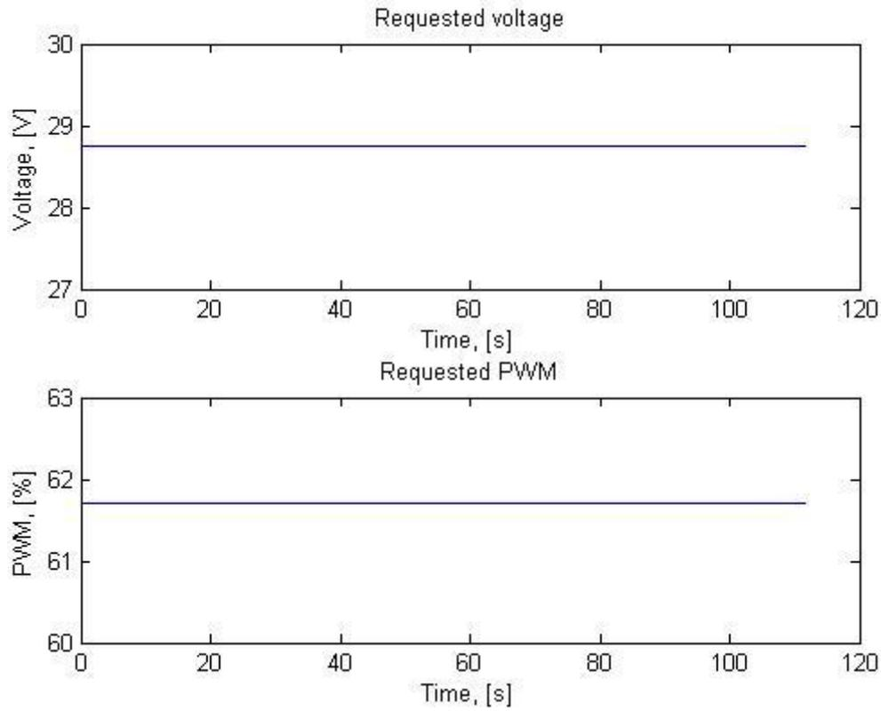
**Figure 8: During the sequence in Figure 7 the demanded PWM signal from the alternator is 61.7%, which corresponds to a demanded voltage of 28.76 V.**
