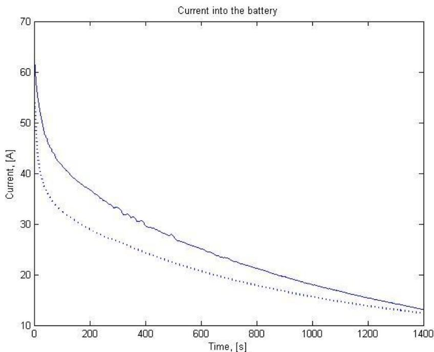
**Figure 38: Current into the battery. The dotted curve is the current into the battery during charging when the control system is not used, while the solid curve is when the control system is being used and a higher charging voltage level is applied.**
