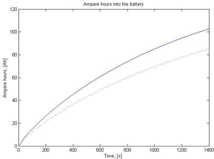
**Figure 39: Ampere hours into the battery during verification test 2, the dotted line is when the control system is not being used and the solid line is when the control system is used.**
