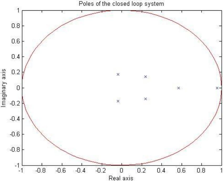
**Figure 28: Pole placement for the discrete closed loop system with no extra load applied to the system. The circle shows the stability limit and the crosses represent the poles.**
