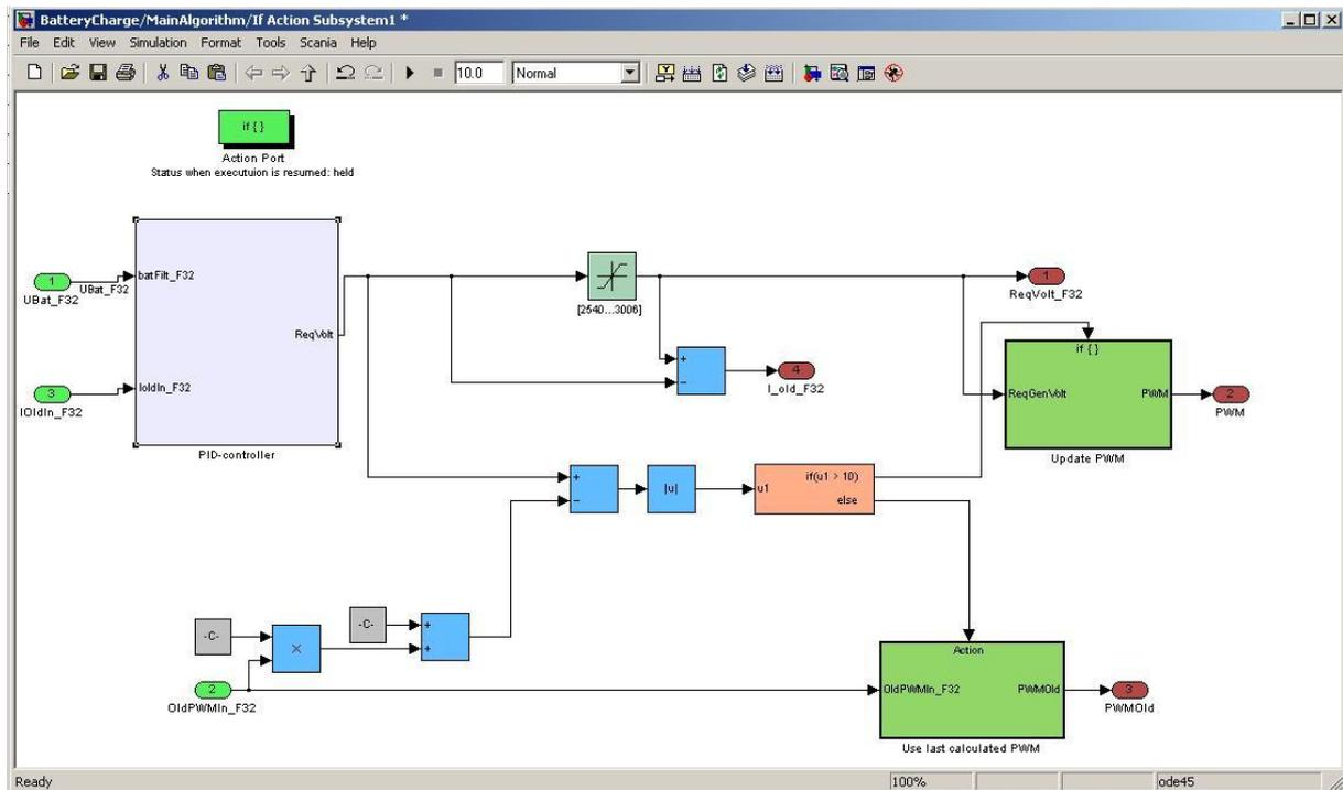
Figure 33: Simulink blocks of the control system
