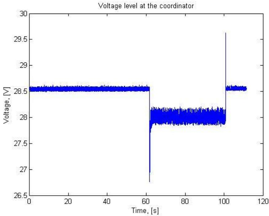
**Figure 11: Voltage level measured in the Coordinator without filtering and decimation when a load is put on the system at 60 seconds and the load is put off at 100 seconds.**
