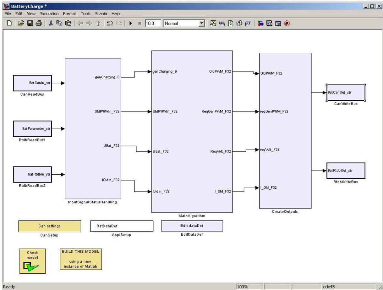
Figure 31: Simulink blocks of the control system, inputs and outputs.
