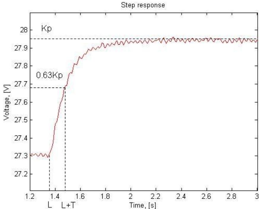
**Figure 24: A step response of the open loop system, used for calculating the parameters for the PID controller.**
