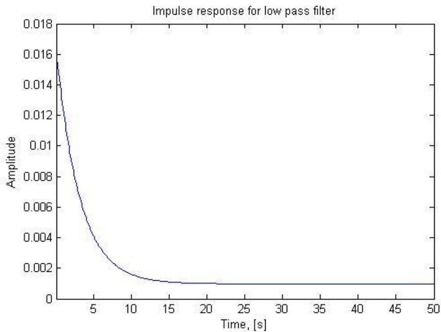
**Figure 10: Impulse response for the low pass filter, the impulse response is zero when  $t < 0$  implying that the filter is causal.**
