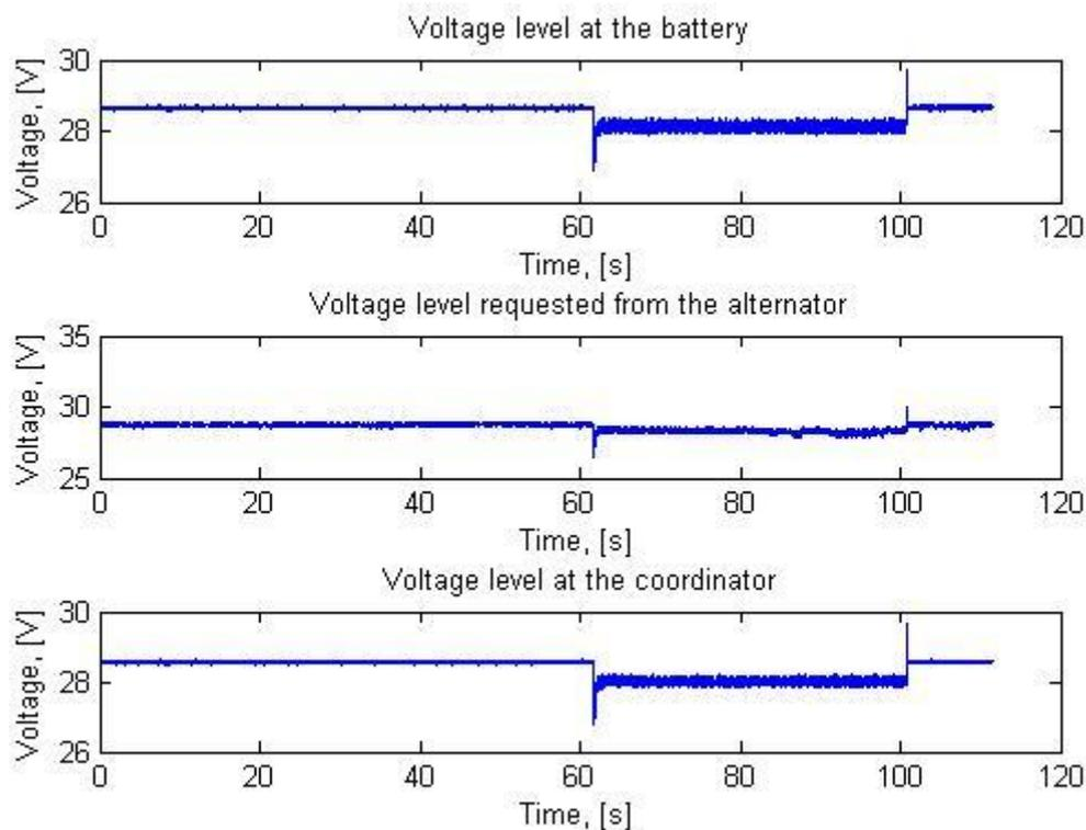
**Figure 7: Data of the measured voltages, with a voltage drop after approximately 60 seconds when the air condition units are turned on and turned off again at about 100 seconds. The top graph is the voltage level at the battery, the graph in the middle is the output voltage from the alternator and the graph at the bottom is the voltage level measured at the Coordinator.**
