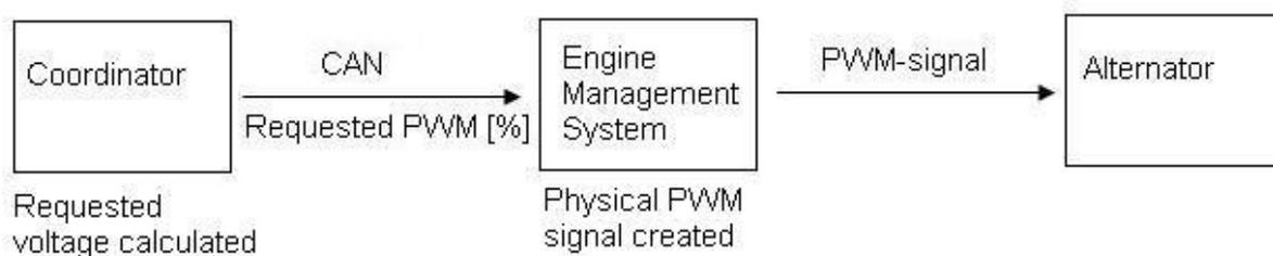
**Figure 2: The information flow in the system, the desired voltage level from the alternator is calculated in the Coordinator, the value is recalculated into per cents and sent to the EMS where the pulse width modulated signal is created and sent to the alternator.**
