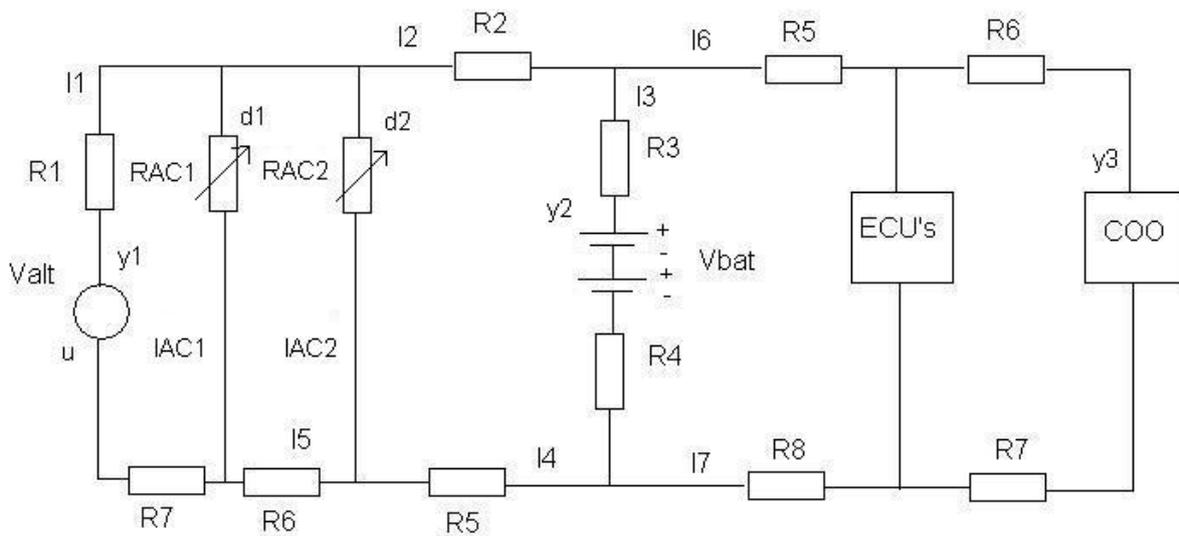
**Figure 3: Schematic figure of the system. In this system one air condition unit is connected in front of the articulation, AC1, of the bus and one air condition unit is connected behind the articulation, AC2. The voltage  $V_{at}$  is the output voltage from the alternator.**
