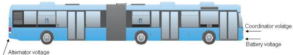
**Figure 5: Measurement setup on the articulated bus. Three voltages are measured, the battery voltage level and the Coordinator voltage level in the front and the alternator voltage level in the rear of the bus.**
