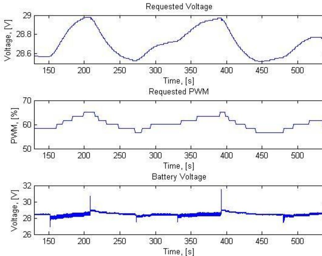
**Figure 25: The top graph is the control signal in voltage, the second curve is the control signal in per cents, i.e. the requested PWM signal, and the third curve is the battery voltage.**
