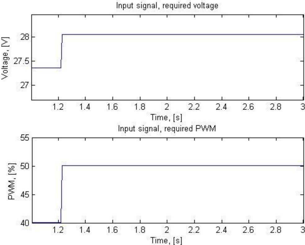
**Figure 23: Input signal to the system when obtaining the step response in Figure 24, The top graph is the requested voltage and the lower graph is the requested voltage recalculated into per cents.**
