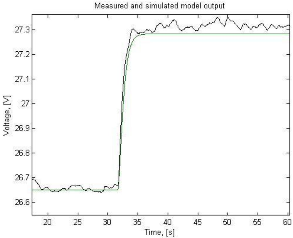
**Figure 20: Cross validation for the second black box model, the solid line is the output from the model and the uneven line is the real value of the battery voltage, sent through the low pass filter as explained in Section 3.4, Data processing.**
