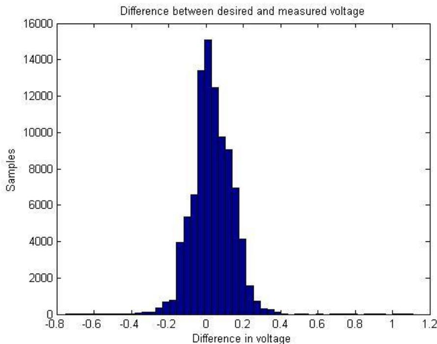
**Figure 36: Histogram of distribution of the difference between the desired voltage level and the battery voltage level when the control system is used for the test drive in verification test 1.**
