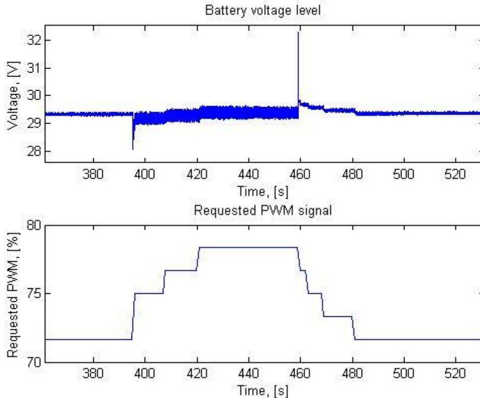
**Figure 27: The desired voltage is 29.3 Volts, after 395 seconds 140 ampere is applied to the system and after 460 seconds the load is turned off.**
