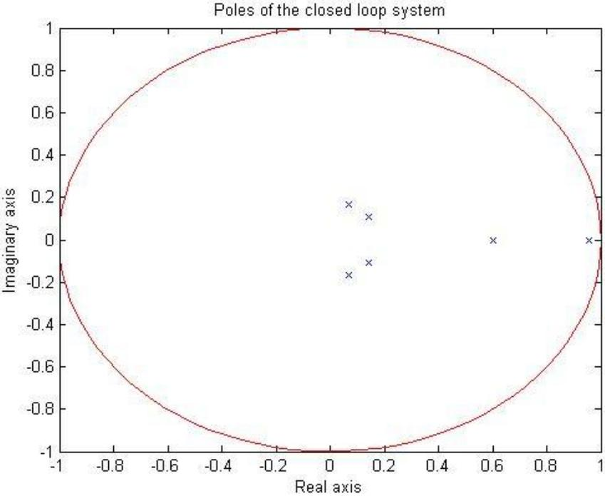
**Figure 29: Poles of the closed loop system with the model with full load on the system.**
