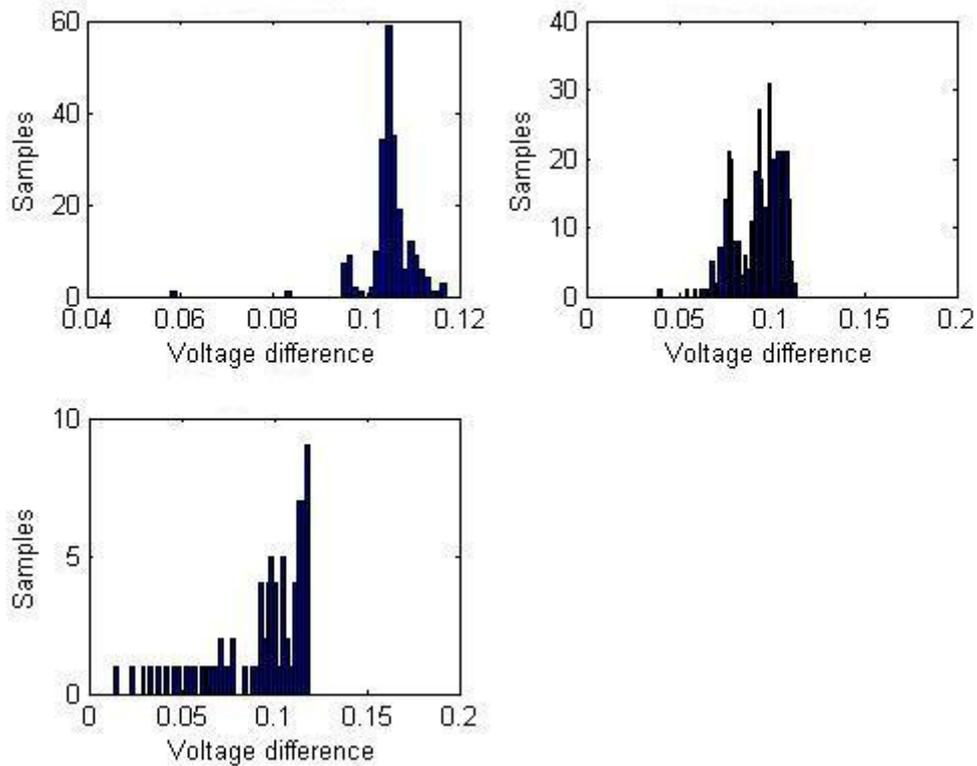
**Figure 16: Histogram of the statistic difference between the battery voltage level and the Coordinator voltage level from Figure 13 and 14.**
