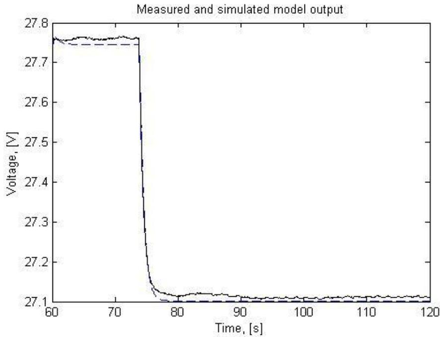
**Figure 18: Cross validation for the black box model, the dashed line is the output from the model and the solid line is the filtered value of the battery voltage.**
