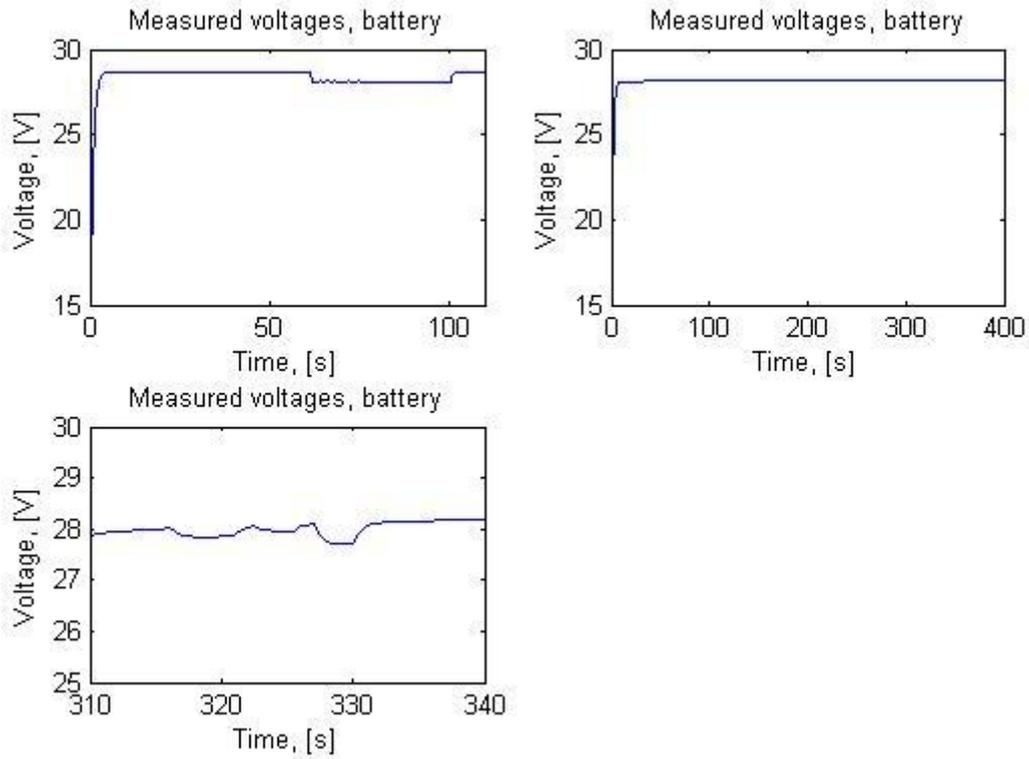
**Figure 13: Three different voltage measurements at the battery, with different loads on the system during different periods of time**
