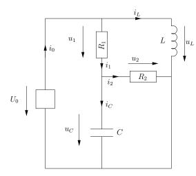
$$x_1 = (u_c, i_L), x_2 = (u_2, i_2, u_0, u_1, u_L, i_1, i_C, i_0)$$
