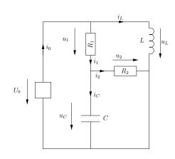
$u_{0} = f(t)$   $u_{1} = R_{1}i_{1}$   $u_{2} = R_{2}i_{2}$   $i_{C} = C\frac{du_{C}}{dt}$   $u_{L} = L\frac{di_{L}}{dt}$   $i_{0} = i_{1} + i_{L}$   $i_{1} = i_{2} + i_{C}$   $u_{0} = u_{1} + u_{C}$   $u_{L} = u_{1} + u_{2}$   $u_{C} = u_{2}$
