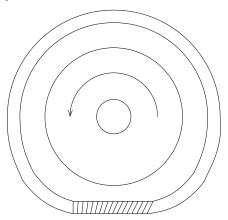
The contact patch is assumed to rectangular and can be divided into an adhesion region  $(0 \le x \le l_c)$  and a sliding region  $(l_c \le x \le l_t)$ .
