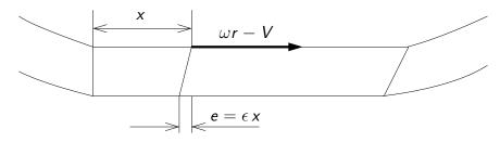
The velocity at the rim is  $\omega r - V$ . The time since the bristle first touch the ground is  $t = x/(\omega r)$ . The deflection at the distance x is:
