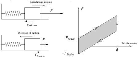
The energy loss due to hysteresis is equal to the shaded in the figure:
