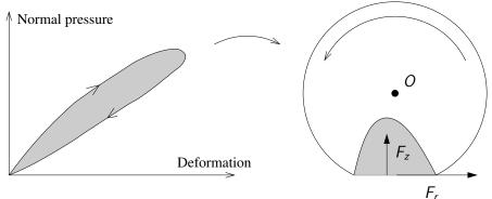
The applied wheel torque on free-rolling tire is zero. Therefore, a horizontal force  $R_r$  at the contact patch must exists to maintain equilibrium. This force is called known as the rolling resistance.
