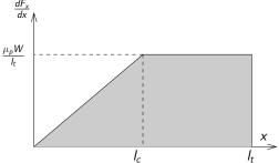
How do we calculate the length of the adhesion region  $I_c$ ?
