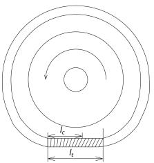
The objective is to find the length of the adhesion region  $I_c$ . When does the longitudinal force becomes so large that the bristles begins to slide?
