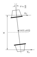
Lateral drift causes a difference in the longitudinal velocity of the wheels in the same way as before:
