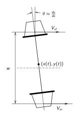
Using  $V_{xl} = (r_0 + \psi y)\omega$  and  $V_{xr} = (r_0 - \psi y)\omega$  the angular velocity can be written as
