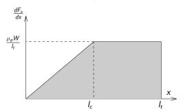
The longitudinal force is equal to the shaded area
