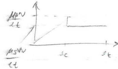
$$b) F_x = \frac{1}{2} d_c \frac{MPW}{l_t} + (l_t - d_c) \frac{MPW}{l_t} \approx 2,2 \text{ kN}$$
