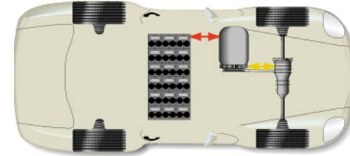
Sketch of the energy paths (Thin=Electric, Thick=Mechanic)
