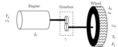
$$T_e - J_e \frac{d}{dt} \omega_e = T_{gb} \quad T_{gb} \cdot \gamma - J_w \frac{d}{dt} \omega_w = T_t$$
