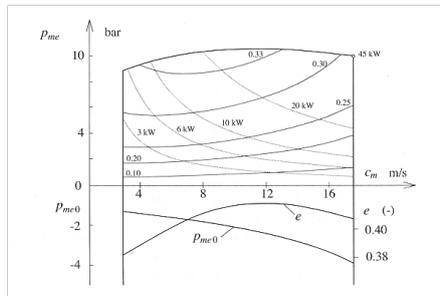
Willans line parameters:  $e(\omega_e) \quad p_{me,0}(\omega_e)$
