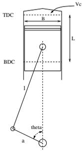
Cylinder, Piston, Connecting rod, Crank shaft
