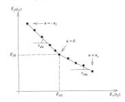
Slopes determine s<sub>dis</sub> and s<sub>chg</sub>.
