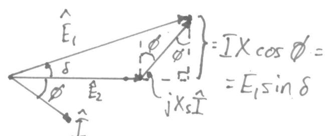
$$\delta = \text{effektrinkel} = \text{fasvinkel}(\hat{E}_1) - \text{fasvinkel}(\hat{E}_2)$$
