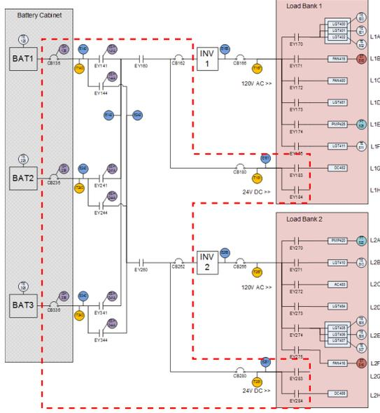
Fig. 2. Schematics of the diagnosis test bed ADAPT. The dark area to the left represents the three batteries and the two dark areas to the right are two load banks. Sensors in the circuit are marked as circles. The DC-circuit considered in this work is inside the dotted line.
