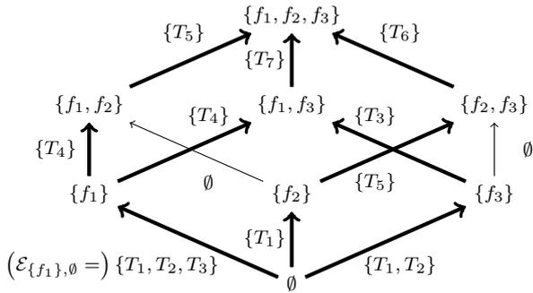
Fig. 4. A lattice set representation of all possible candidates for a system with three possible faults. The set at each arrow represents which test quantities that are able to reject  $d_j$  for  $d_i$  and fulfills a specified distinguishability criteria.
