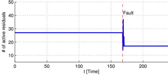
Fig. 8. The number of active residuals during a scenario where two sensors fail,  $f_{24}$  and  $f_{35}$ , occurs at 168 s. The total number of active residuals during the scenario is 54.
