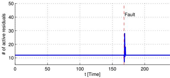
Fig. 9. The number of active residuals during a scenario where two sensors fail,  $f_{24}$  and  $f_{35}$ , occurs at 168 s. The required minimum distinguishability for each residual is lower compared to the result in Fig. 8 resulting in fewer active residuals during the scenario. The total number of active residuals during the scenario is 40.
