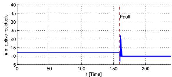
Fig. 6. The number of active residuals during a scenario where a relay gets stuck open,  $f_{10}$ , occurs at 159 s. The required minimum distinguishability for each residual is lower compared to the result in Fig. 5 resulting in fewer active residuals during the scenario. The total number of active residuals during the scenario is 41.
