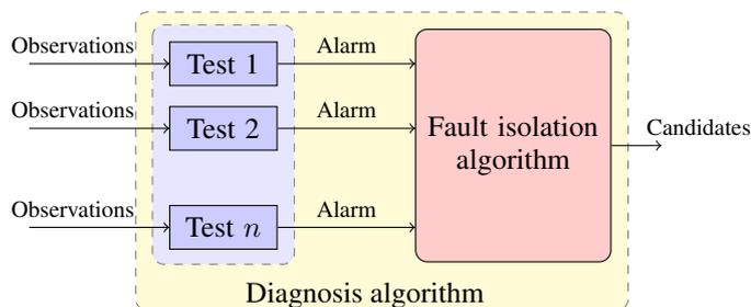
Fig. 1. A diagnosis algorithm consists of a set of test quantities and a fault isolation algorithm to compute (minimal) candidates.
