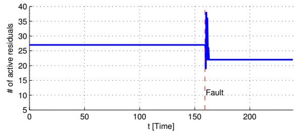
Fig. 5. The number of active residuals during a scenario where a relay gets stuck open,  $f_{10}$ , occurs at 159 s. The total number of active residuals during the scenario is 64.
