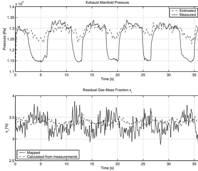
**Figure 7. Top: Exhaust pressure estimation without the use of the estimated residual gas mass. The estimate is within a few percent when the waste-gate is closed, that is when the exhaust pressure is approximately 130 kPa.**
