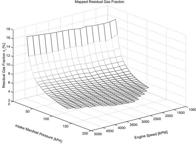
**Figure 4. Mapped residual gas fraction. The mass  $m_r$  is stored in the map used, but the residual gas fraction is shown since it is a more intuitive measure of residual gas.**
