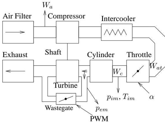
**Figure 1. Sensors and actuators on the engine. The only measured air mass flow is before the compressor,  $W_a$ .**
