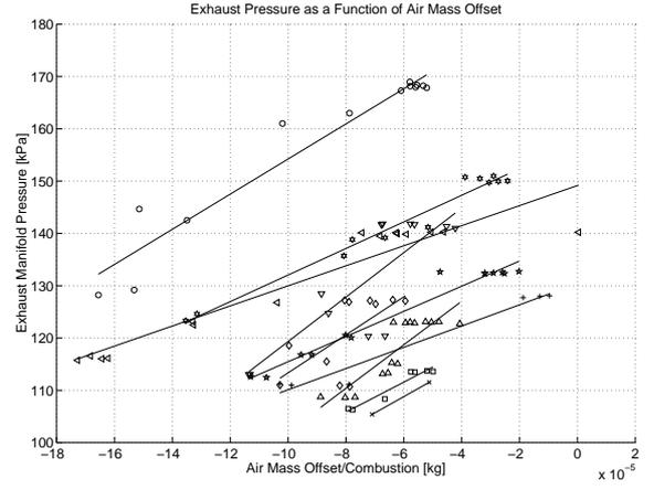
**Figure 3. Measured exhaust pressure with different wastegate settings when the engine was ran stationary. The exhaust pressure is linear as a function of the air mass offset  $m$ . The slope of the fitted first order function varies with engine operating point.**
