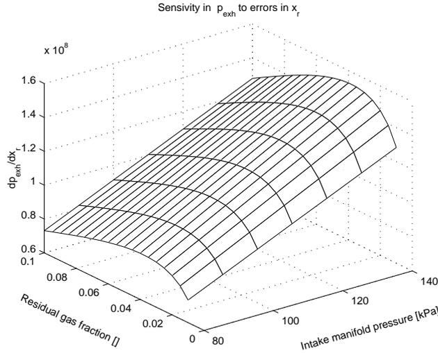
**Figure 9.**  $\frac{dp_{em}}{dx_r}$  for different points  $(p_{im}, x_r)$ . In the calculations  $c_v$ ,  $\eta_{vol}$ ,  $T_{im}$ ,  $\gamma$ , and  $T_r$  were fixed. The sensitivity to errors in  $x_r$  are linear in intake manifold pressure and almost constant for varying  $x_r$ .
