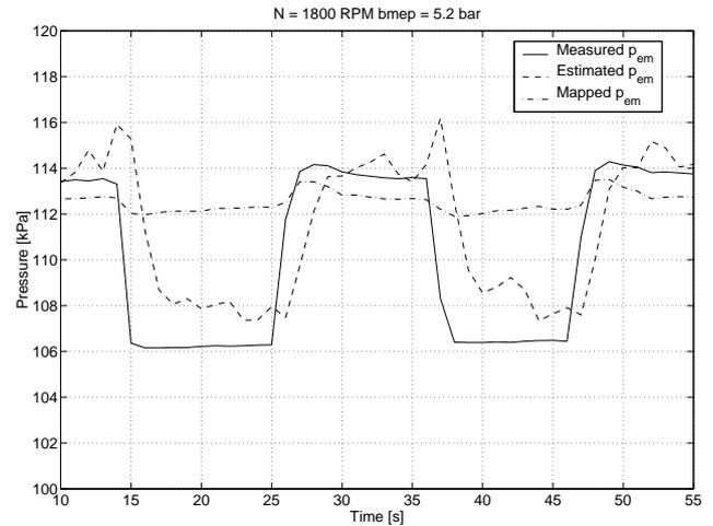
**Figure 5. Estimated exhaust manifold pressure during a wastegate step at low engine speed and load. Steady-state performance is within a few percent.**
