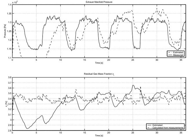
**Figure 8. Top: Estimated and measured exhaust pressure. It takes 10 seconds for the estimator to converge.**
