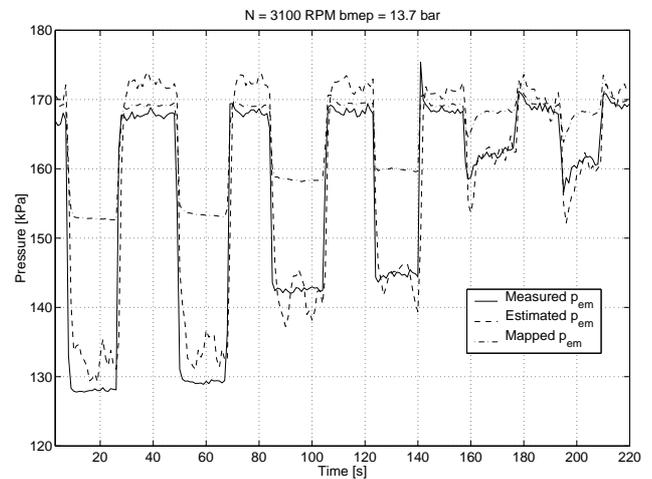
**Figure 6. Estimated exhaust manifold pressure during a wastegate step at medium engine speed and higher load.**
