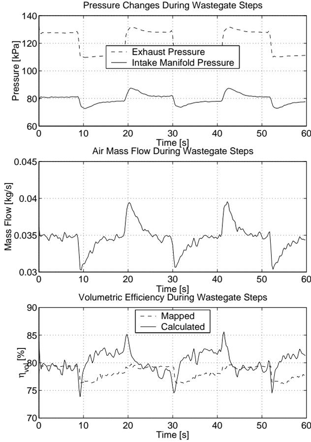
**Figure 2. Top:** When the wastegate is opened the exhaust pressure drops but the air mass flow is maintained constant by a controller (**center**). **Bottom:** At stationary conditions with closed wastegate (time 8, 28, and 50) the mapped volumetric efficiency agrees with the current volumetric efficiency  $\eta_{vol} = \frac{W_{af} RT_{im} n_r}{p_{im} V_d N}$ . When the wastegate is open (time 17, 30, and 60) the volumetric efficiency does not match the mapped value.
