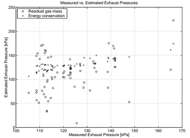
**Figure 10.** Stationary evaluation of the estimated exhaust pressure compared to measured pressure. Residual gas mass estimation results in a higher root square mean square error 4.7 kPa compared to 1.1 kPa for the energy conservation method.
