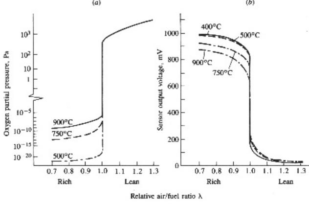
**Figure 4. Sensor characteristics as a function of air/fuel ratio, from [7]. Note the voltage jump at  $\lambda = 1.0$ .**
