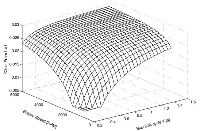
**Figure 9. Result using  $2K_p = \min(K_{I_u}, K_{I_d})\tau_{d1}$  and delayed switching. Here  $K_{I_d} = \frac{1}{3}K_{I_u}$ . The figure shows the maximum mean deviation from stoichiometric with these settings.**
