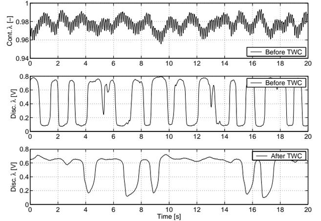
**Figure 3.** Measured air/fuel ratio of an engine running at idle. Top: Continuous  $\lambda$ , which oscillates with an amplitude of around 1%. In the measurement there is a sensor offset that drives the measured value from 1. Center: Measured  $\lambda$  in volts from an HEGO placed in front of the TWC. The oscillations are caused by the limit cycle of the controller. Bottom: Measured  $\lambda$  in volts from the HEGO behind the TWC. Note the voltage fluctuations.
