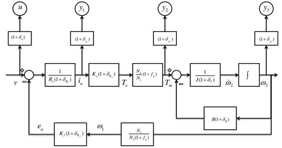
Figure 2: Block diagram model of DC motor.
