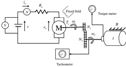
Figure 1: DC motor diagram.
