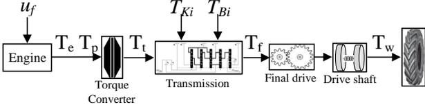
Fig. 2. Schematic view of the powertrain and driveline components with focus on transmission inputs and outputs.
