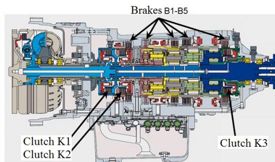
Fig. 1. Cutaway drawing of a nine speed automatic gearbox and torque converter.
