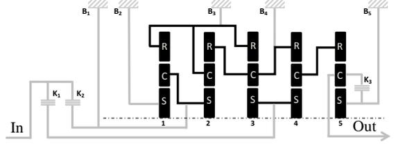
Fig. 3. Schematic view of a nine speed automatic gearbox and mechanical links between planetary gearsets components, Sun(S)-Carrier(C)-Ring(R), with respect to clutches and brakes.
