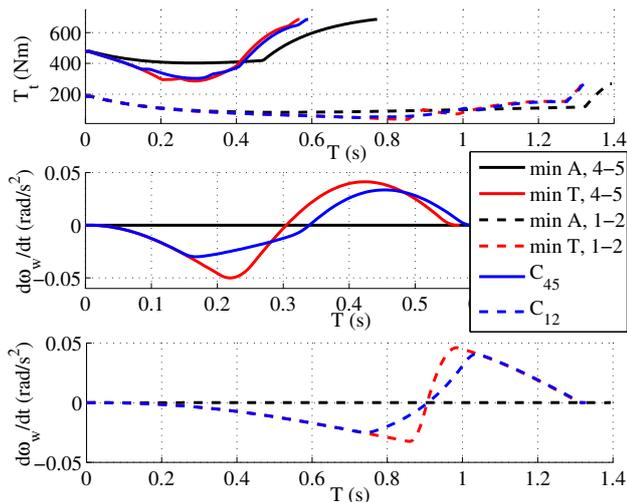
Fig. 11. Transmission input torque and vehicle acceleration/deceleration in min  $T$ , min  $A$  and  $C_{45}$  solutions of 1-2 and 4-5 up-shifts.
