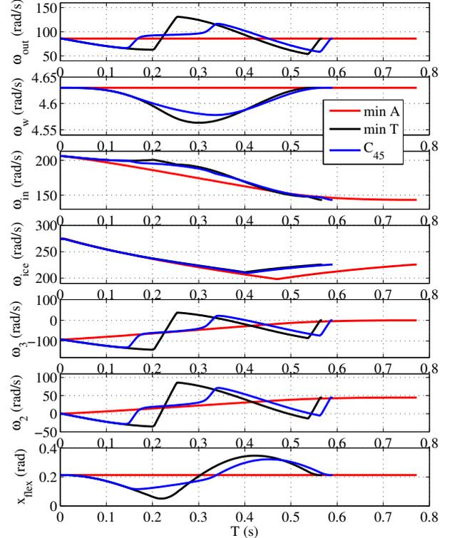
Fig. 10. Optimal state transients for min  $T$ , min  $A$  and  $C_{12}$  cases in a 4-5 up-shift where  $\omega_{out}=\omega_7$  and  $\omega_{in}=\omega_6$ .
