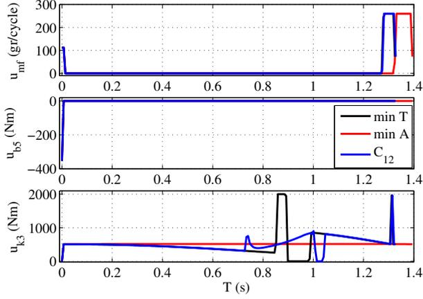
Fig. 7. Optimal control transients for min  $T$ , min  $A$  and  $C_{12}$  cases in a 1-2 up-shift.
