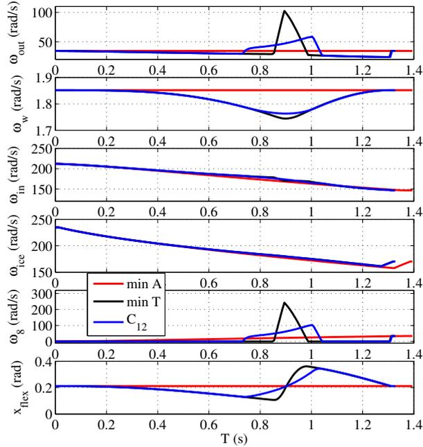
Fig. 8. Optimal state transients for min  $T$ , min  $A$  and  $C_{12}$  cases in a 1-2 up-shift where  $\omega_{out}=\omega_7$  and  $\omega_{in}=\omega_6$ .
