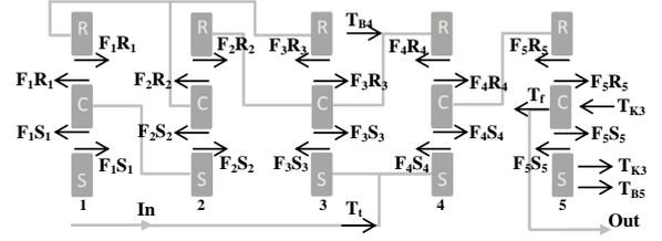
Fig. 5. Graphical representation of exerted torques on transmission components in a 1-2 gearshift.
