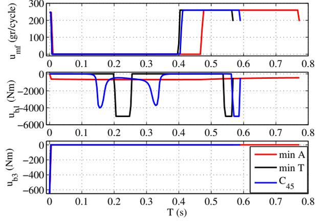
Fig. 9. Optimal control transients for min  $T$ , min  $A$  and  $C_{45}$  cases in a 4-5 up-shift .
