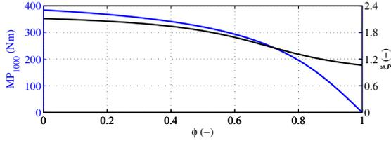
Fig. 4. Torque converter characteristic curves.
