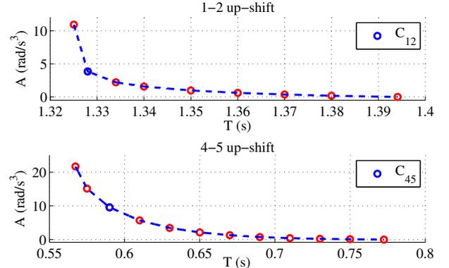
Fig. 6. The trade-off between time and jerk for 1-2 and 4-5 up-shifts. At  $C_{12,45}$  there is a compromise between the two objectives.
