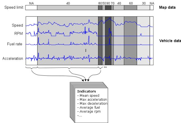
Fig. 1 Illustration of the segmentation process. The posted speed limit defines the segment boundaries. Based on available data in each segment, various performance indicators are calculated for subsequent statistical analysis.
