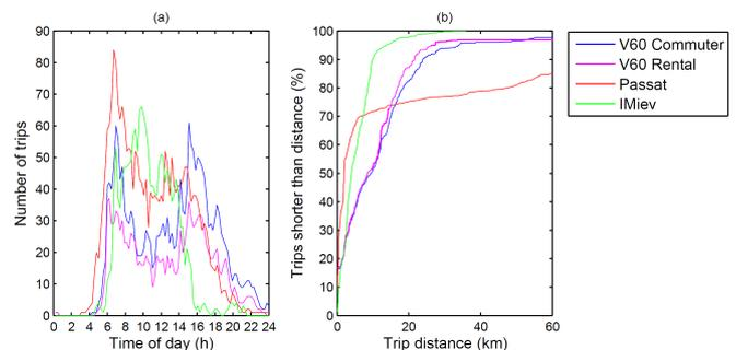
Fig. 2 Number of trips when the vehicles are in motion as a function of time of day (a), and the cumulative percentage of trips below a certain distance (b).
