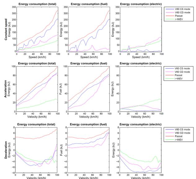
Fig. 4 Mean total (left), electric (middle) and fuel (right) energy consumption across all 5-second segments as a function of vehicle speed.
