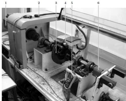
Figure 3: Brake dynamometer. The individual components are: 1. Dynamometer motor; 2. CAN cable; 3. Disc rotor; 4. EMB; 5. Thermometer connected to a thermocouple embedded in the brake pad; 6. Torque sensor.
