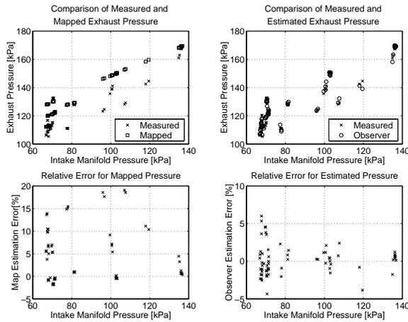
Fig. 4. *Left column:* When the static map of the exhaust pressure is used the exhaust pressure is overestimated as the wastegate is opened. *Right column:* The air mass offset information decreases the estimation error when the wastegate is opened.
