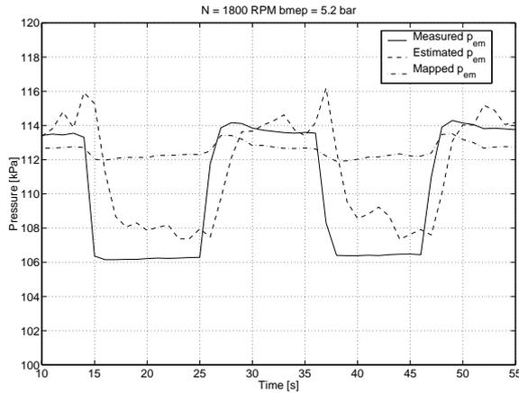
Fig. 5. Estimated exhaust manifold pressure during a wastegate step at low engine speed and load. Steady-state performance is within a few percent.
