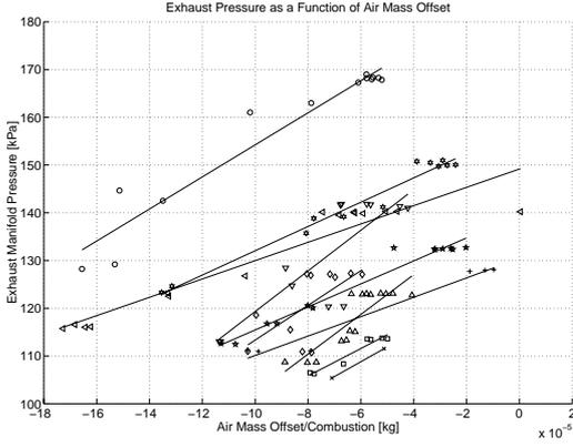
Fig. 3. Measured exhaust pressure with different wastegate settings when the engine was running at stationary conditions. The exhaust pressure is linear as a function of the air mass offset  $m$ . The slope of the fitted first order function varies slightly with engine operating point.
