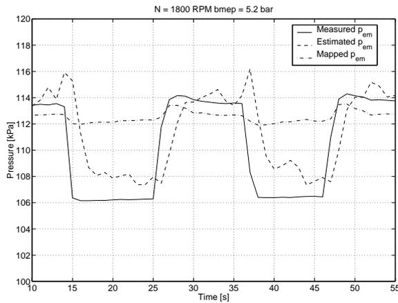
Fig. 5. Estimated exhaust manifold pressure during a wastegate step at low engine speed and load. Steady-state performance is within a few percent.
