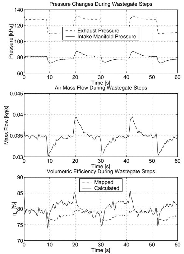
Fig. 2. *Top:* When the wastegate is opened the exhaust pressure drops but the air mass flow is maintained constant by a controller (*center*). *Bottom:* At stationary conditions with closed wastegate (time 8, 28, and 50) the mapped volumetric efficiency agrees with the current volumetric efficiency  $\eta_{vol} = \frac{W_{at} R_c T_{im} n_r}{p_{im} V_d N}$ . When the wastegate is open (time 17, 30, and 60) the volumetric efficiency does not match the mapped value.
