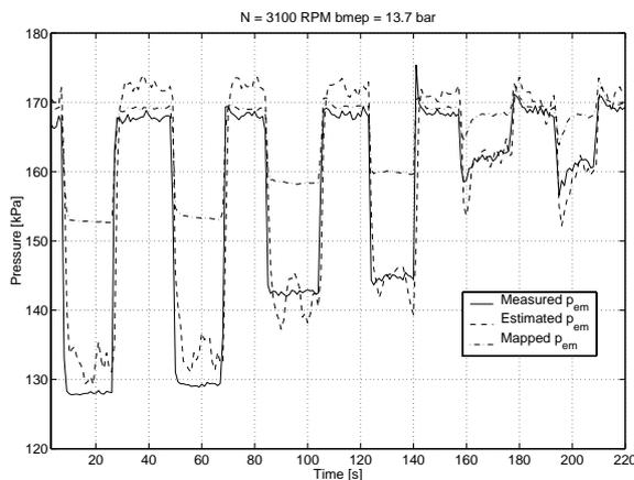
Fig. 6. Estimated exhaust manifold pressure during a series of wastegate steps at medium engine speed and higher load.
