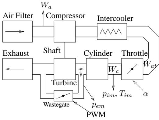
Fig. 1. Sensors and actuators on the engine. The only measured air mass flow is before the compressor,  $W_a$ .
