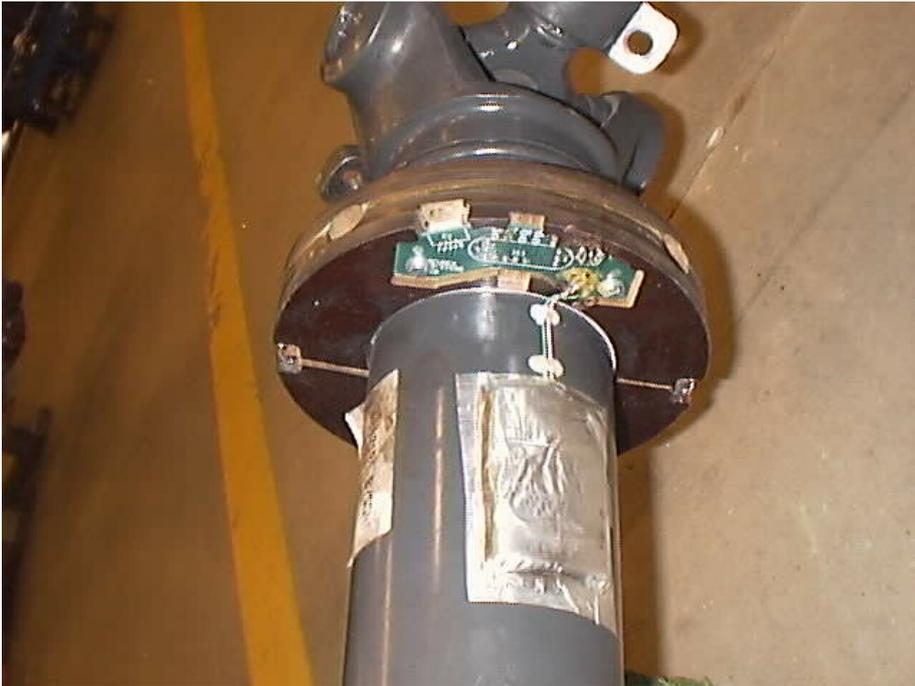
Figure 5.2: Strain gauges used to measure true torque on the propeller shaft.
