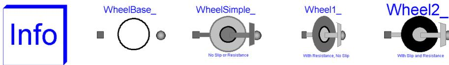
Figure 4.1: Wheel library, several exchangeable modules of different complexity.
