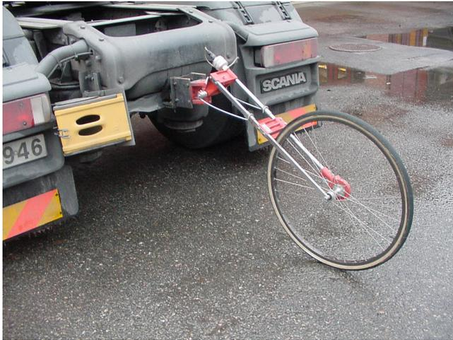
Figure 7.3: 5th wheel mounted after the truck to measure speed and distance.
