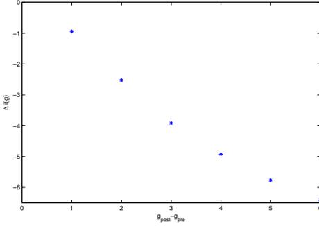
Figure 6: Dependence of difference in gear ratios,  $i(g_{post}) - i(g_{pre})$ , to number of steps between gears,  $g_{post} - g_{pre}$ , (where  $g_{pre} = 6$ ).
