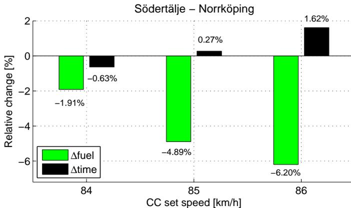
Figure 5: Trial run results on the road from Södertälje to Norrköping with varying cruise controller (CC) set speed.
