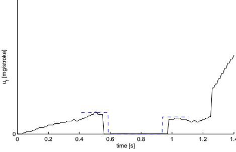
Figure 9: A gear shift from 10th to 11th gear in a  $-2\%$  downhill road gradient, model (dashed) and experimental test data (solid).
