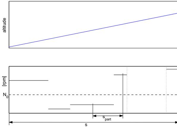
Figure 3: An optimal control which switches between many velocities is always replaceable to an optimal control that switches between no more than two speeds on a constant gradient.
