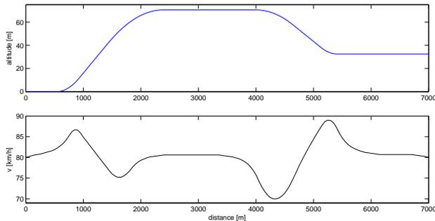
Figure 1.2: Optimal speed profile in significant hills.
