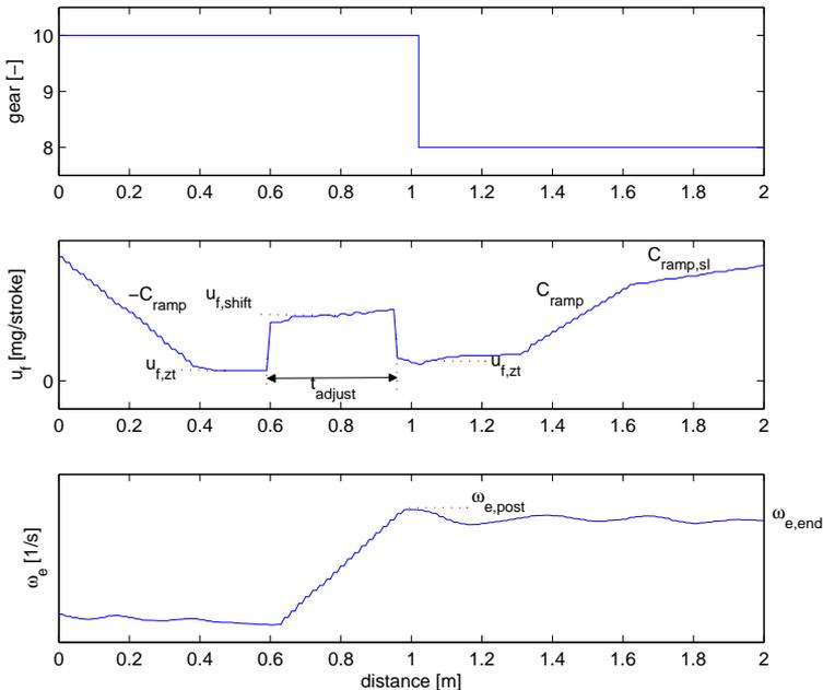
Figure 1: A gear shift from 10th to 8th gear of a 37 tonnes truck in a 6.5% uphill gradient.
