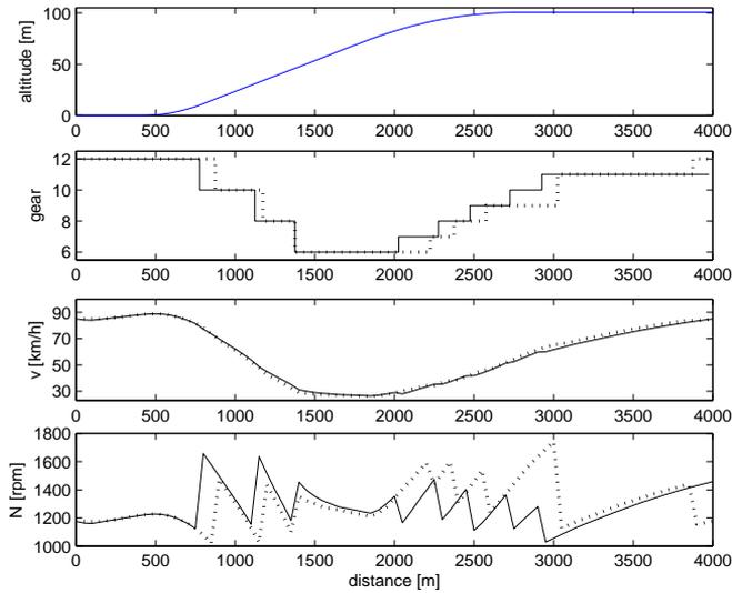
Figure 15: Truck of 60 tonnes: Optimal gear-shifting strategy (solid) reduces fuel consumption by 0.1% compared to a standard AMT (dotted) while keeping the same mean speed.
