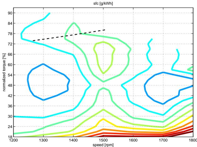
Figure 1: Fuel map showing sfc [g/kWh] of a combustion engine. The disadvantageous speed 1500 rpm requires a higher sfc than 1300 or 1700 rpm. The dashed line is the operation line of stationary speeds for a small uphill gradient.
