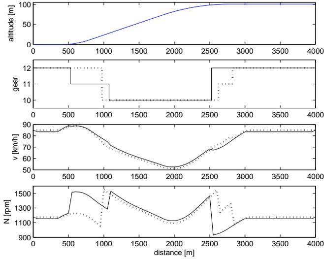
Figure 11: Truck of 30 tonnes: The  $\beta_{time}$ -case (solid) reduces fuel consumption by 0.1% compared to a standard AMT (dotted) while going 0.5% faster.
