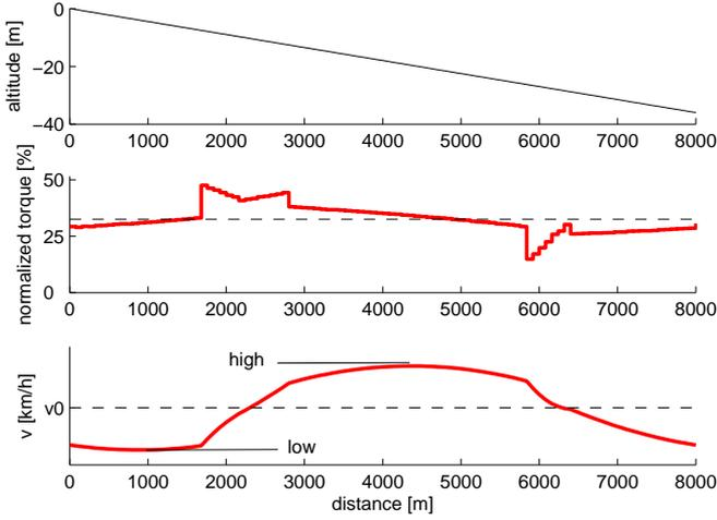
Figure 13: Solid - optimal control. Dashed - constant speed control.  $\Delta m_f = -1\%$  on a 8000 m road stretch.
