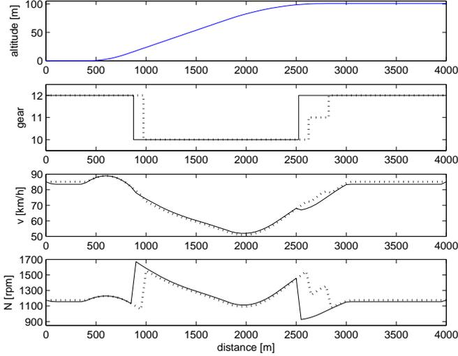
Figure 12: Truck of 30 tonnes: The  $\beta_{fuel}$ -case (solid) reduces fuel consumption by 0.4% compared to a standard AMT (dotted) while going 0.2% slower.
