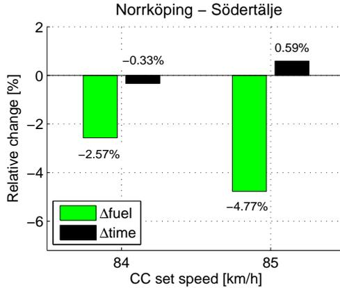
Figure 6: Trial run results on the road from Norrköping to Södertälje with varying cruise controller (CC) set speed.
