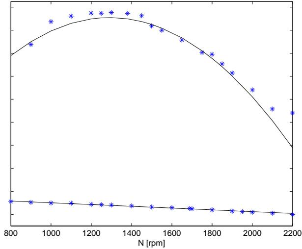
Figure 10: Maximum and minimum torque.
