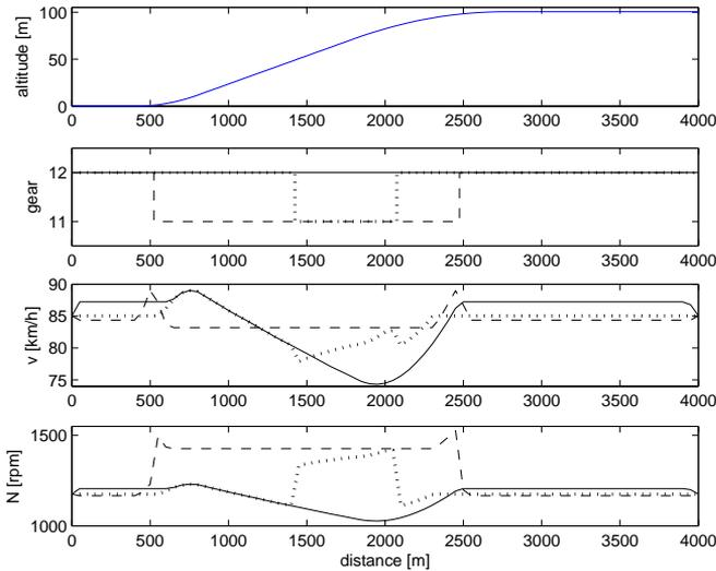
Figure 10: Truck of 17 tonnes: Optimal gear-shifting strategy (solid) reduces fuel consumption by 0.7% compared to a standard AMT (dotted) and by 2.2% compared to a manual gear-shifting strategy (dashed) while keeping the same mean speed.
