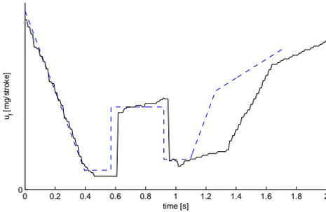
Figure 7: A gear shift from 10th to 8th gear in a 7% uphill road gradient, model (dashed) and experimental test data (solid).
