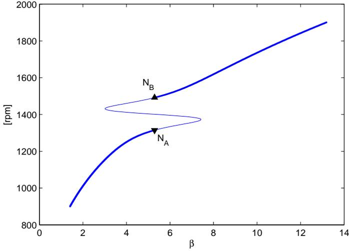
Figure 7: Stationary solutions,  $\hat{N}$ , where the global minimum,  $\hat{N}^*$ , is marked with fat lines, and the boundary velocities,  $N_A$  and  $N_B$ .
