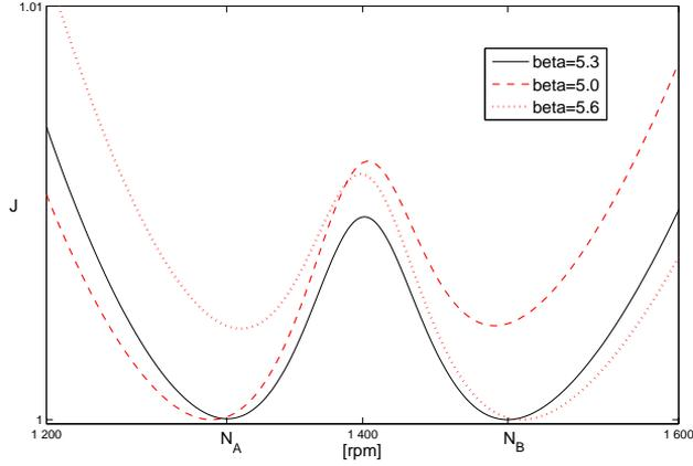
Figure 8: Objective function (26) for the studied constant road grade with different  $\beta$ .
