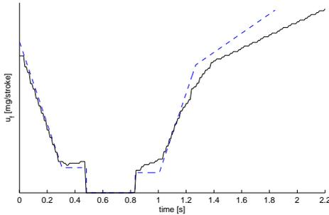
Figure 8: A gear shift from 10th to 11th gear in a 2% uphill road gradient, model (dashed) and experimental test data (solid).
