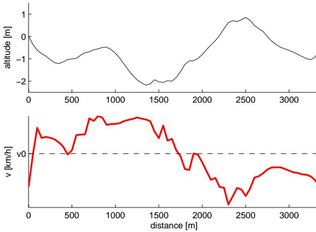
Figure 18: Solid - optimal control. Dashed - constant speed control ( $\Delta m_f = -1.1\%$ ).
