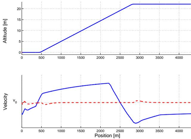
Figure 2: Upper plot: altitude profile. Lower plot: Solid line - optimal control, see (Hellström et al., 2006). Dashed line - cruise control with constant set speed,  $v_0$ .
