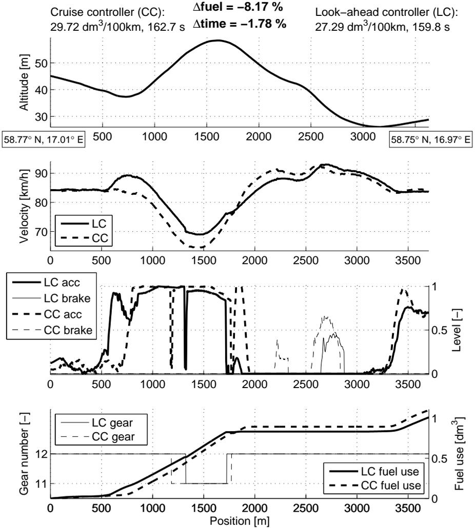
Figure 7: The Hället segment. The LC accelerates at 500 m prior to the uphill and slows down at 1750 m when the top is reached.
