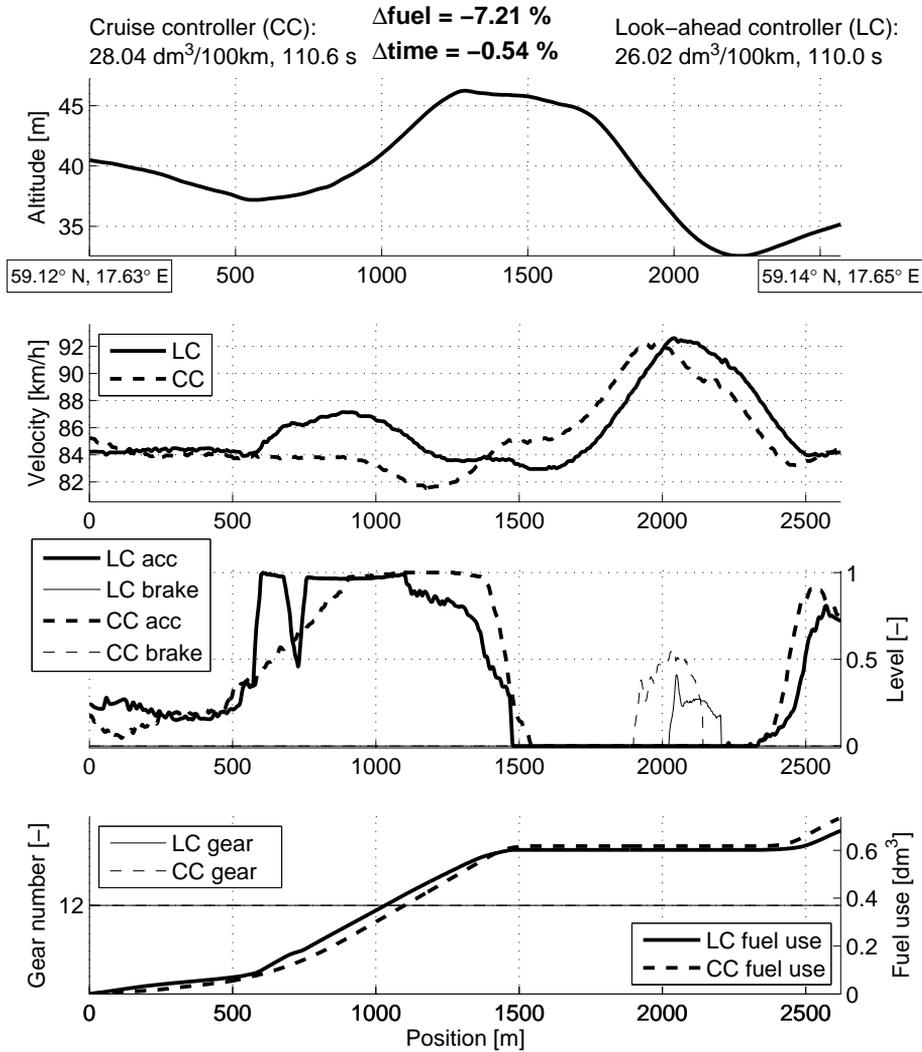
Figure 10: The Järna segment. The LC accelerates at 500 m and slows down at 1400 m thereby reducing the braking effort needed later on.
