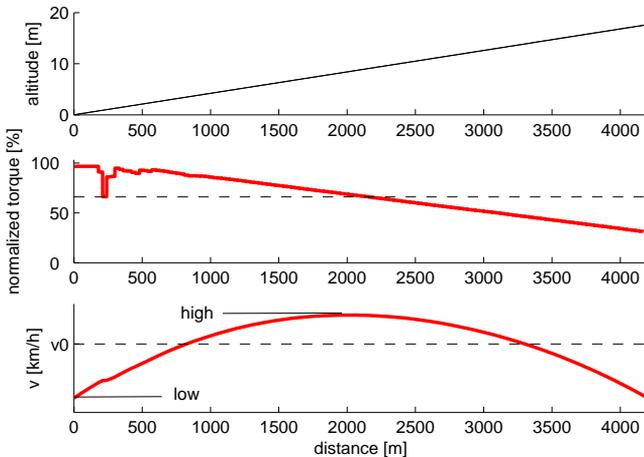
Figure 11: Solid - optimal control. Dashed - constant speed control.  $\Delta m_f = -2.4\%$  on a 4200 m road stretch.
