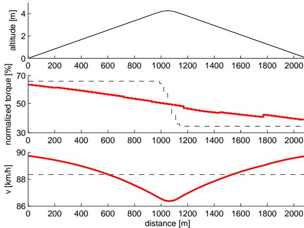
Figure 15: Solid - optimal control. Dashed - constant speed control.  $\Delta m_f = -1.6\%$  on a 2100 m road stretch.
