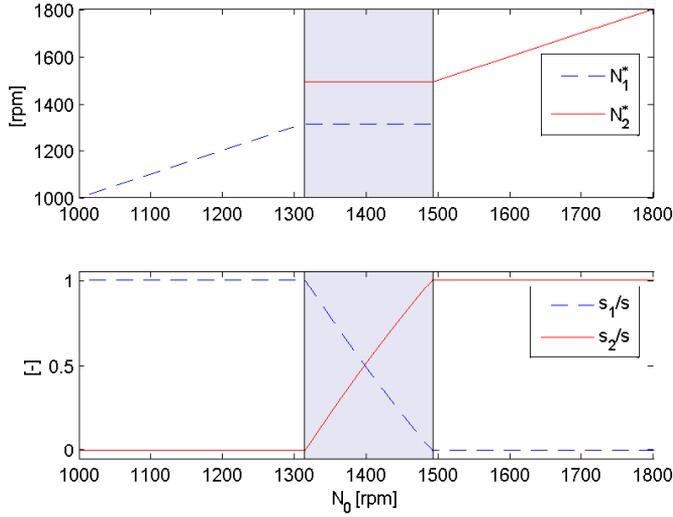
Figure 4: Optimal solution for varying  $N_0$  ( $N_{\text{sfc}_0}=1400$  rpm). The upper plot shows the optimal speeds, i.e. switch velocities in the switching zone (shaded area) and constant speed outside the switching zone. The lower plot shows the distances traveled with each speed.
