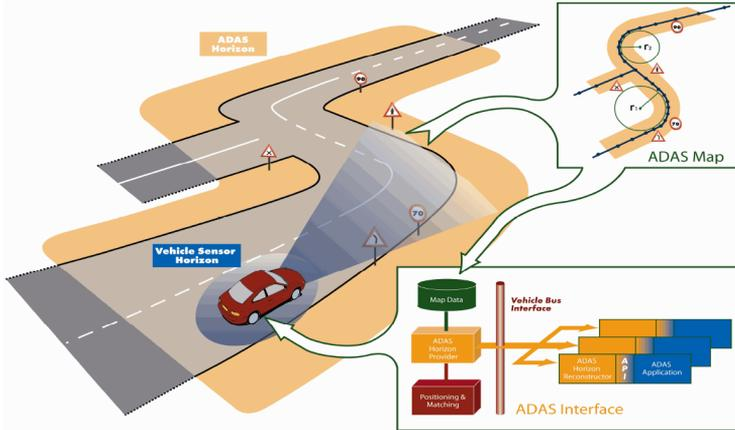
Figure 1.1: Look ahead horizon of a predicted future route with different attributes such as speed limits and road curvature. (Illustration courtesy of the PREVENT project).
