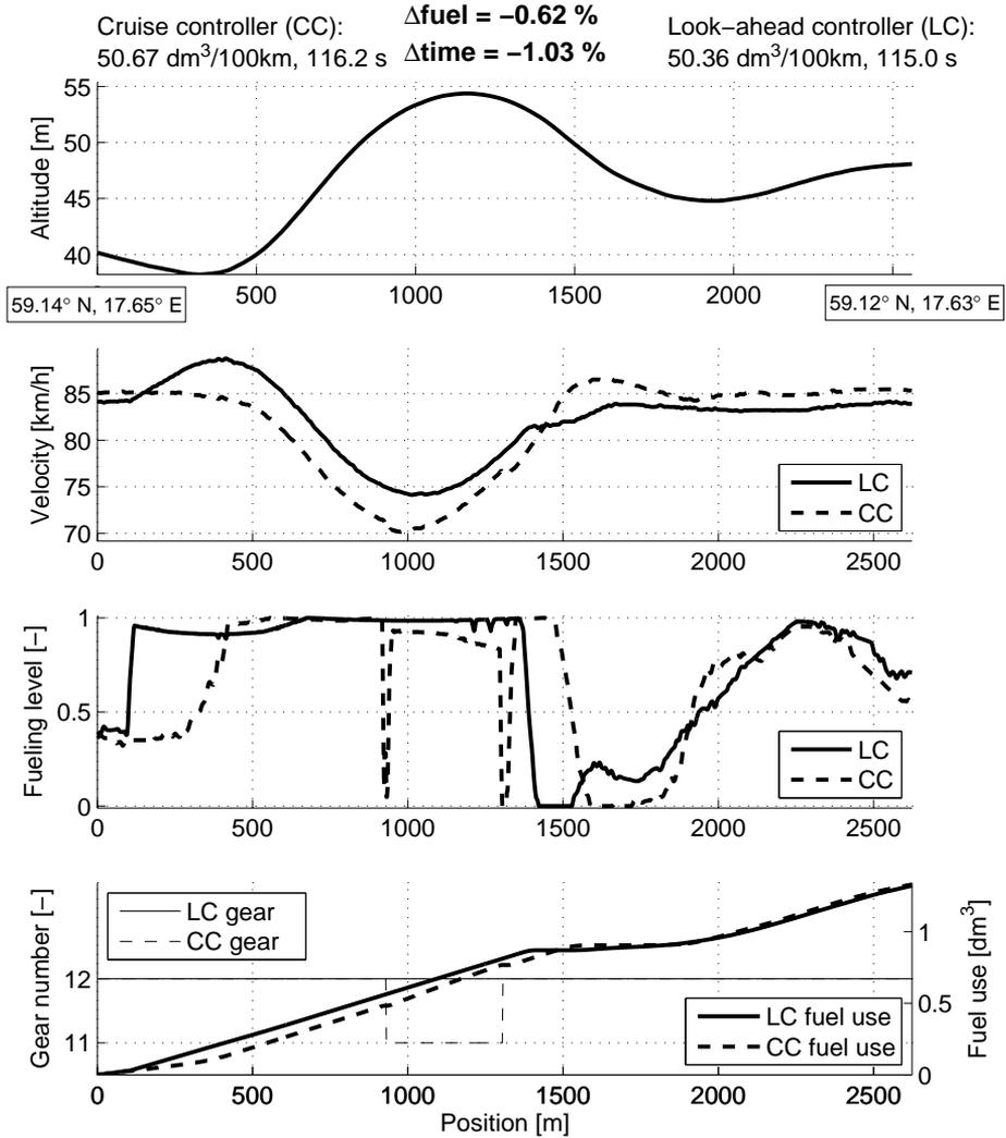
Figure 9: The Järna segment. The LC gains speed at 200 m prior to the uphill and avoids a gear shift. At 1400 m the LC slows down and the truck is let to accelerate in the downslope.
