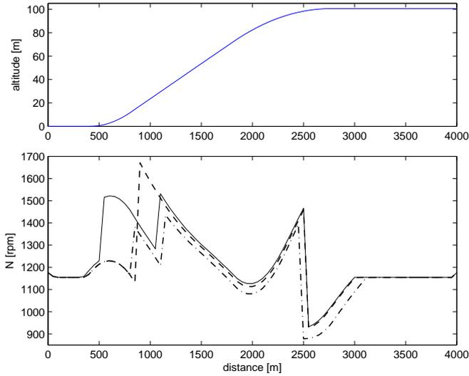
Figure 14: Engine speeds for  $\beta_{time}$ -case (solid),  $\beta_{fuel}$ -case (dashed) and  $igs$ -case (dotted-dashed).
