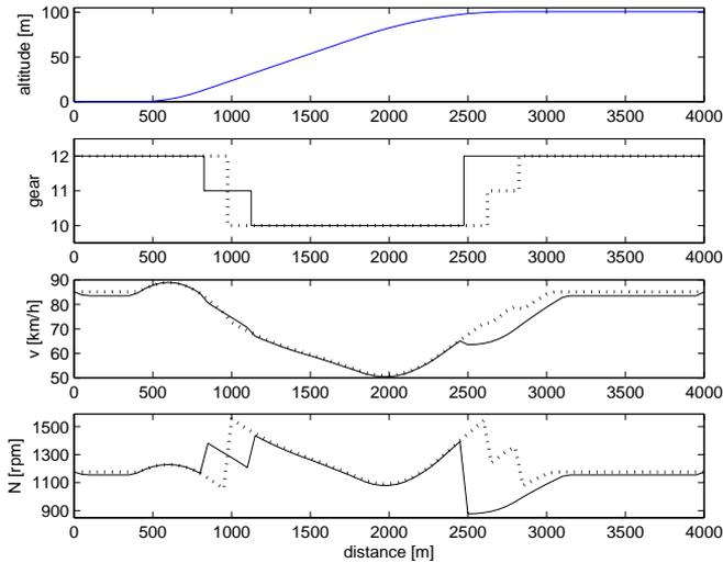
Figure 13: Truck of 30 tonnes: the *igs*-case (solid) reduces fuel consumption by 1.2% compared to a standard AMT (dotted) while going 2.2% slower.
