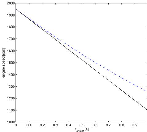
Figure 5: The model of a realistic engine deceleration as an affine function (solid) and engine speed as an exponential function solving (15) for  $T_{e,gas} = 0$ .
