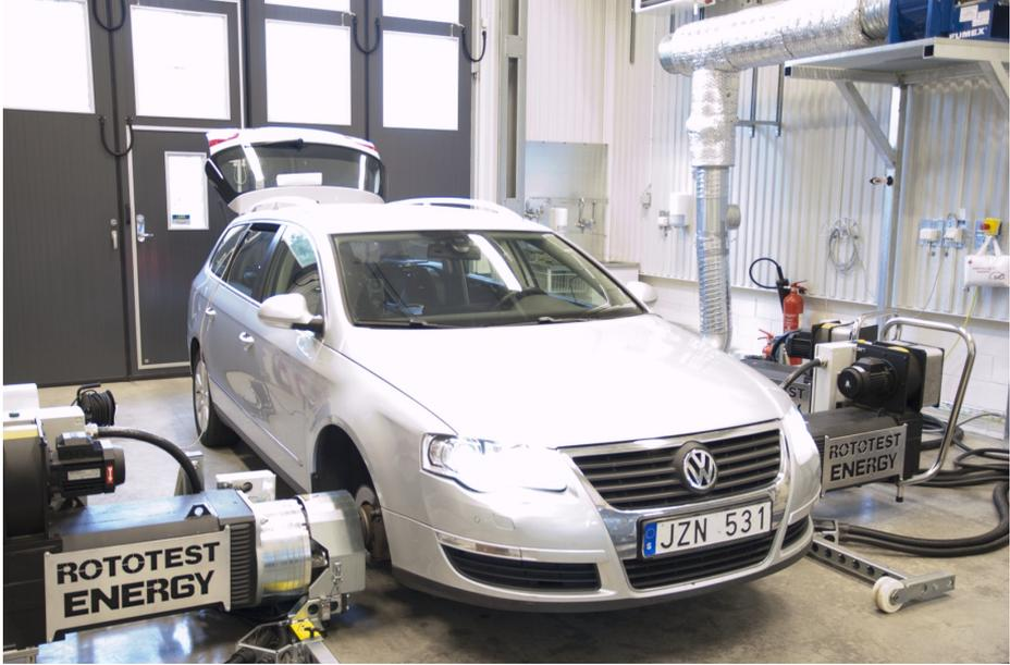
Figure 2: The Volkswagen Passat that is used in the experiment mounted in the chassis dynamometer of the vehicle propulsion laboratory.
