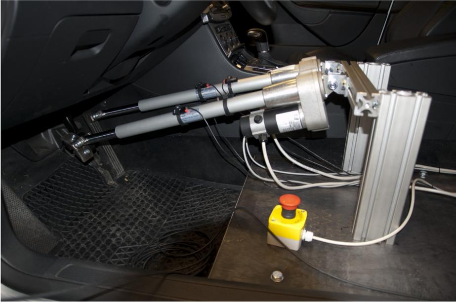
Figure 4: Pedal robot installed in the Volkswagen Passat test vehicle.
