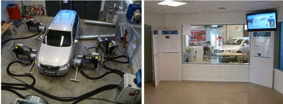
Figure 3: Left: View of the vehicle propulsion laboratory with four mobile dynamometers, head wind fan and exhaust ventilation. Right: View from the corridor.
