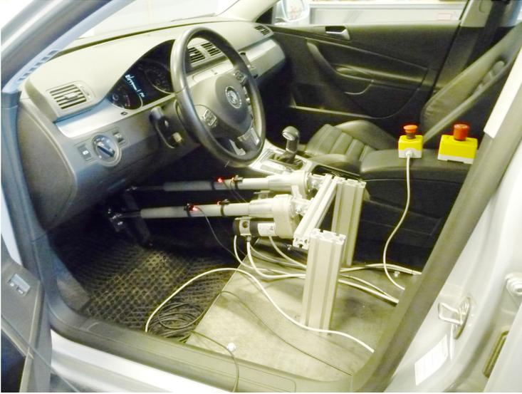
Figure 11: The pedal robot that was used to actuate the gas and brake pedal according to the input from the driver in the SIM-III simulator.
