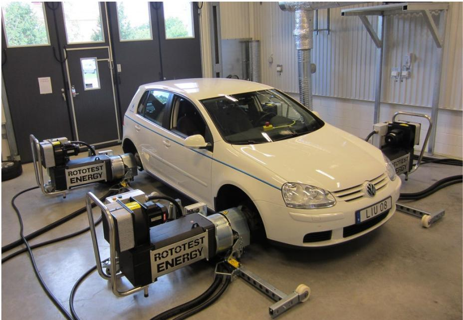
Figure 1: A glance of the new chassis dynamometer lab. A Golf V with a 1.4l multifuel engine has been mounted to the dynamometer units in a 4WD configuration.
