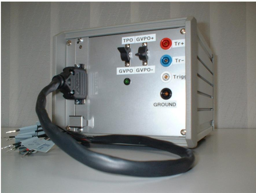
Figure 5.1. Construction of gate voltage pulsed operation. The front panel has switches to select pulse mode, temperature pulsed or gate voltage pulsed operation, and to select the sign (positive or negative potential) for the gate voltage pulsed operation mode. Temperature pulsed operation is a method to heat a sensor with controlled heat intervals. Further, the front panel has an output for trigger functions.
