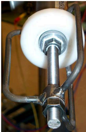
Figure 3.6: Picture of restriction position when doing EGR flow experiment, medium EGR.
