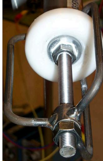
Figure 3.5: Picture of restriction position when doing EGR flow experiment, low EGR.
