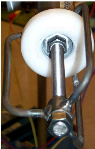
Figure 3.4: Picture of restriction position when doing EGR flow experiment, called minimum or no EGR.
