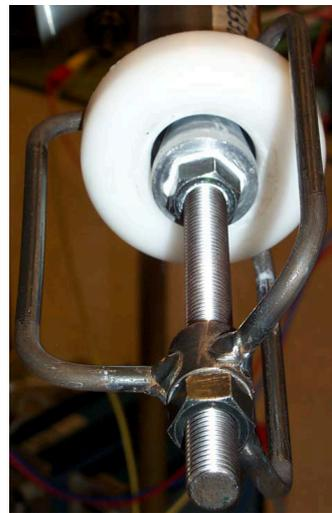
Figure 3.7: Picture of restriction position when doing EGR flow experiment, high EGR.
