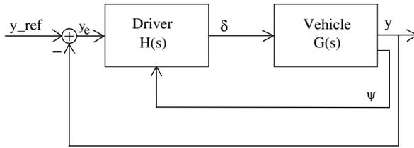
Figure 3.3: Basic structure of multi-input model
