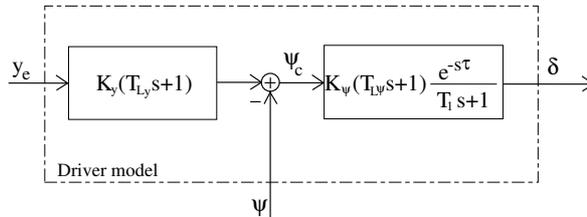
Figure 3.4: Multi-input driver model
