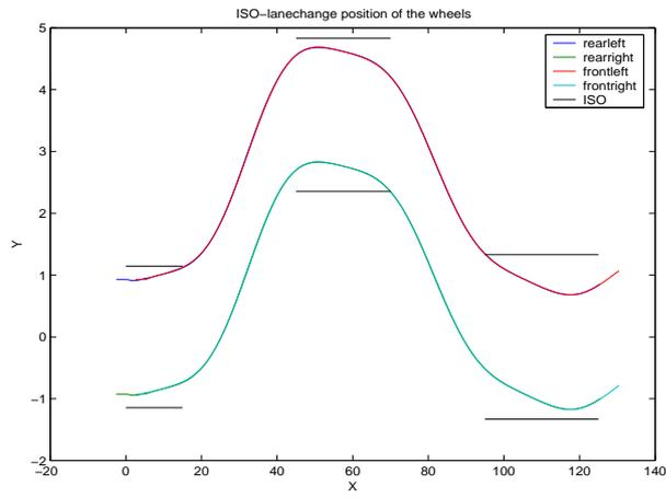
Figure 5.2: The wheel positions in a smoother ISO lane-change manoeuvre
