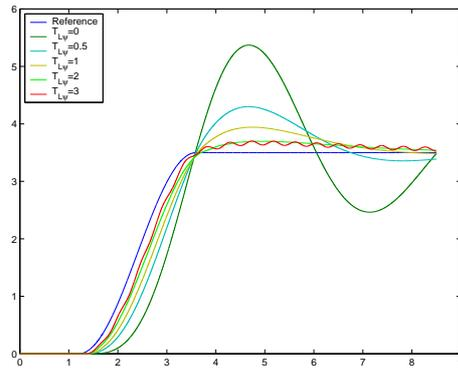
Figure 3.8: Influence of driver lead time,  $T_{L\psi}$
