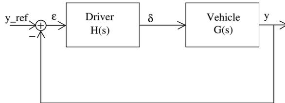
Figure 3.1: Basic structure of compensation tracking model
