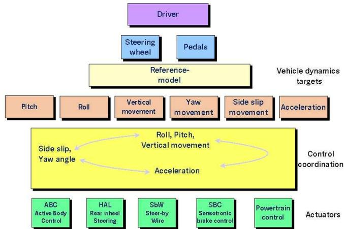
Figure 1.3: Overview of the VFD system in Technoshuttle.
