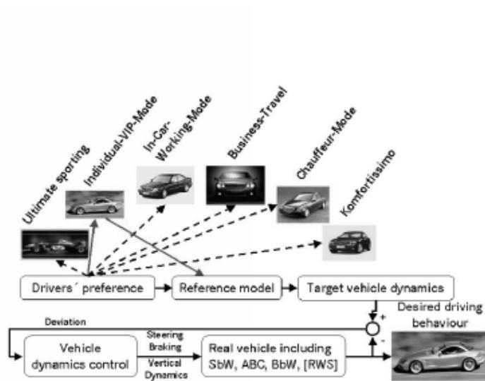
Figure 1.2: Overview of the integrated chassis control.
