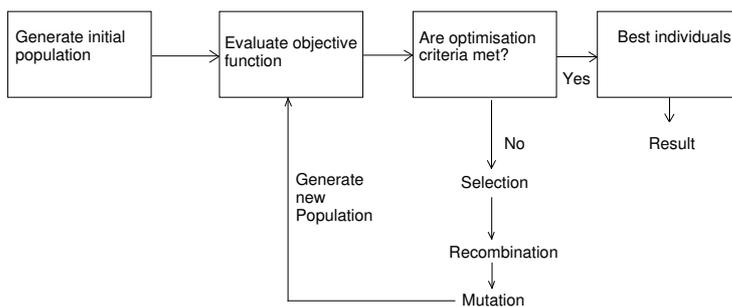
Figure 4.1: Evolutionary Algorithm Structure
