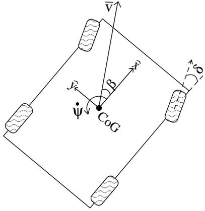
Figure 2.1: The Center of Gravity co-ordinate system.
