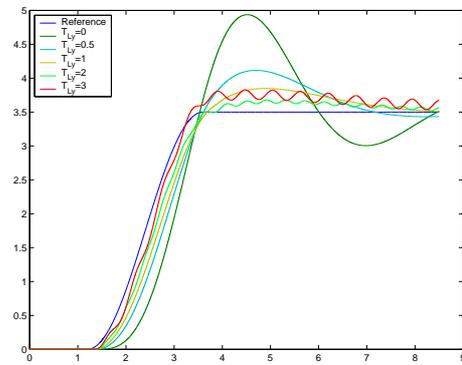
Figure 3.7: Influence of driver lead time,  $T_{Ly}$
