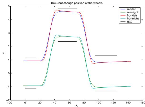
Figure 5.1: The wheels of the vehicle as the driver takes a middle path in the ISO lane-change
