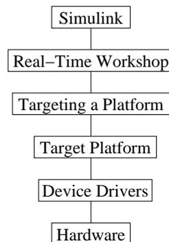
Figure 3.1: A way of viewing the system components and their relations to each other. Target platforms will be RTLinux or RTAI. The targeting of a platform is the conforming of the automatically Real-Time Workshop generated code to a specific platform.
