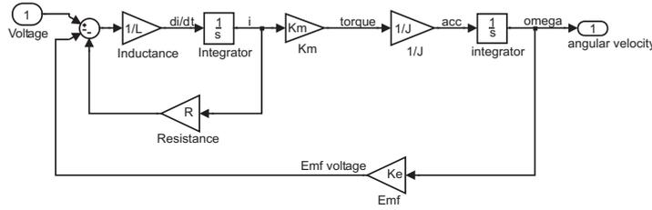
Figure 4.3: A Simulink model of a DC motor.
