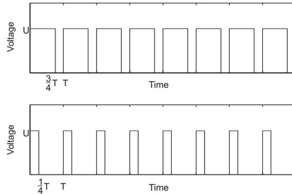
Figure 3.2: PWM signals with 75% and 25% duty cycle respectively.
