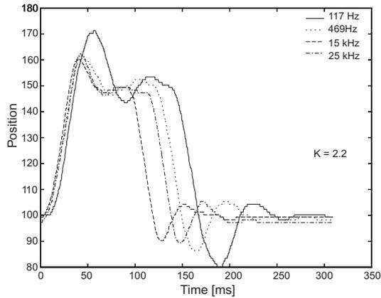
Figure 6.3: Comparison between four different PWM frequencies. Both the low and the high frequencies have problems.
