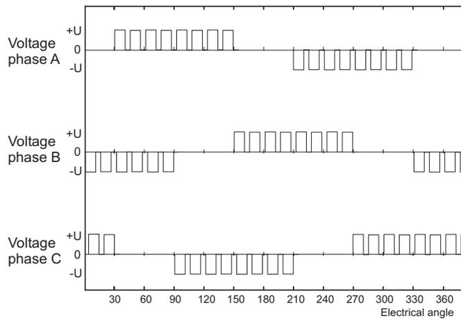
Figure 3.8: Voltages for each phase from the bridge gate driver.
