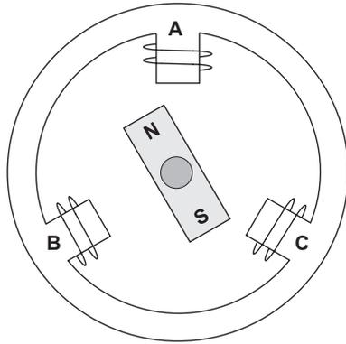
Figure 3.1: A three-phase BLDC motor.
