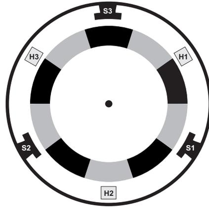
Figure 3.9: The MMT motor with five polepairs.
