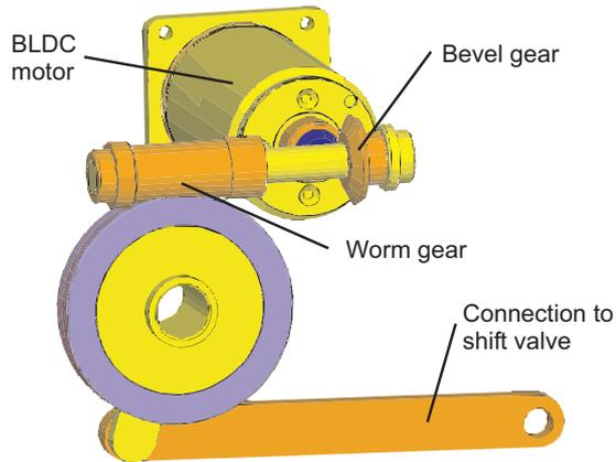
Figure 2.2: Actuator: DC motor and a gear reduction of 1:200.
