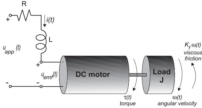
Figure 4.2: A simple model of a DC motor.
