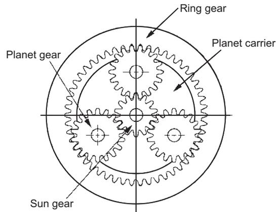
Figure 2.1: A planetary gear system.
