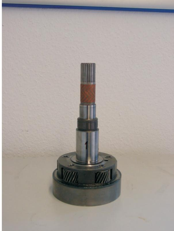
Figure 2.4: Gear Set from the 45RFE Transmission
