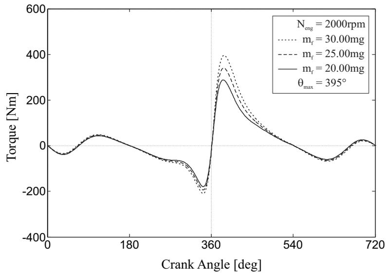
Figure 4.3: The simulated individual cylinder torque for  $N_{eng} = 2000\text{rpm}$  and different injected fuel quantities
