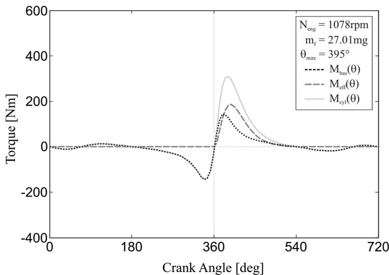
Figure 4.1: The simulated torque for one cylinder
