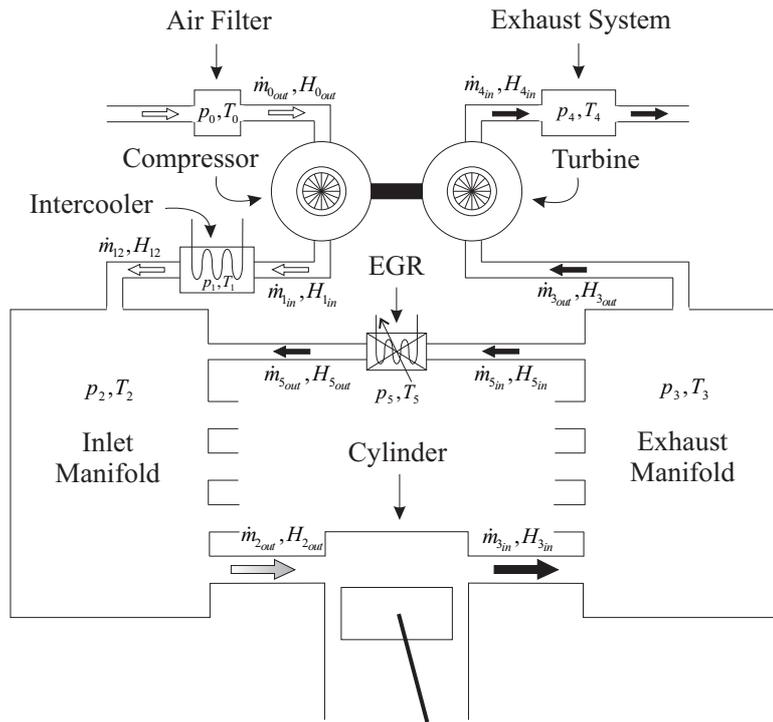
Figure 2.1: The structure of a basic diesel engine
