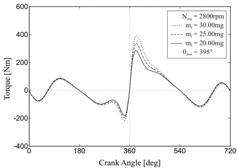
Figure 4.4: The simulated individual cylinder torque for  $N_{eng} = 2800\text{rpm}$  and different injected fuel quantities
