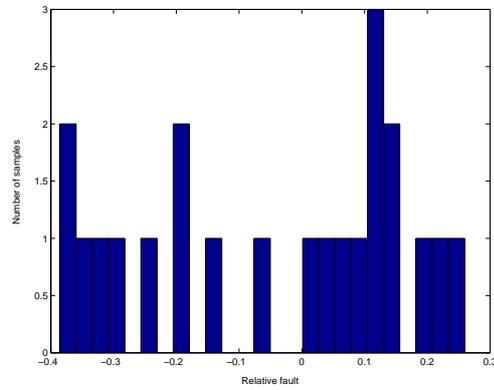
Figure 5.2: Histogram of the relative errors for the polynomial model.
