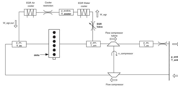
Figure 3.7: Extended model with two stage restriction EGR model.
