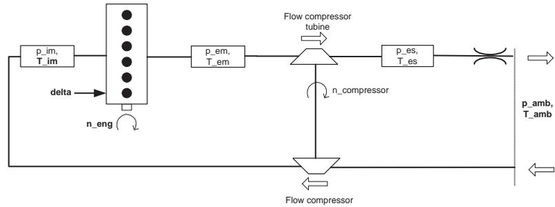
Figure 3.1: Schematic illustration of the existing model, input signals are bold.
