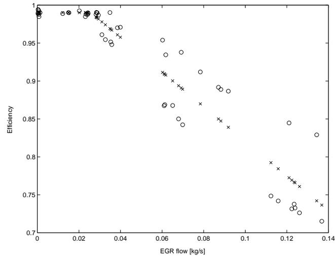
Figure 4.5: Measured cooler efficiency (o) and fitted model data (x).
