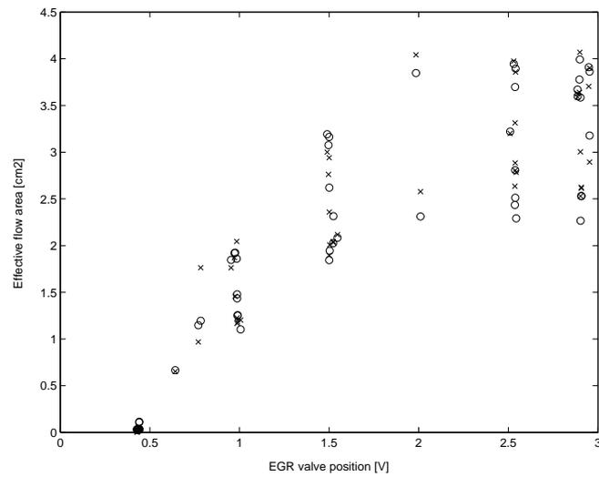
Figure 4.2: Measured effective area (o) and fitted model data (x), black-box model.
