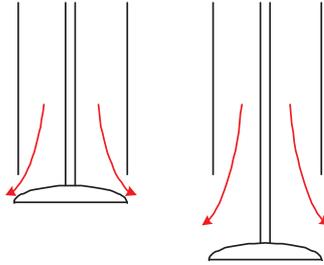
Figure 3.4: Illustrating the linear and evening-out phase of the effective flow area.
