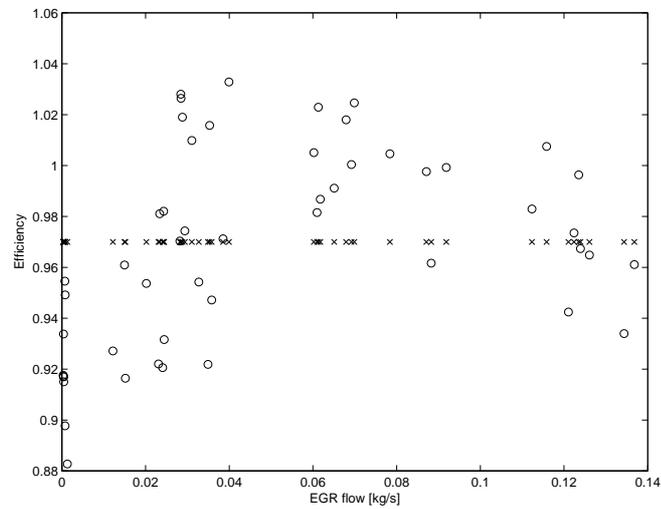
Figure 4.6: Measured cooler efficiency (o) and fitted model data (x).
