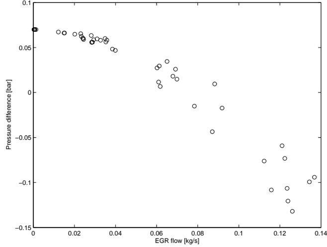
Figure 4.3: Pressure difference vs. EGR flow.
