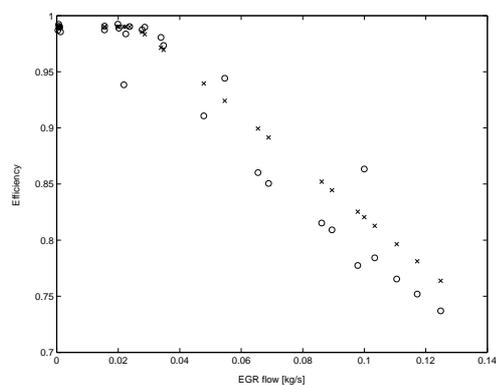
Figure 5.7: Measured efficiency (o) and modelled efficiency (x) for the water cooler.
