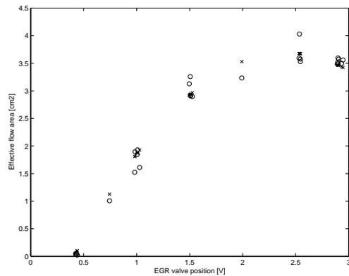
Figure 5.5: Measured effective area (o) and modelled effective area (x) for the two stage model
