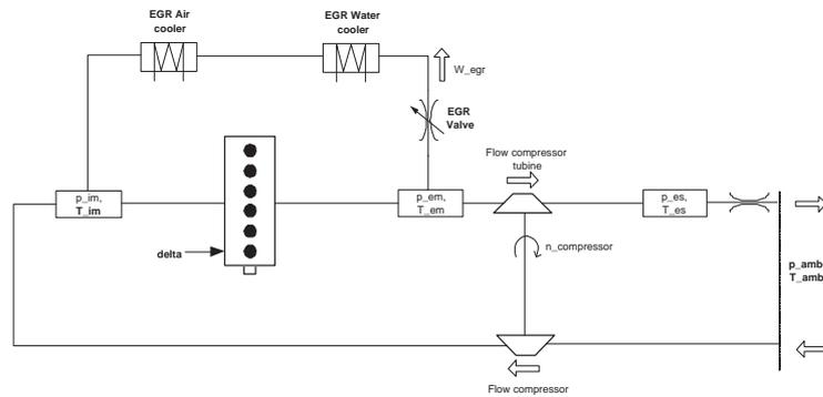
Figure 3.6: Extended model with single restriction EGR model.
