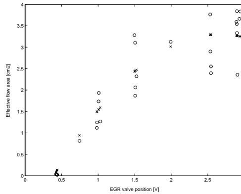
Figure 5.1: Measured effective area (o) and modelled effective area (x) for the single restriction polynomial model
