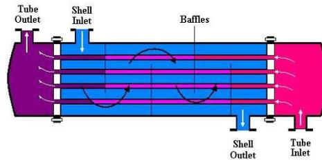
Figure 3.5: Shell and tube heat exchanger.
