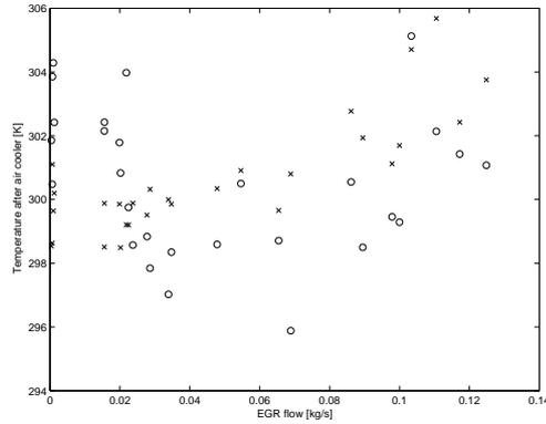
Figure 5.10: Measured temperature after the air cooler (o) and modelled temperature (x).
