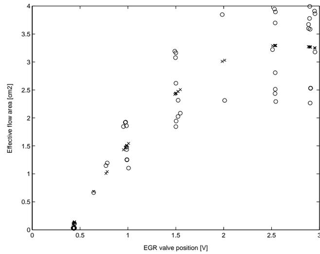
Figure 4.1: Measured effective area (o) and fitted model data (x), polynomial model.
