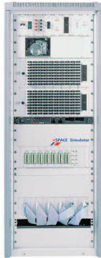
Figure 5.1: dSPACE HiL simulator [24]
