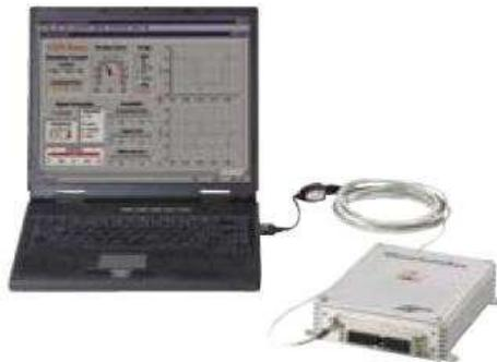
Figure 5.2: A laptop connected to the MicroAutoBox.
