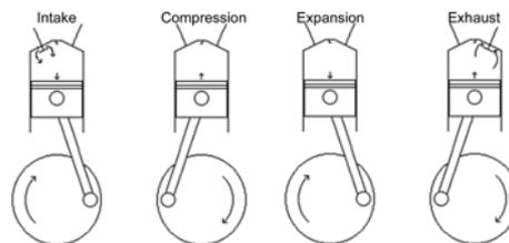
**Figure 2.1.** The four stages, or strokes, of the SI engine operation. Ignition occurs near the end of the compression stroke.
