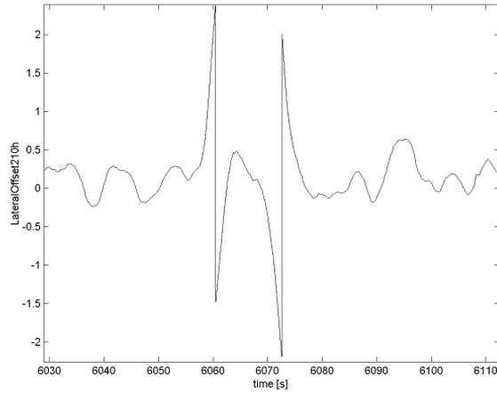
Figure 3.1: Lateral offset signal from the LDS. Typical signal characteristics when overtaking. Lane change to the left are followed by lane change to the right. [Offset in meters]
