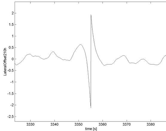
Figure 2.2: Lateral offset signal from the LDS. Typical lane change to the right. [Offset in meters]
