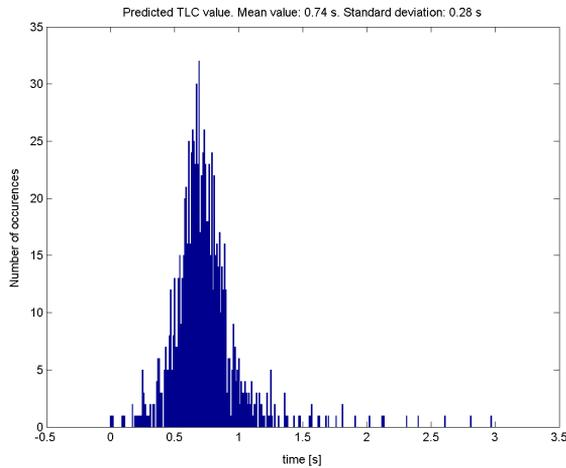
Figure 8.3: TLC predicted by the TLC system. Real TLC is 0.6 seconds. [Cases where TLC prediction is 3 seconds, i.e. cases where predicted TLC is undefined, are not shown. They are 4% of the cases]
