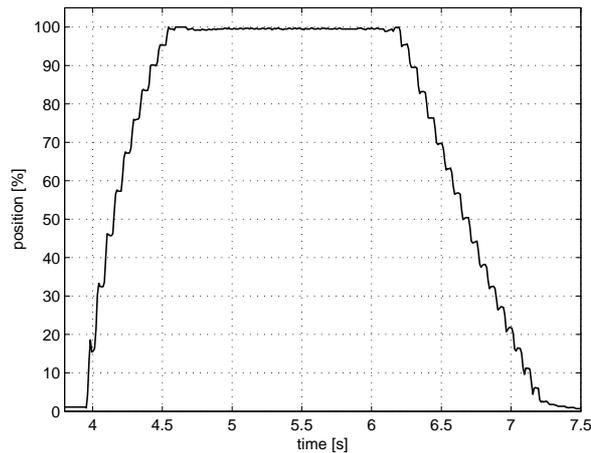
**Figure 5.7.** Different measured lengths in movement when increasing the piston position, dependent on start position. Constant length when decreasing it.
