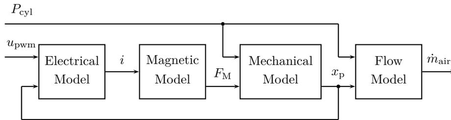
**Figure 2.4.** Block diagram of the valve.
