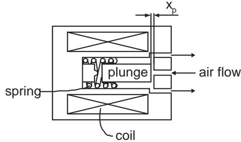
**Figure 2.2.** Sketch of the On/Off valve.
