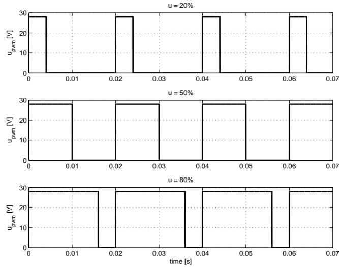
**Figure 2.3.** Simulated PWM signals with period time  $T = 20$  ms where  $u_{\text{pwm}} = 28$  V represents high and  $u_{\text{pwm}} = 0$  V represents low. From top to bottom:  $u = 20\%$ ,  $u = 50\%$  and  $u = 80\%$ .
