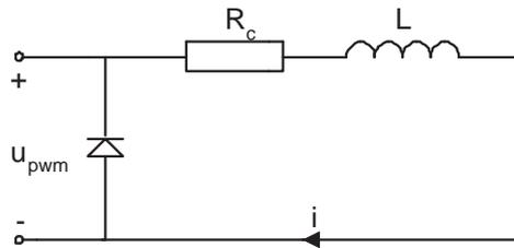
**Figure 5.9.** Schematic figure of the electrical circuit with a free wheel diode connected to the ECU's output circuit.
