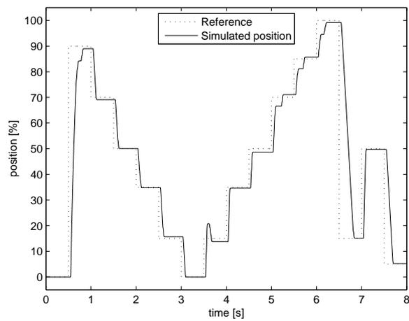
Figure 6.4. The pneumatic system simulated with a PID-controller.
