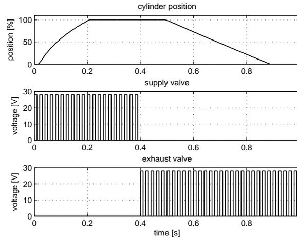
**Figure 5.6.** Measured piston position when given a constant input signal of 50% first to the supply valve, then to the exhaust valve, showing that the system is integrating.
