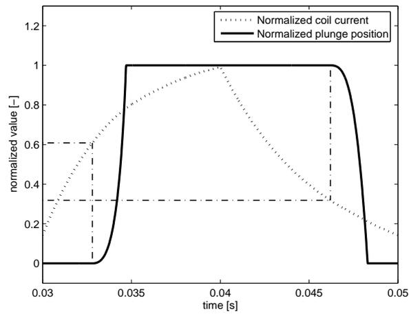
**Figure 5.2.** Simulation of the current through the coil and the plunge movement, showing at which current levels the plunge starts to move.
