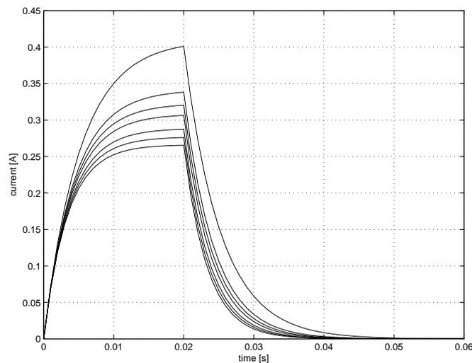
**Figure 5.3.** Simulated current in the electric circuit at different temperatures. From top to bottom:  $0^\circ\text{C}$ ,  $20^\circ\text{C}$ ,  $40^\circ\text{C}$ ,  $60^\circ\text{C}$ ,  $80^\circ\text{C}$ ,  $100^\circ\text{C}$  and  $120^\circ\text{C}$ .
