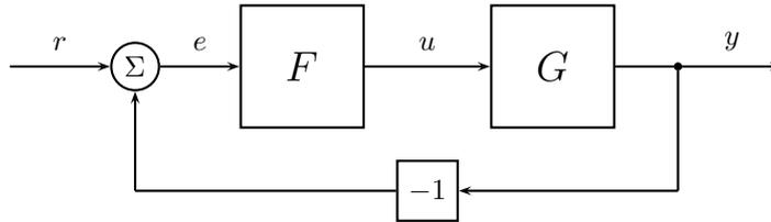
**Figure 6.1.** The structure of a basic feedback control loop.
