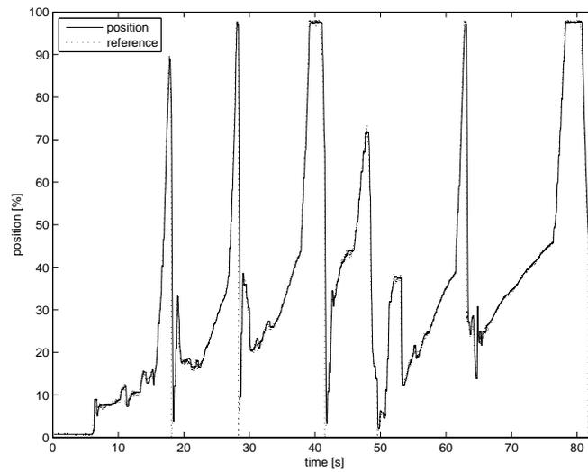
**Figure 6.17.** Reference for the piston position from a common driving case and measured piston position in a test bench.
