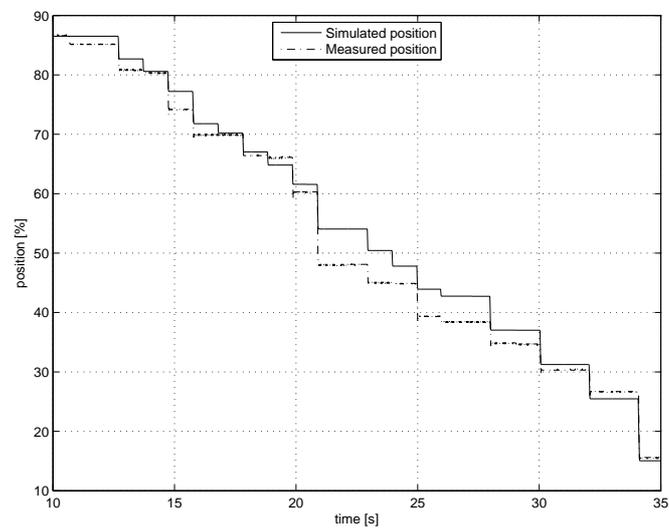
**Figure 3.4.** Simulated and measured position for the static calibration data for the exhaust valve.
