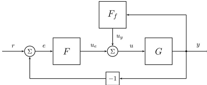
**Figure 6.16.** The structure of the controller implemented in the test bench.
