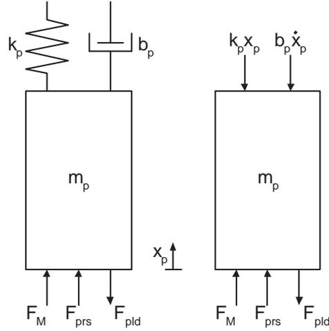
**Figure 2.9.** Sketch and free body diagram of the plunger.
