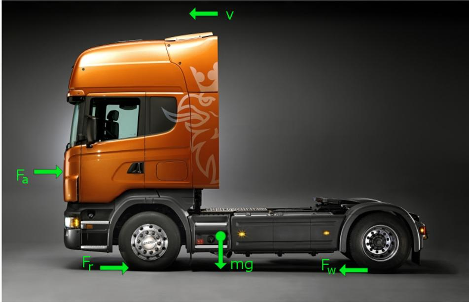
Figure 2.6: The forces acting on the vehicle.
