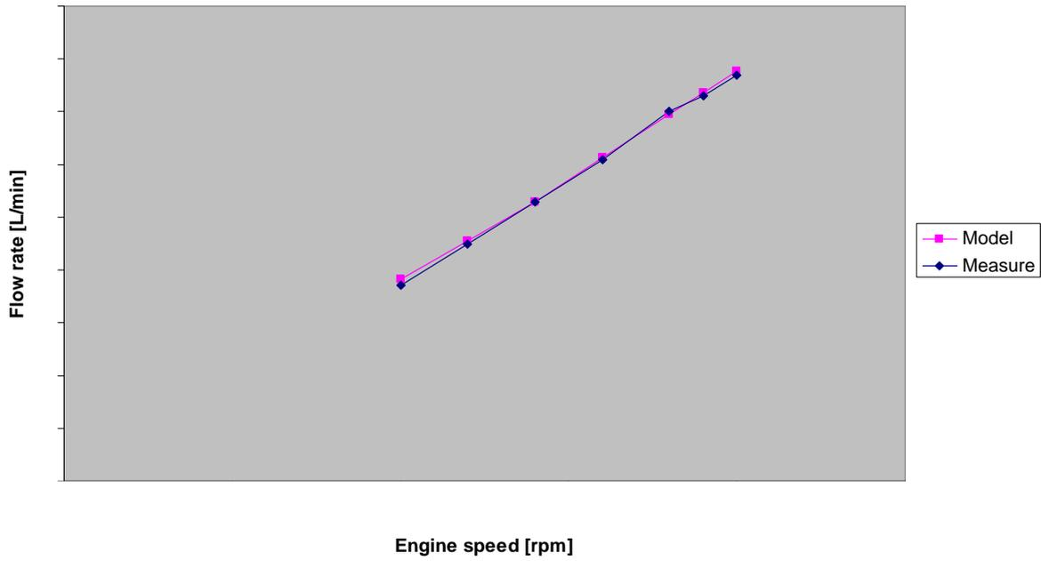
Figure 48. Flow through urea heater, Test 15.
