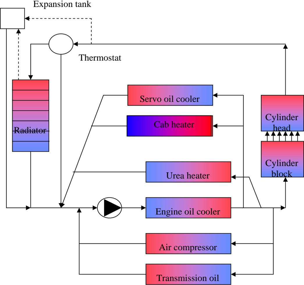
Figure 2. The cooling system.
