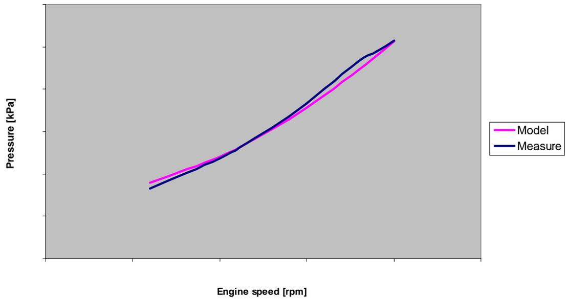
Figure 61. Pressure after coolant pump, Test 11.
