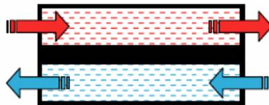
Figure 12. Counter flow heat exchanger.
