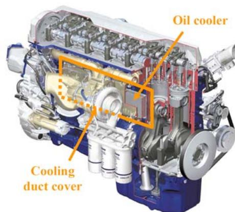
Figure 35. Oil cooling position.
