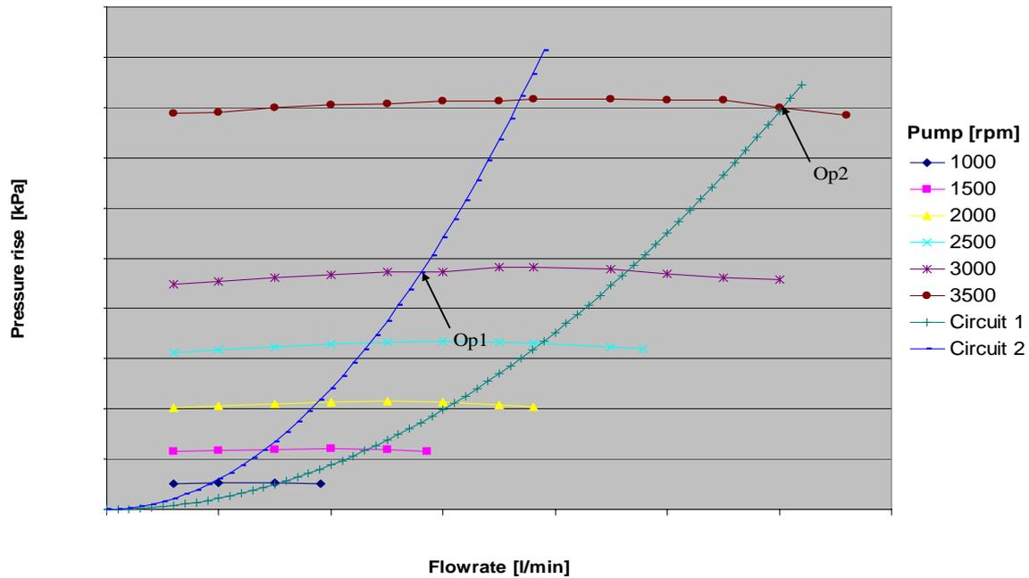
Figure 20. Coolant pump characteristic curve with system curves.
