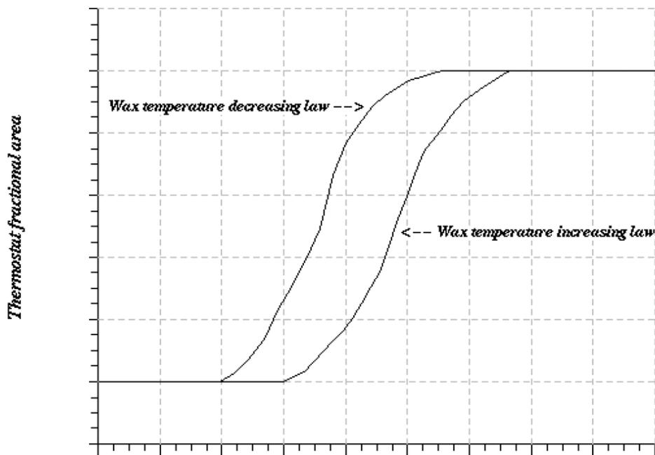
Figure 22. Characteristics curves for the thermostat.
