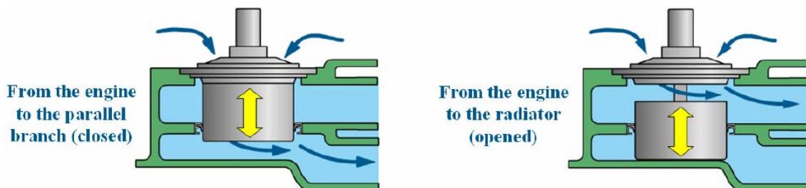
Figure 23. Closed and fully open thermostat.
