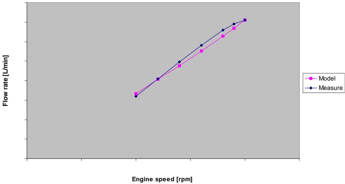
Figure 49. Flow through air compressor cooler, Test 15.
