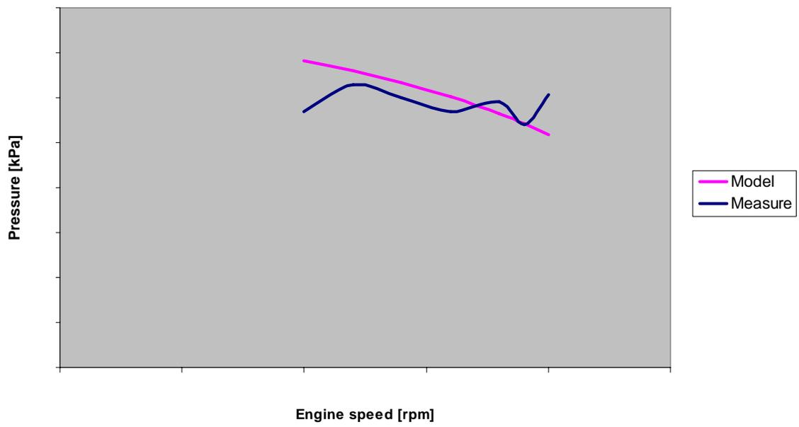
Figure 72. Pressure before coolant pump, Test 13.
