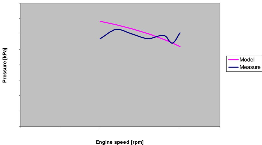
Figure 46. Pressure before coolant pump, Test 13.
