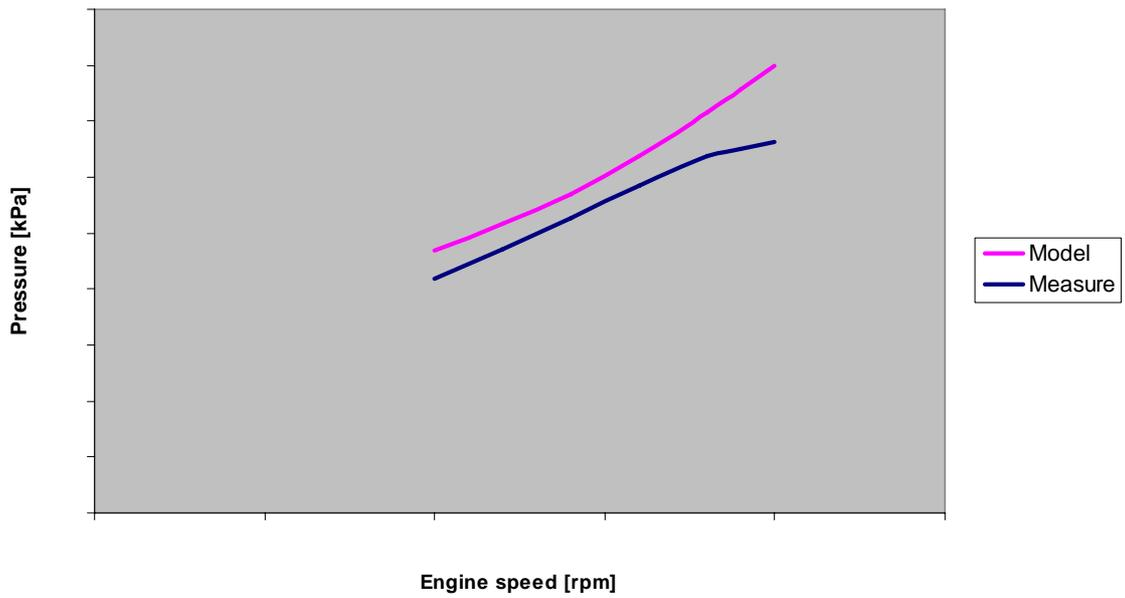
Figure 88. Pressure before transmission, Test 15.
