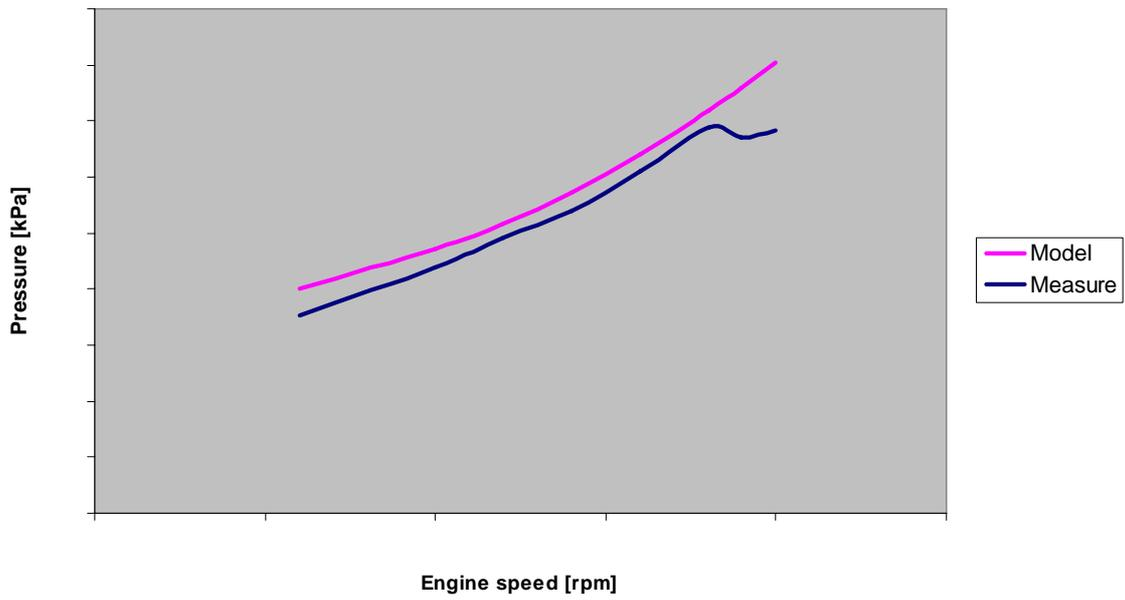
Figure 62. Pressure before transmission, Test 11.
