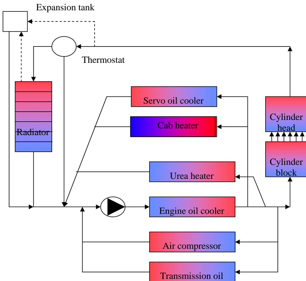
Figure 17. The coolant circuit.
