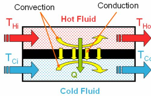
Figure 11. A general heat exchanger.
