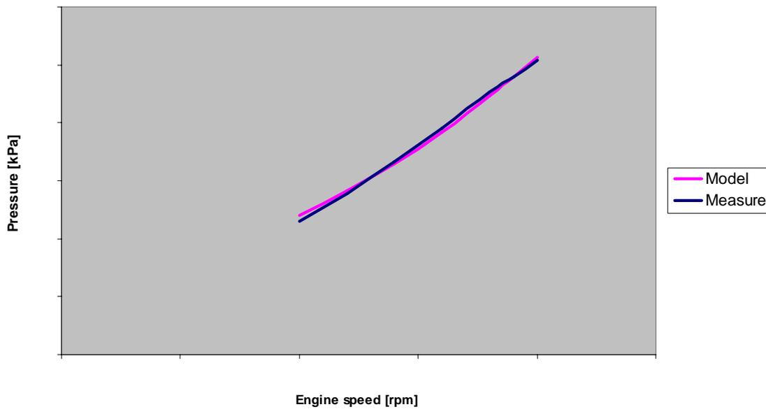
Figure 51. Pressure after coolant pump, Test 15.
