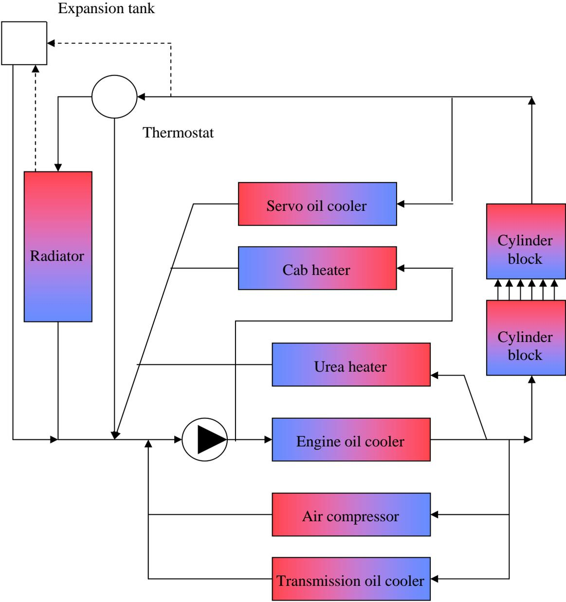
Figure 52. The modified circuit.
