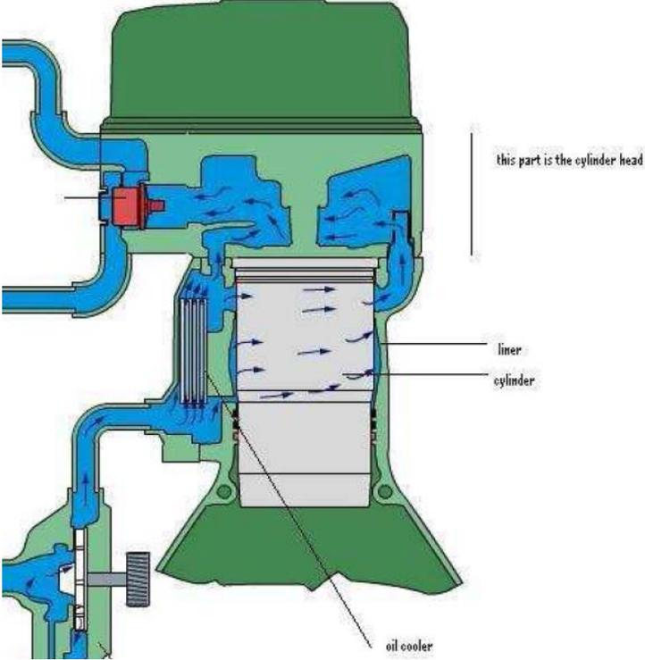
Figure 93. The flow through cylinder head and cylinder block.
