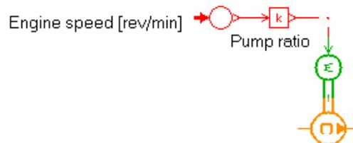
Figure 21. Coolant pump in AMESim.
