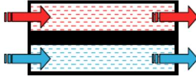
Figure 13. Parallel flow heat exchanger.
