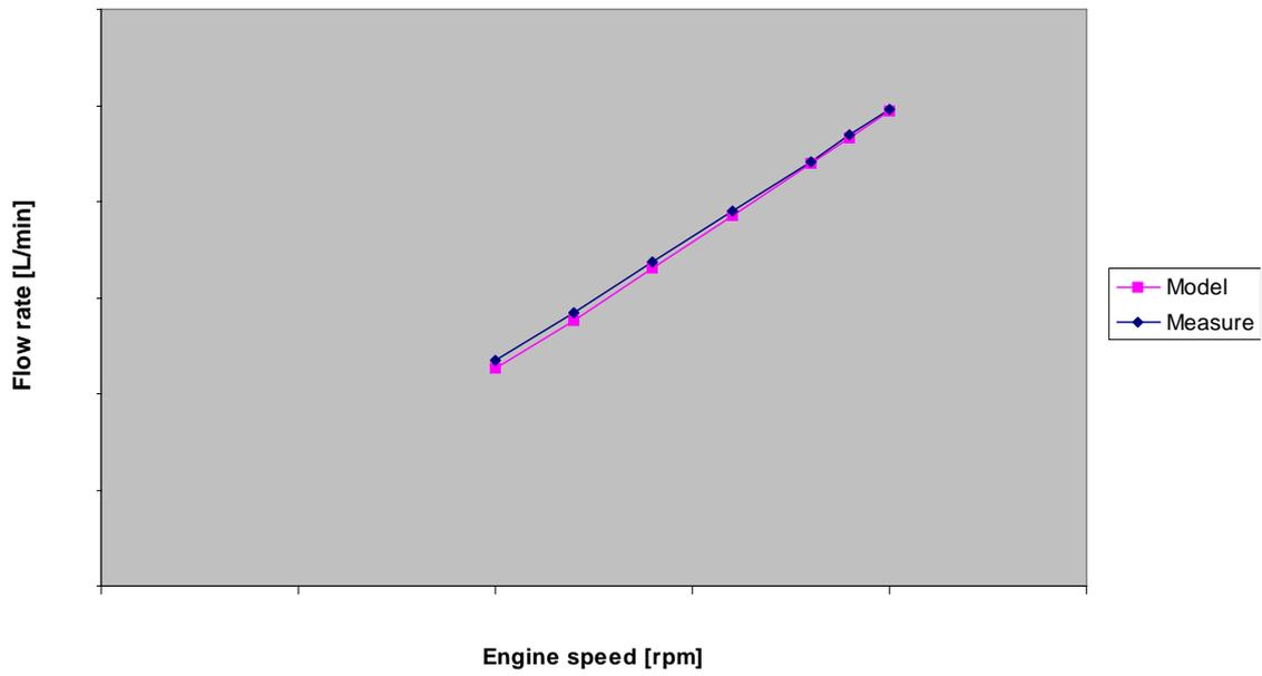
Figure 65. Flow through cab heater, Test 13.
