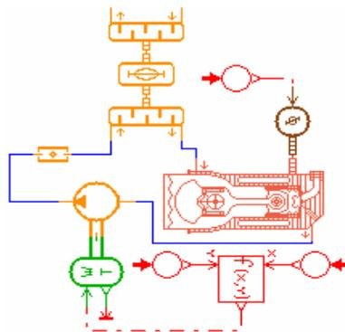
Figure 30. AMESim model of air compressor.
