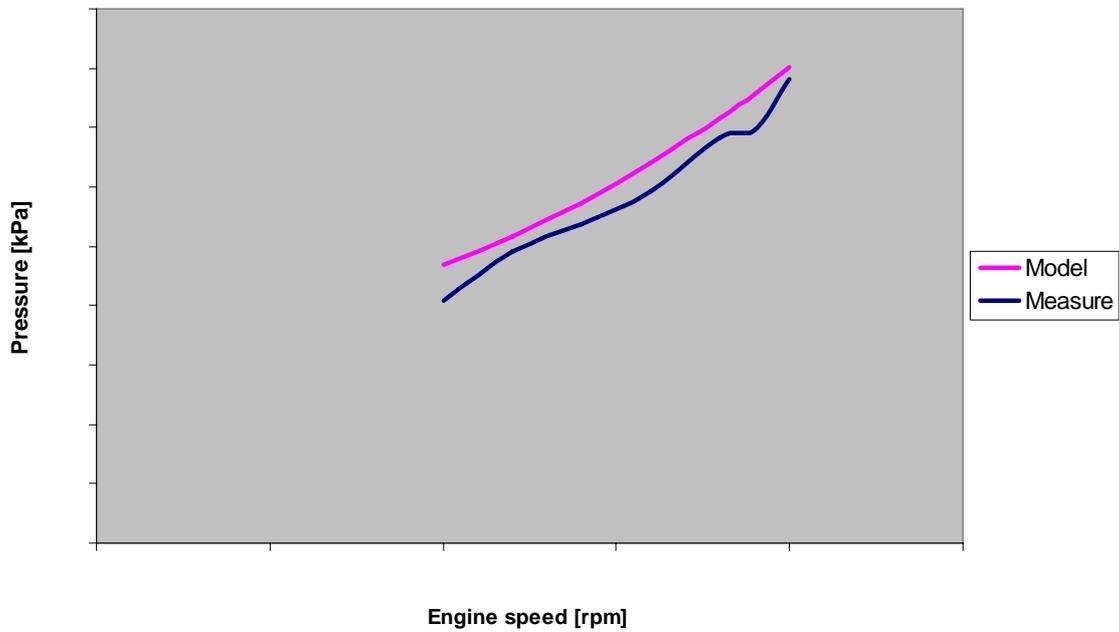
Figure 45. Pressure before transmission, Test 13.
