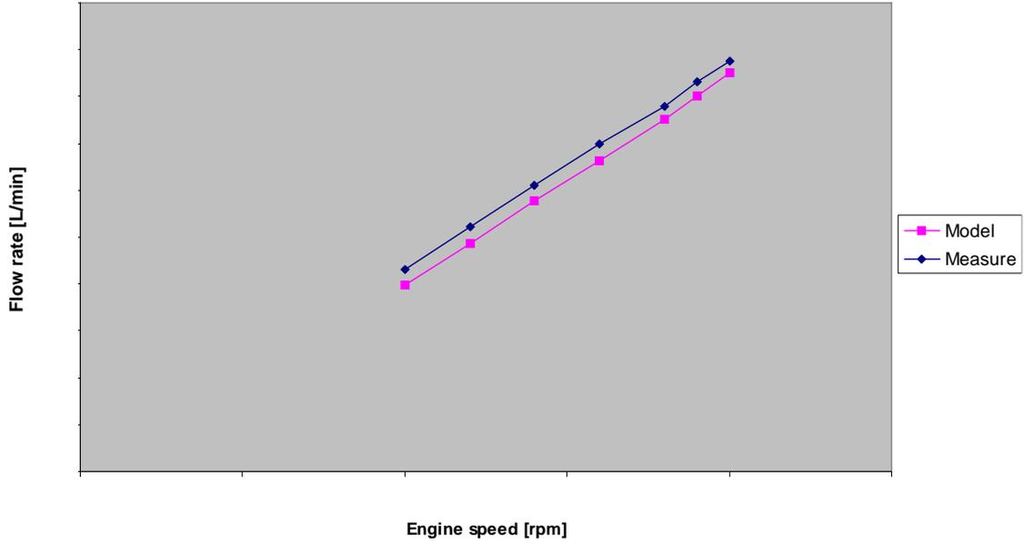
Figure 67. Flow through radiator, Test 13.
