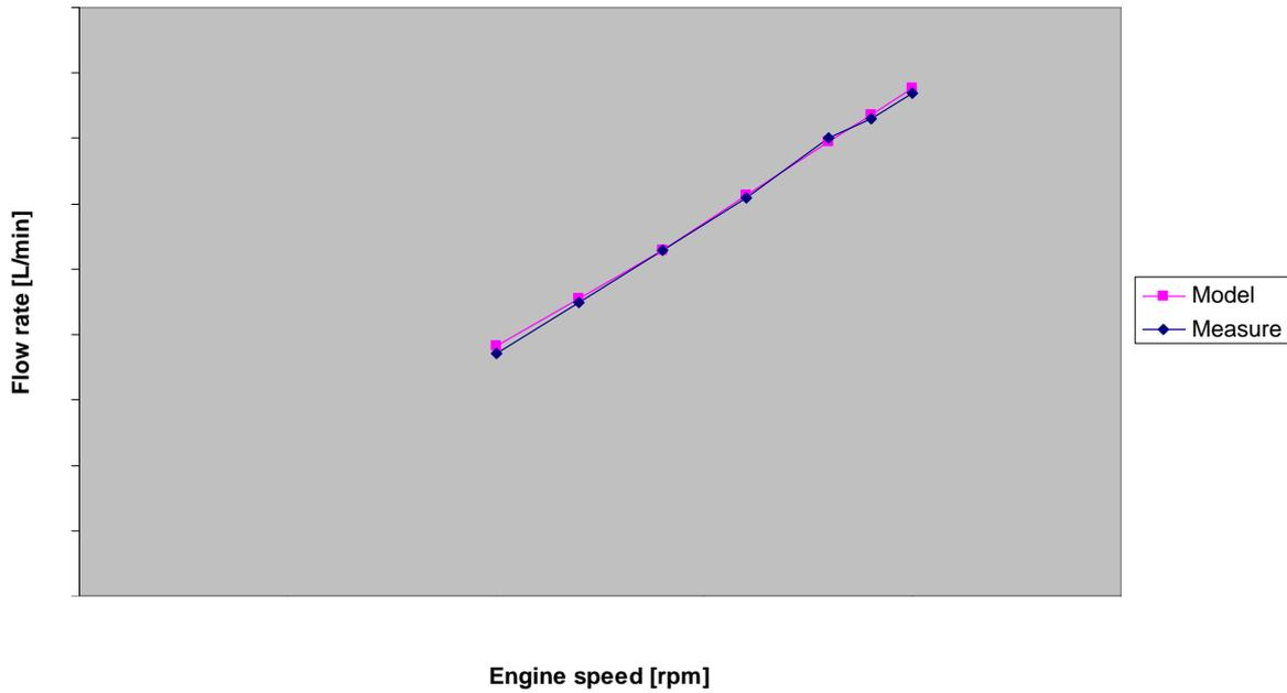
Figure 43. Flow through urea heater, Test 13.
