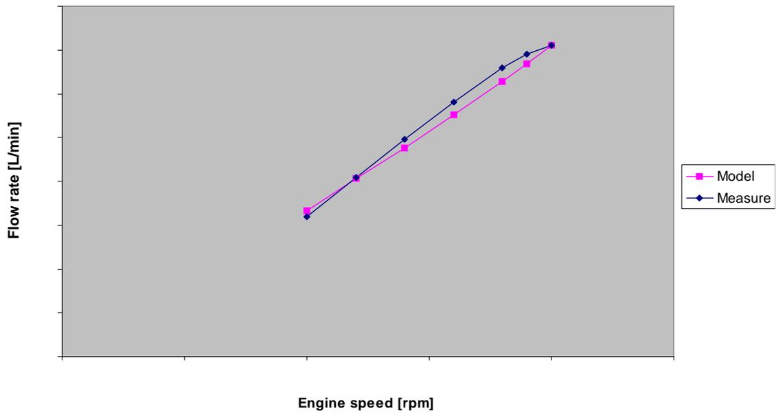
Figure 82. Flow through air compressor cooler, Test 15.
