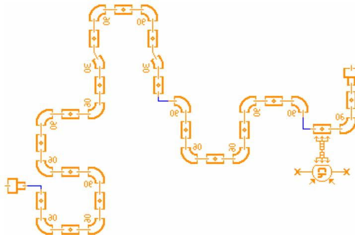
Figure 28. The AMESim model of urea heater.
