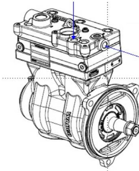
Figure 29. Two cylinders air compressor.
