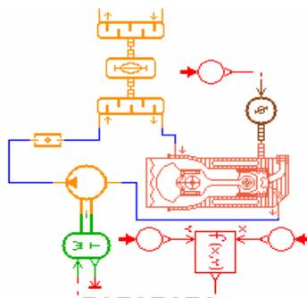
Figure 34. AMESim model of general heat exchanger.
