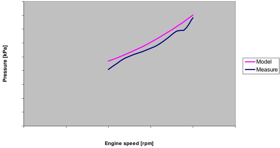
Figure 75. Pressure before transmission, Test 13.
