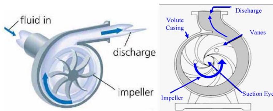
Figure 18. Centrifugal pump.
