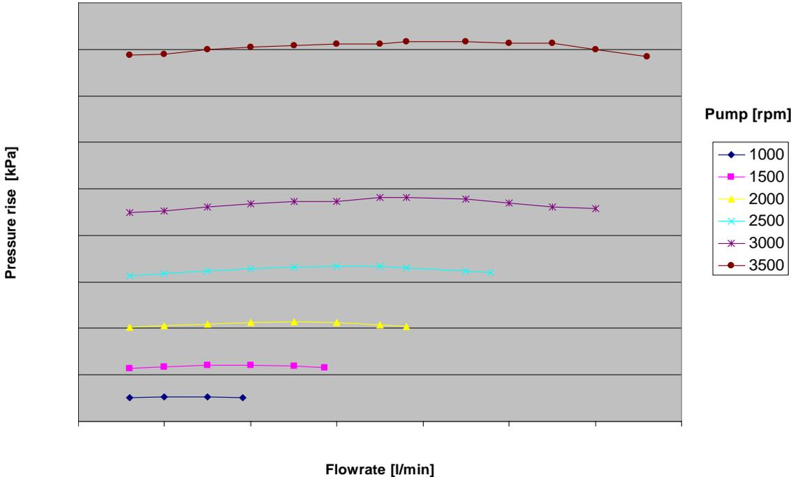
Figure 19. Coolant pump characteristic curve for a MD13 EURO5.
