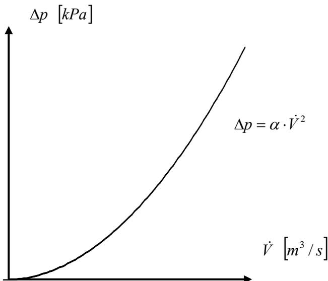
Figure 3. The system curve.
