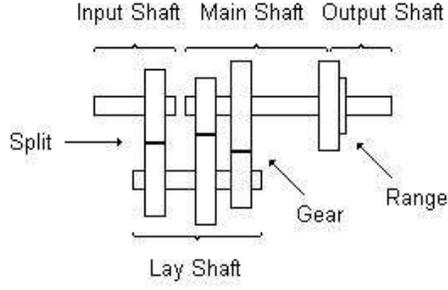
**Figure 3.3.** The gearbox in principle. A real gearbox has more cogwheels than the picture shows.
