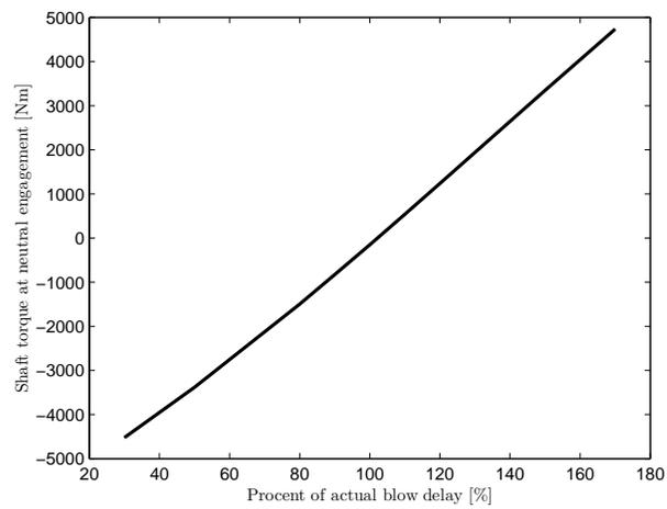
**Figure 7.14.** The shaft torque at neutral engagement with error in the blow delay.
