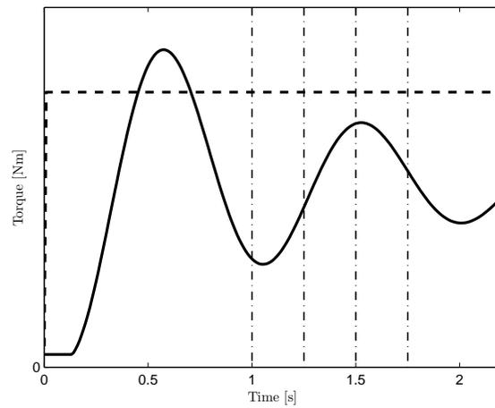
**Figure 6.2.** A step in the reference torque (dashed and scaled) results in oscillations in the shaft torque (solid). Gear shifts are commanded at different times after the step to investigate how initial conditions affect the controllers.
