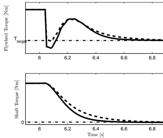
**Figure 10.4.** The difference between PD-controller (solid) and the D-controller (dashed).
