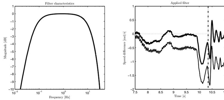
**Figure 8.2.** Left: The Butterworth bandpass filter characteristics. Right: The speed difference used as feedback signal, unfiltered (thin) and band pass filtered signal (bold).
