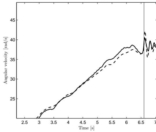
**Figure 5.5.** Simulated (dashed) and measured (solid) transmission speed during tip-in and neutral engagement on gear four. The vertical line shows when the neutral sensor indicates that neutral is engaged.
