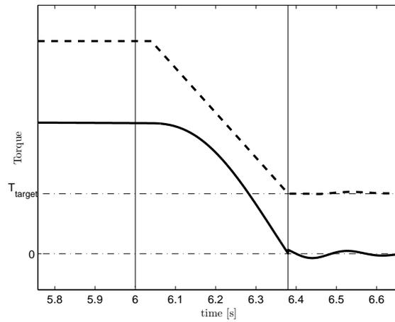
**Figure 7.2.** Flywheel torque  $T_{in}$  (dashed) and shaft torque  $T_d$  (solid) during torque control in half a period.
