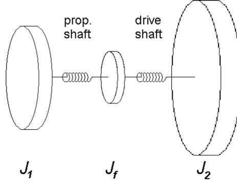
**Figure 3.5.** The three inertia model with two springs.
