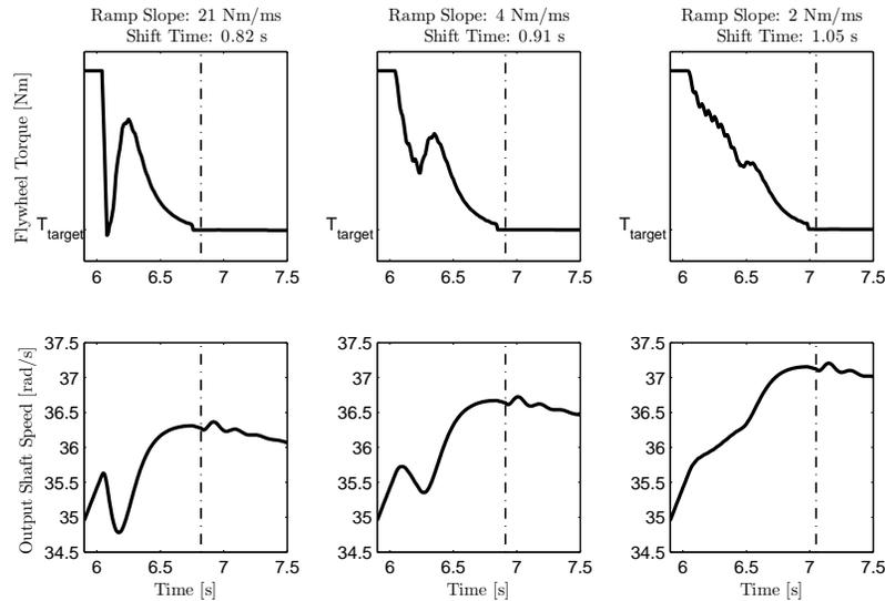
**Figure 8.7.** Three neutral engagements with a ramp plus D-controller with different slopes of the ramps. Top figures show the flywheel torque and the bottom figures show the output shaft speed. The vertical lines represents neutral engagement (dash dotted). The oscillations in the output shaft speed is about the same, but the sink is deeper the steeper the slope is.
