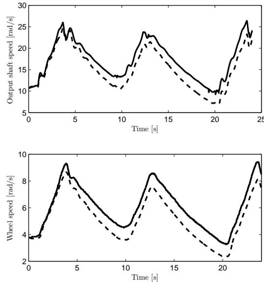
**Figure 5.2.** Top figure: Simulated (dashed) and measured (solid) transmission speed when driving without gear shift on gear two. Bottom figure: Simulated (dashed) and measured (solid) wheel speed when driving without gear shift on gear two.
