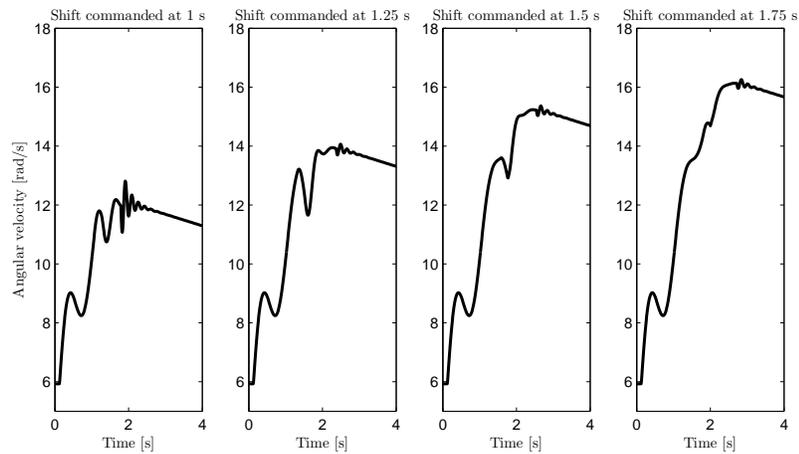
**Figure 8.9.** The transmission speed for different gear shifts with the combined controller. A gear shift was commanded at 1.0 s, 1.25 s, 1.5 s and 1.75 s after a step in the reference torque.
