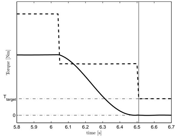
**Figure 7.17.** Flywheel torque  $T_{in}$  (dashed and scaled) and shaft torque  $T_d$  (solid) during gear shift with step controller.
