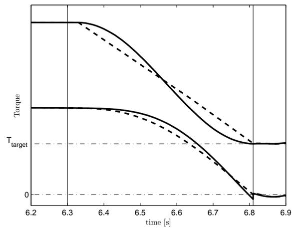
**Figure 7.11.** Comparison between the ramp controller (dashed) and the sinus controller (solid). Flywheel torque  $T_{in}$  and shaft torque  $T_d$  during torque control.
