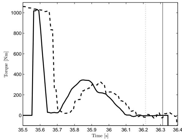
**Figure 9.5.** Flywheel torque (dashed and scaled) and reference torque (solid) when using the D-controller.
