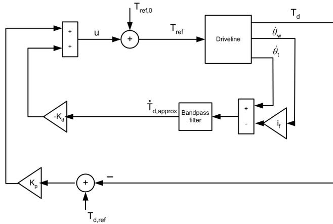
**Figure 10.2.** The structure of the PD-controller. In order to achieve a non-zero reference torque for the engine, the signal  $T_{ref,0}$  is required. A simple solution is to choose  $T_{ref,0}$  as a ramp with a reasonable slope and control the shaft torque with the other reference signal.
