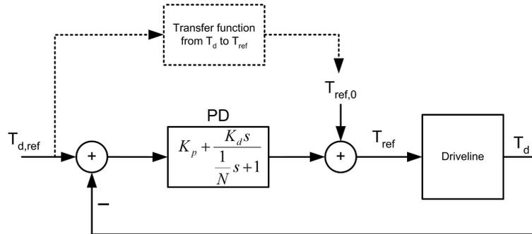
**Figure 10.1.** A regular PD-structure where the shaft torque derivative is calculated and low pass filtered in the controller. The reference for the engine torque  $T_{ref,0}$  can be calculated using feedforward, but a simple solution is to use a ramp as  $T_{ref,0}$ .
