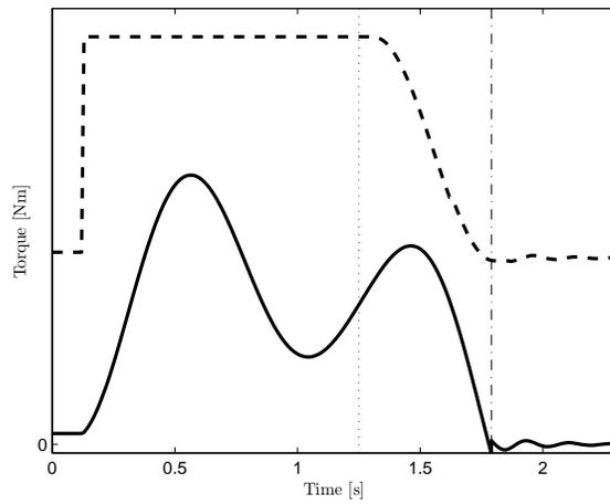
**Figure 7.13.** The shaft torque (solid) and input torque (dashed) when a gear shift is commanded after a step in the input torque. The vertical lines shows when the gear shift was commanded (dotted) and when the neutral was engaged (dash dotted).
