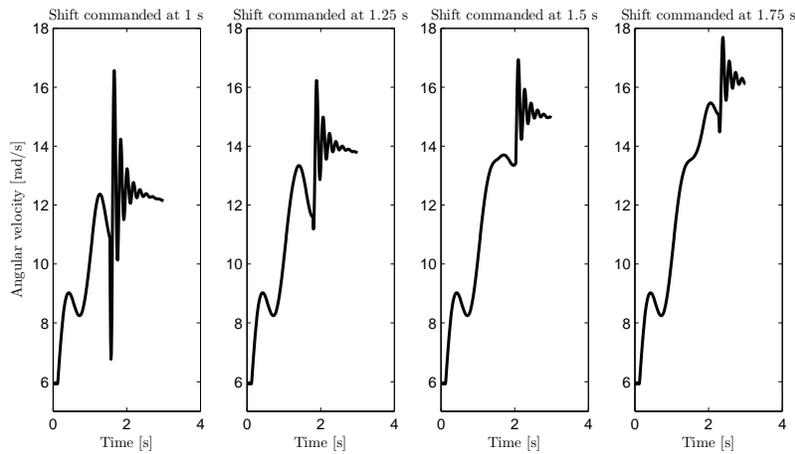
**Figure 7.12.** The transmission speed for different gear shifts. A gear shift was commanded at 1.0 s, 1.25 s, 1.5 s and 1.75 s after a step in the reference torque.
