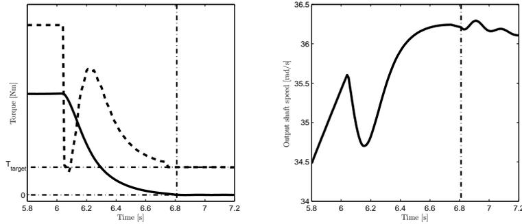
**Figure 8.4.** Left figure: Torque control with the D-controller, flywheel torque (dashed and scaled) and shaft torque (solid). Right figure: Output shaft speed during torque control with the D-controller.
