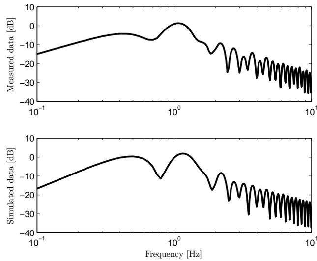
**Figure 5.6.** Upper: FFT of measured output shaft speed. Lower: FFT of corresponding simulated data.
