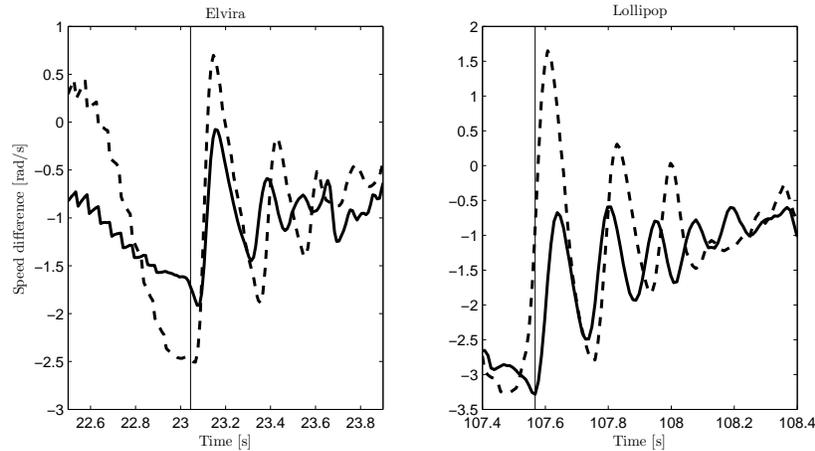
**Figure 9.1.** Speed difference after neutral engagement for entire period ramp controller (solid) and existing controller (dashed) in the trailer-truck Elvira (left) and the truck Lollipop (right). The vertical lines represent neutral engagement.
