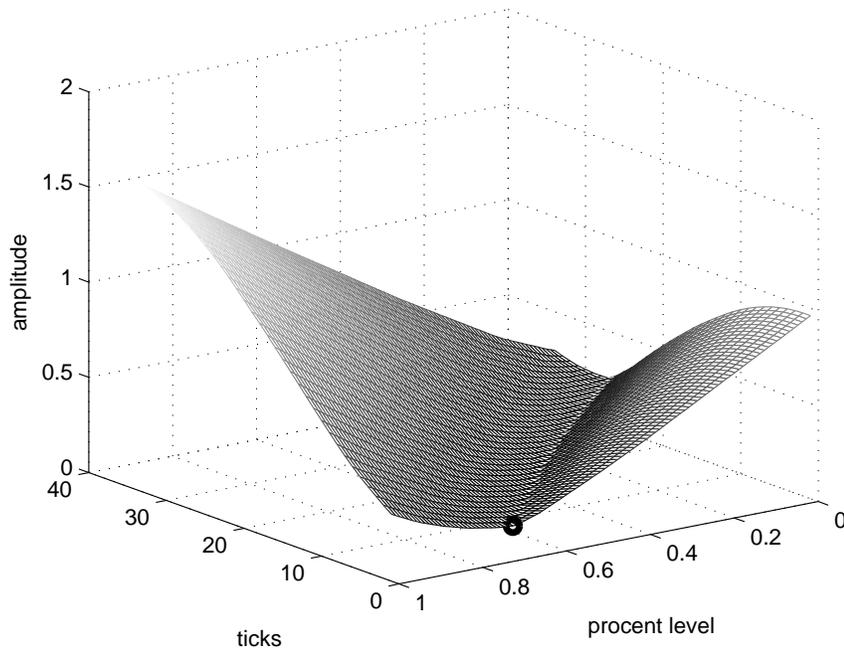
**Figure 7.9.** The amplitude of the oscillations in the output shaft speed after neutral engagement from gear four. The x- and y-axis shows where the breakpoint was placed. The smallest amplitude was measured when the breakpoint between the two ramps was placed one tick (10 ms) from the start of the control and on a level of 71% from the target torque.
