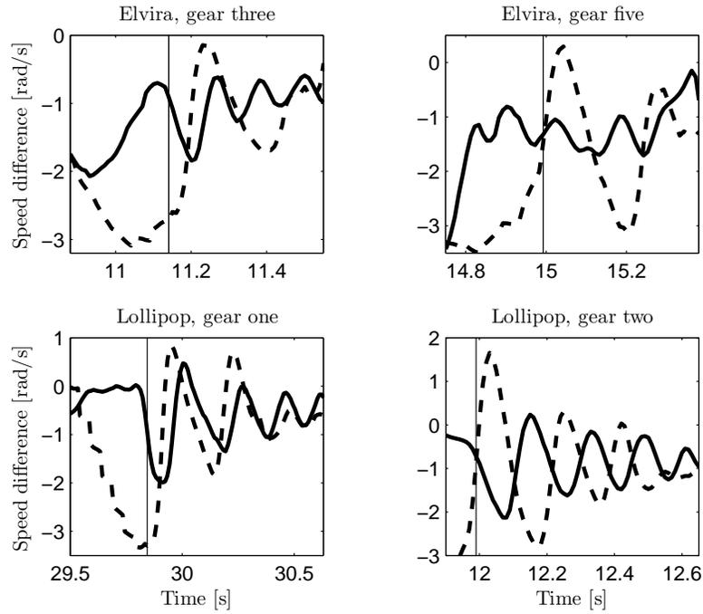
**Figure 9.4.** Speed difference after neutral engagement for the D-controller (solid) and existing controller (dashed). The vertical lines represent neutral engagement.
