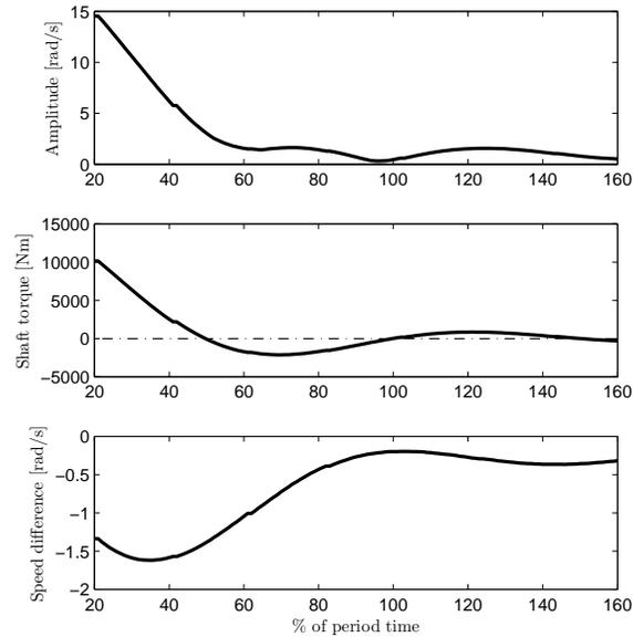
**Figure 7.4.** Amplitude of output shaft oscillations (top), shaft torque before neutral engagement (middle) and speed difference before neutral engagement (bottom) during a simulation sweep where the period is changed.
