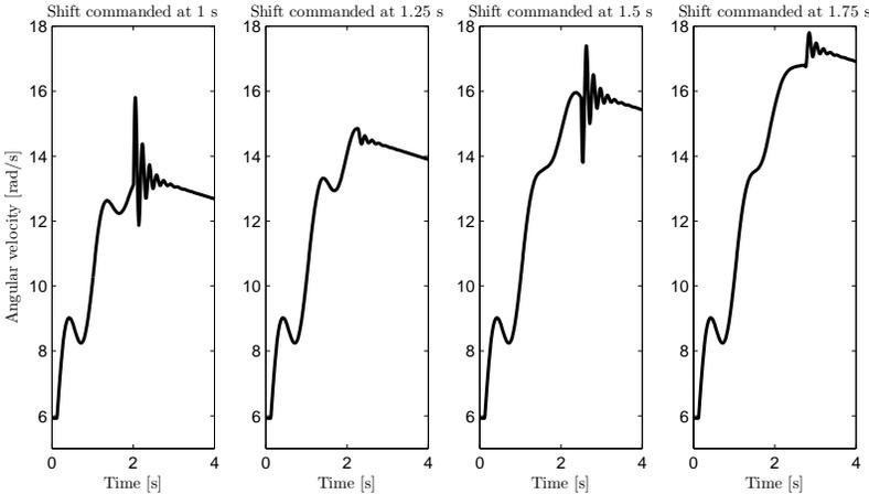
**Figure 7.5.** The transmission speed for different gear shifts with the ramp performed in an entire period. A gear shift was commanded at 1.0 s, 1.25 s, 1.5 s and 1.75 s after a step in the reference torque.
