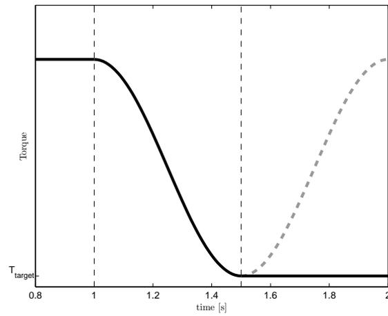
**Figure 7.10.** The reference torque  $T_{ref}$  is computed with the cosinus-function during the control time and is then set to  $T_{target}$ .
