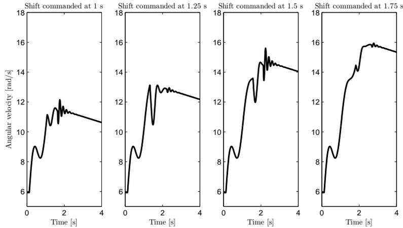
**Figure 8.6.** The transmission speed for different gear shifts with the D-controller. A gear shift was commanded at 1.0 s, 1.25 s, 1.5 s and 1.75 s after a step in the reference torque.
