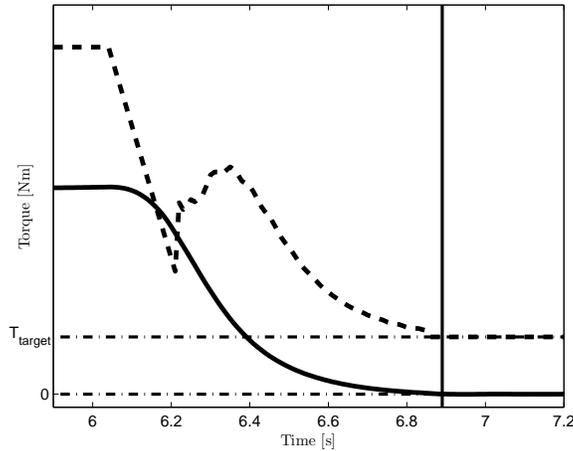
**Figure 8.8.** Torque control with the D-controller combined with a ramp with constant slope. The D-controller is activated at 25% of the ramp.
