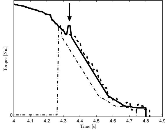
**Figure 5.1.** Measured flywheel torque (dashed), measured reference torque (dash-dotted) and the simulated flywheel torque (solid). The arrow implies where the input signal is changed from the flywheel torque to the delayed reference torque.
