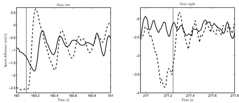
**Figure 9.7.** Speed difference after neutral engagement when making a gear shift with a ramp plus the D-controller (solid) and the existing controller (dashed) in the trailer-truck Elvira. The vertical lines represents neutral engagement.
