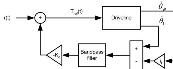
**Figure 8.3.** The driveline with a D-controller. The reference signal  $r(t)$  is used to add the target torque or combine the D-controller with an open-loop strategy.
