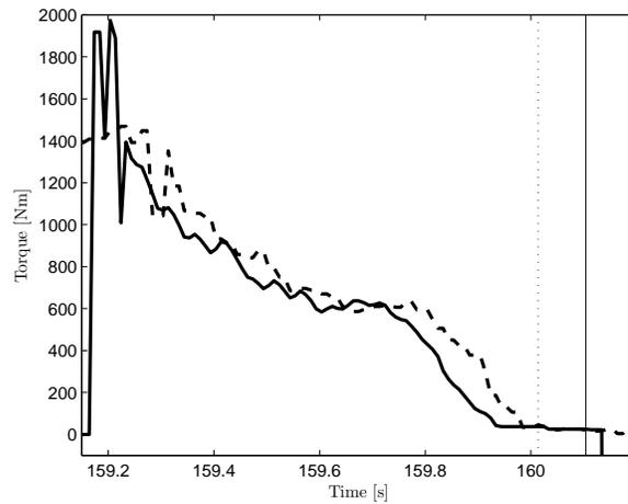
**Figure 9.6.** Flywheel torque (dashed and scaled) and reference torque (solid) when using a ramp plus the D-controller.
