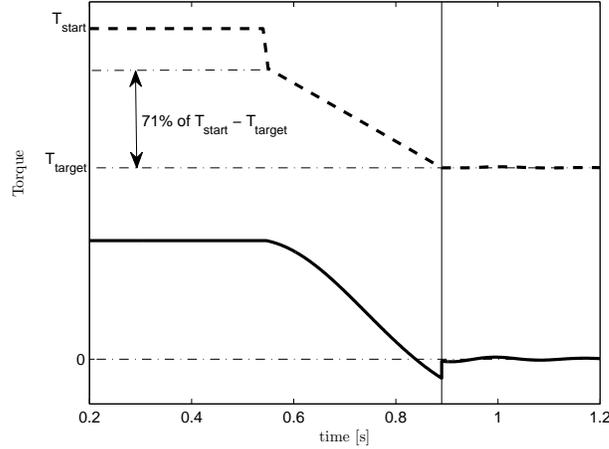
**Figure 7.8.** Flywheel torque  $T_{in}$  (dashed) and shaft torque  $T_d$  (solid) during torque control with two ramps in a total control time of half a period on the fourth gear. The discontinuity in the shaft torque at gear disengagement was discussed in Section 4.1.2
