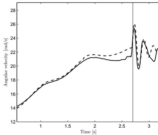
**Figure 5.4.** Simulated (dashed) and measured (solid) transmission speed during tip-in and neutral engagement on gear two. The vertical line shows when the neutral sensor indicates that neutral is engaged.
