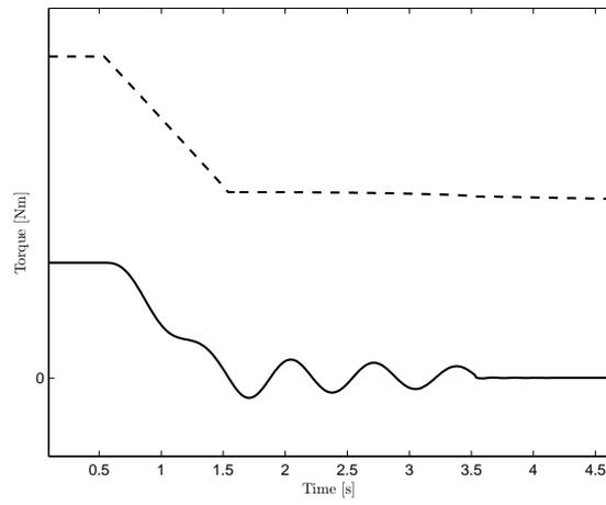
**Figure 7.1.** Reference torque  $T_{ref}$  (dashed) and shaft torque  $T_d$  (solid) during torque control.
