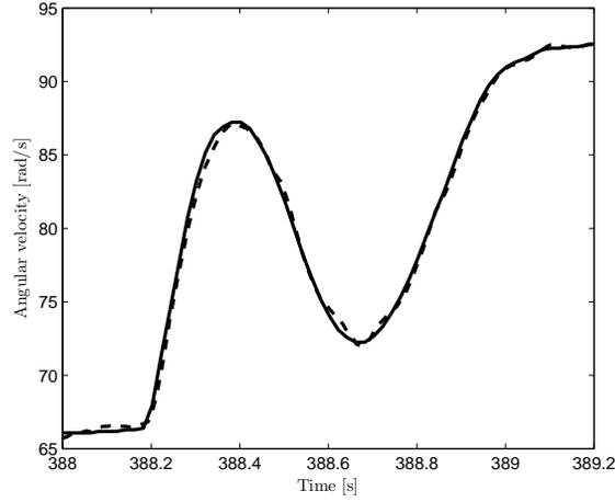
Figure 3.6. Engine speed (solid) and output shaft speed (dashed).
