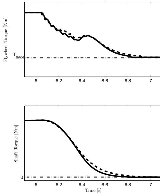
**Figure 10.5.** The difference between PD-controller (solid) and the D-controller (dashed).
