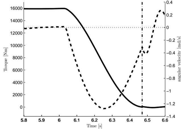
**Figure 8.1.** The shaft torque (solid) and the speed difference (dashed),  $\dot{\theta}_t - \dot{\theta}_{wi_f}$ , during simulated torque control with the step controller. The speed difference is a good approximation of the shaft torque.
