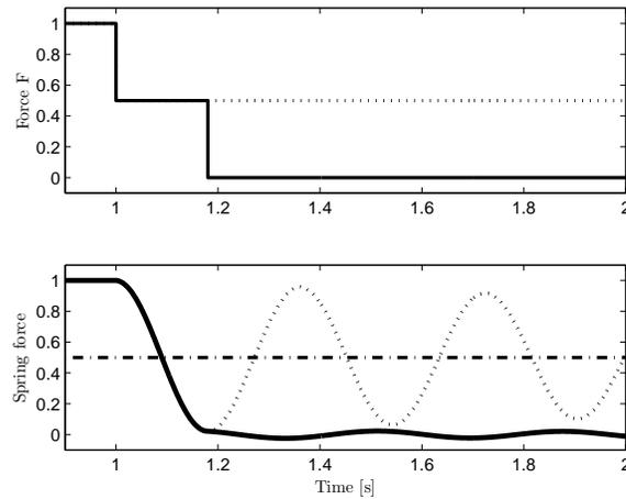
**Figure 7.16.** Change of load on a damped spring. Top: controlling force. Bottom: Spring force.
