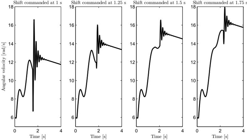
**Figure 7.6.** The transmission speed for different gear shifts with the ramp performed in half a period. A gear shift was commanded at 1.0 s, 1.25 s, 1.5 s and 1.75 s after a step in the reference torque.
