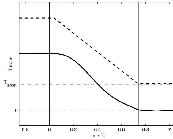
**Figure 7.3.** Flywheel torque  $T_{in}$  (dashed) and shaft torque  $T_d$  (solid) during torque control in one period.
