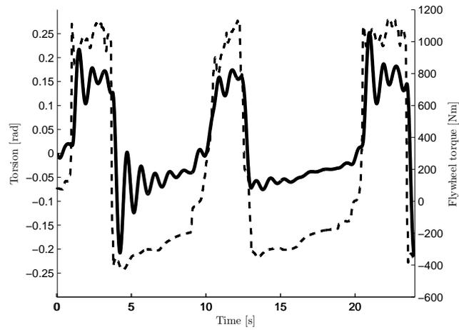
**Figure 5.3.** Simulated torsion (solid) and flywheel torque (dashed) when driving without gear shift on gear two.
