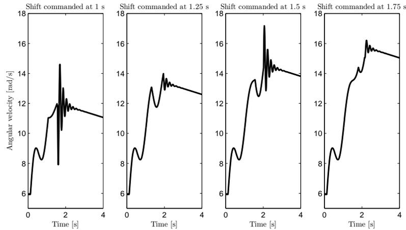
**Figure 7.19.** The transmission speed for different gear shifts. A gear shift was commanded at 1.0 s, 1.25 s, 1.5 s and 1.75 s after a step in the reference torque.
