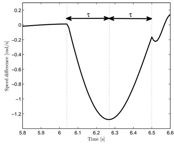
**Figure 7.18.** The speed difference,  $\dot{\theta}_t - \dot{\theta}_w i_f$ , during a gear shift using the step controller.
