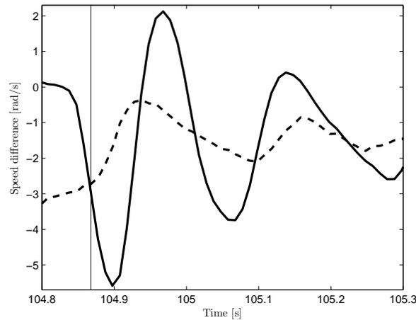
**Figure 9.3.** Speed difference after neutral engagement for step controller (solid) and existing controller (dashed) in the trailer-truck Elvira. The total control time from gear shift command to neutral engagement was 0.57 s for the step controller and 0.54 s for the existing controller. The vertical line represents neutral engagement.
