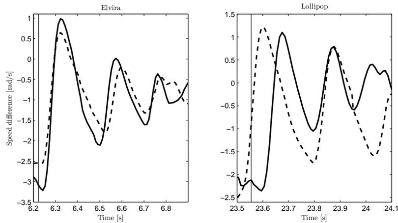
**Figure 9.2.** Speed difference after neutral engagement for half period ramp controller (solid) and existing controller (dashed) in the trailer-truck Elvira (left) and the truck Lollipop (right). The vertical lines represent neutral engagement.
