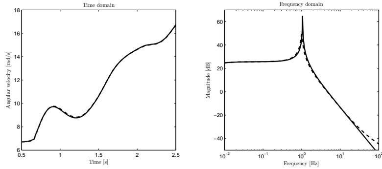
**Figure 3.7.** Left: Simulated output shaft speed during a tip-in on gear 2 with optimized parameters. Right: Amplitude spectrum of transfer function from  $T_{in}$  to shaft torque for gear 2. Two inertia model (solid) and three inertia model (dashed).
