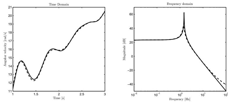
**Figure 3.8.** Left: Simulated output shaft speed during a tip-in on gear 4 with optimized parameters. Right: Amplitude spectrum of transfer function from  $T_{in}$  to shaft torque for gear 4. Two inertia model (solid) and three inertia model (dashed).
