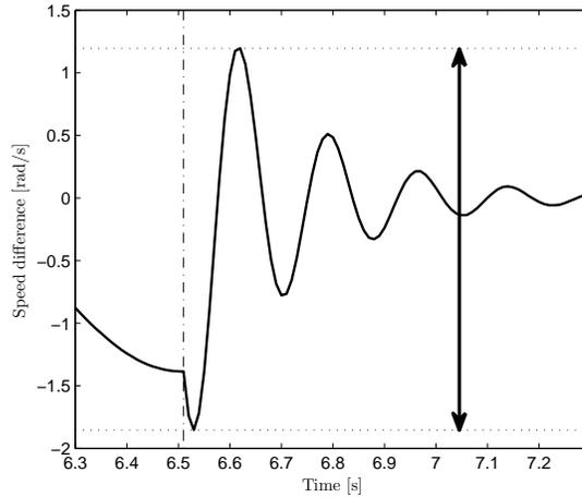
**Figure 6.1.** How the amplitude is calculated to evaluate shift quality.  $\dot{\theta}_t i_f - \dot{\theta}_w$  (solid) and time when neutral is engaged (dash-dotted).
