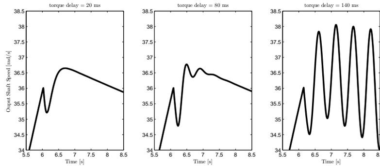
**Figure 8.5.** The transmission speed for different gear shifts with the D-controller. The torque delay was varied and the neutral was not engaged.
