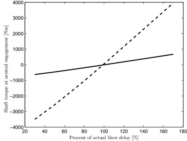
**Figure 7.7.** The shaft torque at neutral engagement for entire period ramp (solid) and half period ramp (dashed) with error in the blow delay.
