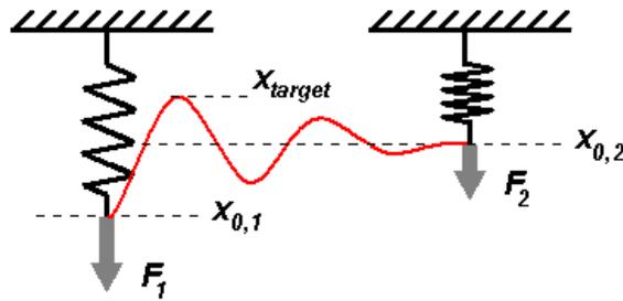
Figure 7.15. Change of load on a damped spring.
