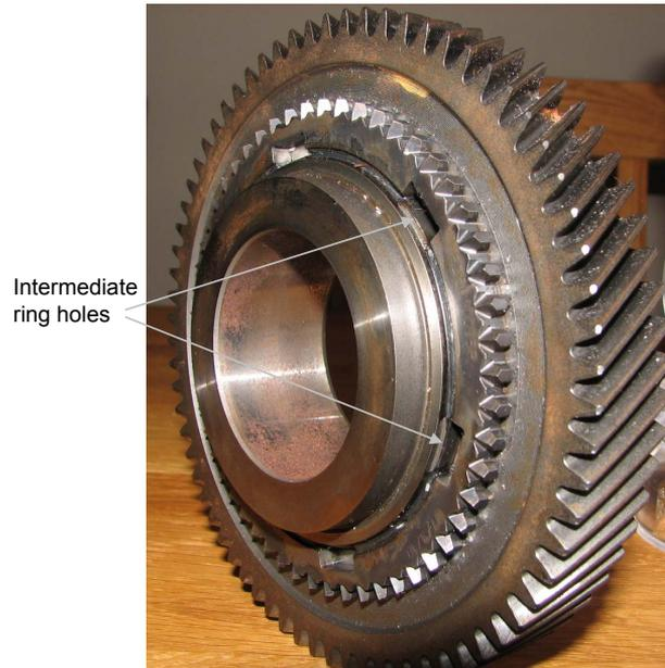
**Figure 2.6.** A gear wheel. Gear wheels are placed at the ends of the parts in figure 2.5. The intermediate ring hooks in figure 2.5 are hooked into the holes marked in this figure.
