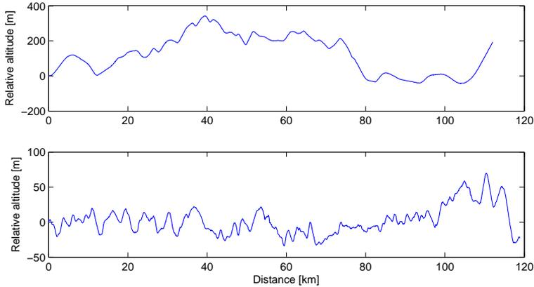
**Figure 2.2.** Road profile of Koblenz-Trier (upper) and Södertälje-Norrköping (lower) routes
