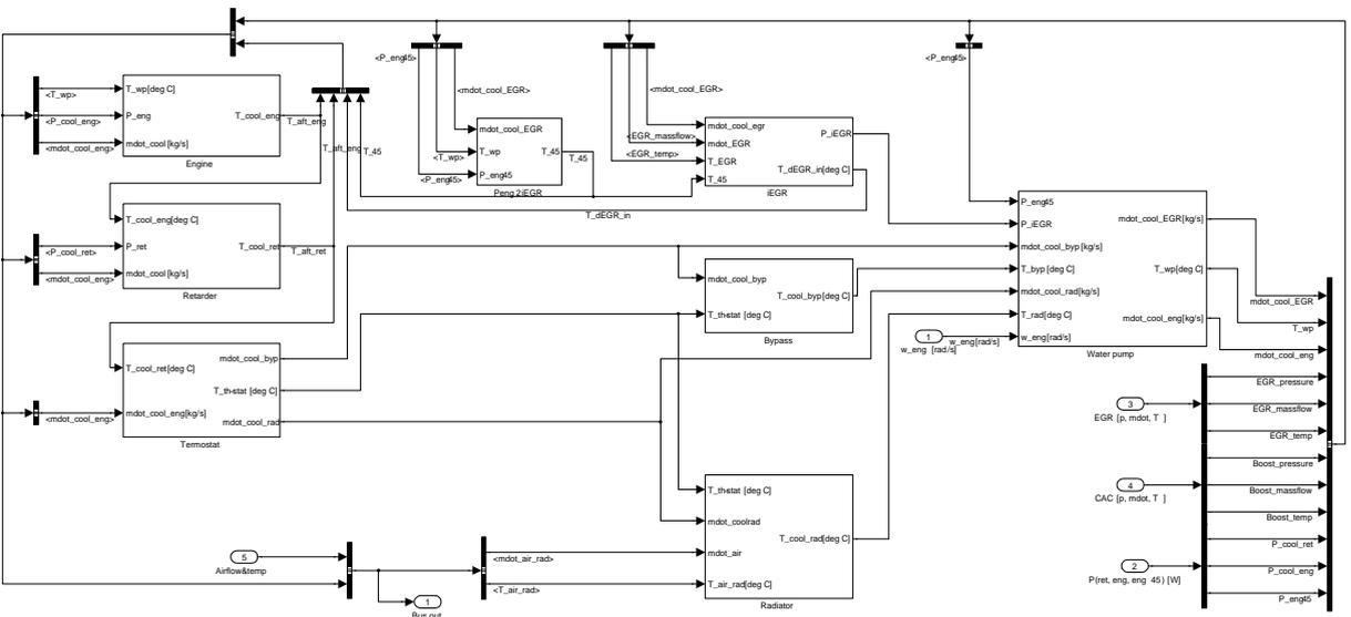
Figure 2.5. The cooling system model implemented in SIMULINK
