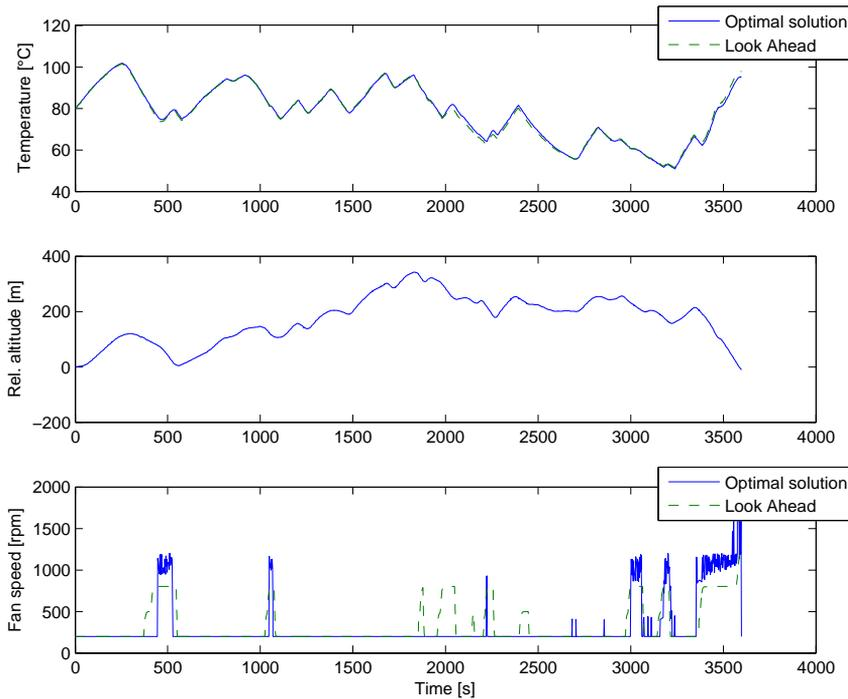
**Figure 3.11.** The optimal solution is presented and compared to the Look Ahead ditto during a one hour drive at the Koblenz-Trier route, with an ambient temperature of 30 °C. The noise is an effect of chosen calculation technique.
