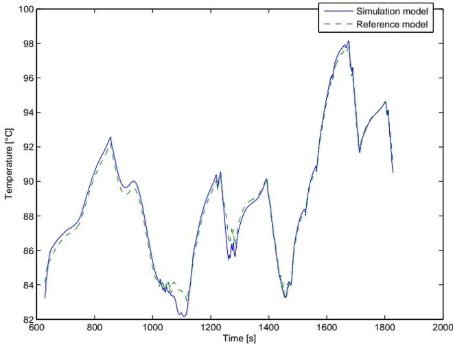
**Figure 2.8.** Cooling system model validation. Data are recorded from simulations with the cooling system model used at Scania today, and compared to the result of a simulation with the cooling system model presented in this paper. The figure presents a comparison of coolant temperatures and the accuracy is as seen quite good.
