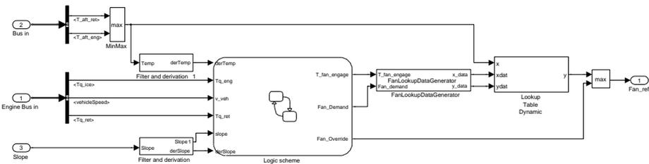
**Figure 3.2.** Top level of the Look Down controller implementation
