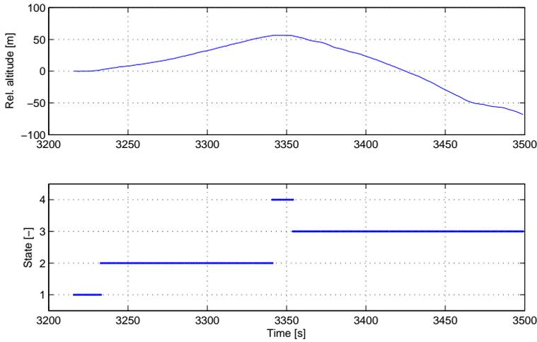
**Figure 3.4.** Example of how road segments are divided into one of four different states: 1 = flat road, 2 = uphill, 3 = downhill and 4 = crest
