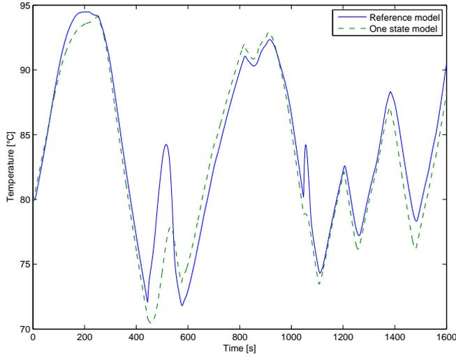
**Figure 2.9.** Validation of one state cooling model. As seen, the main dynamic is captured but the accuracy is not very good, which could be expected when using such a simplified model.
