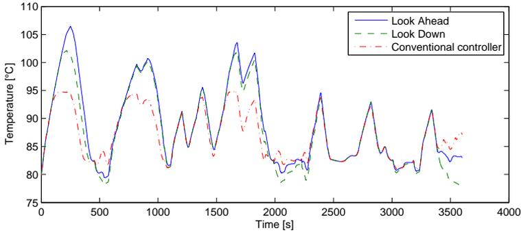
**Figure 3.8.** Engine coolant temperatures during a simulated drive at the Koblenz-Trier route, with an ambient temperature of 30 °C
