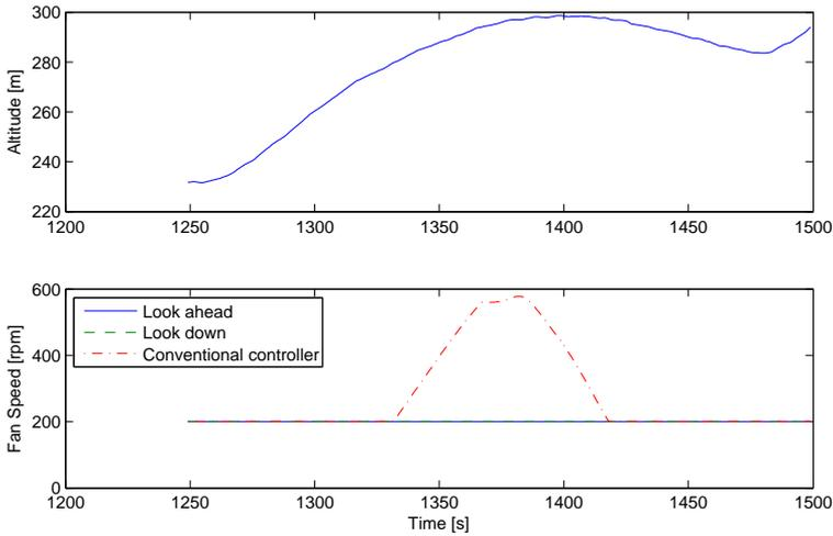
**Figure 3.7.** The figure shows an example of how a conventional fan controller engages the fan before a crest. Both the improved controllers have detected the crest and prohibit fan engagement. Note that it is only the conventional controller that engages the fan.
