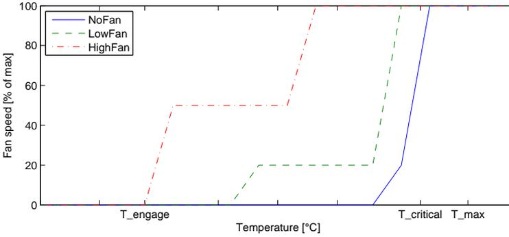
**Figure 3.3.** Fan speed map for the Look Down and Look Ahead fan controllers. The three curves correspond to the three fan engagement probability levels, and the values are given as percentage of maximum fan speed. The horizontal axle is dynamic and the values depend on  $T_{engage}$ .  $T_{critical}$  is however constant.
