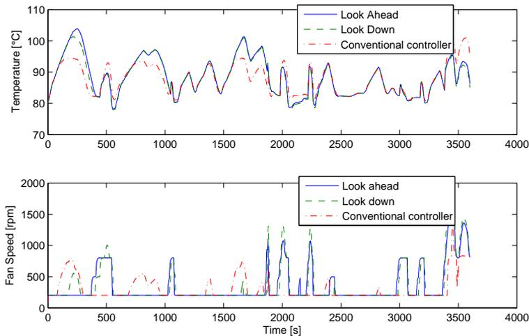
**Figure 3.9.** Coolant temperature after the retarder, and fan usage for both the conventional controller and the improved controllers. Data is collected from a simulation at the Koblenz-Trier route. See Table 3.2 for the key values associated to this simulation.
