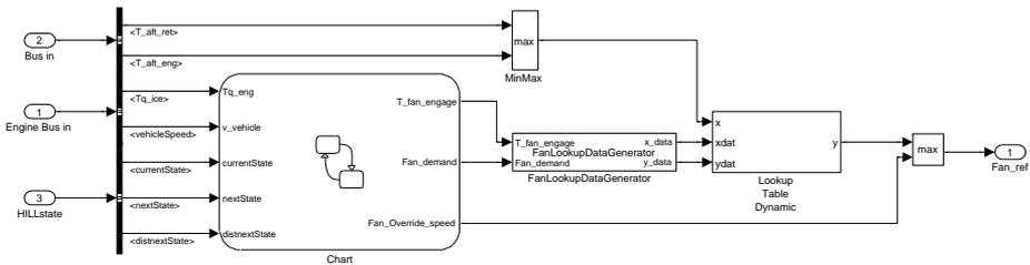
**Figure 3.6.** Top level of the Look Ahead fan controller implementation
