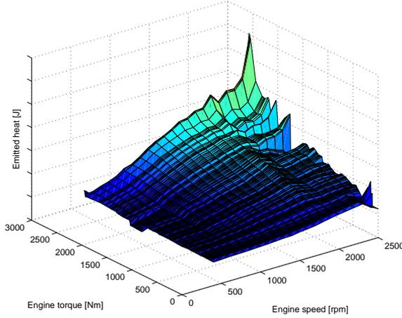
**Figure 2.6.** Heat power transfer map from engine to coolant
