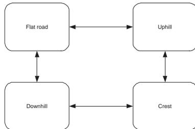
**Figure 3.5.** Top level of the stateflow implementation. The four states represent *downhill slopes, flat roads, uphill slopes and crests*. Only one state is active at a given time, and the arrows show in what direction a change of states is possible.
