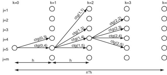
**Figure 2.10.** Sketch showing the principle layout of the optimization problem.  $ctg(k, j)$  represent the *cost* that corresponds to a change from current state to state  $j$  during time step  $k$  to  $k + 1$ . It is calculated as the cost for the step itself plus the *cheapest* path from  $k + 1$ , see Equation (2.30).
