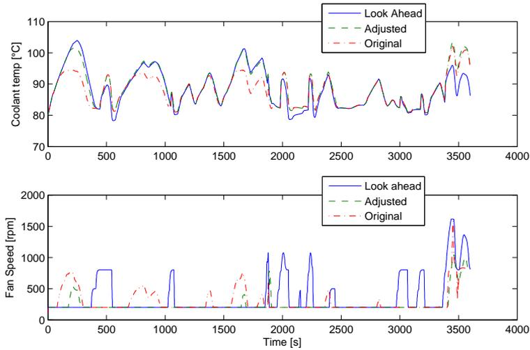
**Figure 3.10.** Coolant temperature after the retarder and fan usage for two variants of the conventional controller, one with an adjusted temperature map, and for the Look Ahead fan controller. Data is collected from a simulation at the Koblenz-Trier route. See Table 3.4 for the key values associated to this simulation.
