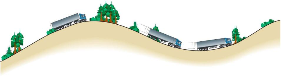
**Figure 1.1.** Example of a road where Look Ahead information could reduce energy-, and thereby fuel consumption if applied on cruise- or fan control e.g.
