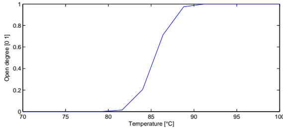
**Figure 2.7.** Part of coolant that is guided through the radiator as function of coolant temperature
